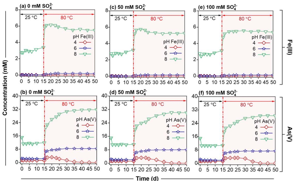
Fig. 2 Temporal changes in the concentrations of aqueous Fe(III) and As(V) during HFA transformation at  $\text{SO}_4^{2-}$  concentrations of (a and b) 0 mM, (c and d) 50 mM, and (e and f) 100 mM as a function of pH (4, 6, and 8) under the 25 °C condition for 15 d followed by aging at 80 °C (up to day 50).
