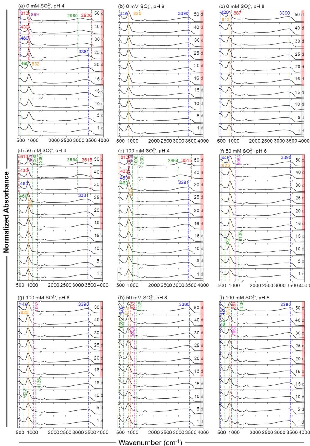
Fig. 4 FTIR spectra recorded upon the addition of different concentrations of  $\text{SO}_4^{2-}$  (a)–(c) 0 mM, (d), (f) and (h) 50 mM, and (e), (g) and (i) 100 mM to the HFA system at different pH conditions and over different stabilization times.
