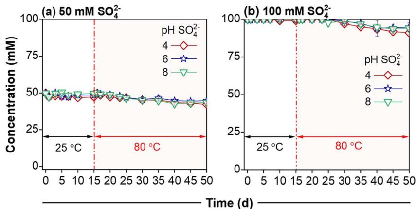
Fig. 1 Temporal changes in the aqueous  $\text{SO}_4^{2-}$  concentration during HFA transformation. These changes were investigated using various concentrations of  $\text{SO}_4^{2-}$  ((a) 50 mM and (b) 100 mM) at pH 4, 6, and 8.
