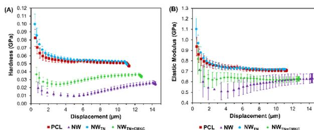
**Fig. 5** (A) Indentation hardness (GPa) vs. displacement ( $\mu\text{m}$ ) and (B) elastic modulus (GPa) vs. displacement ( $\mu\text{m}$ ) for different surfaces.
