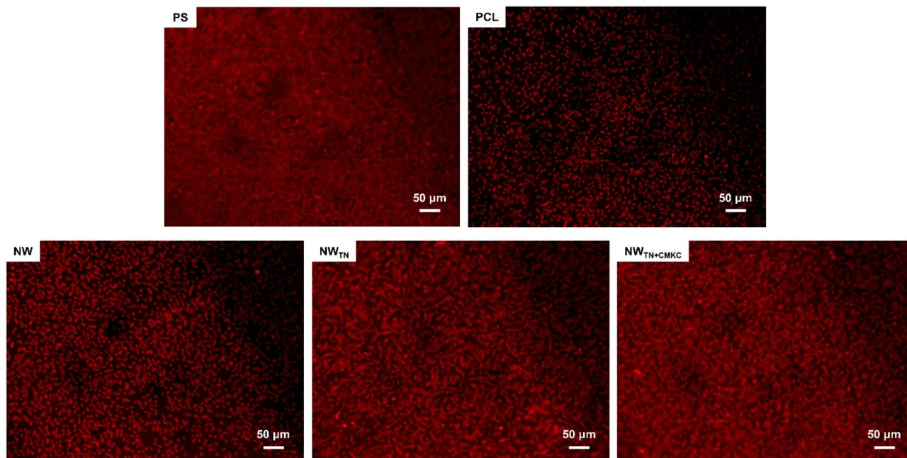
Fig. 10 Representative fluorescence microscopic images of adhered erythrocyte cells on surfaces after 6 hours of incubation.
