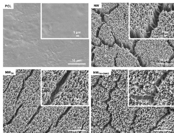
Fig. 1 Representative SEM images of different surfaces at low (2500 $\times$ ) and high magnification (insert, 7500 $\times$ ). Scale bars of low and high magnification images indicate 10  $\mu\text{m}$  and 1  $\mu\text{m}$ , respectively.
