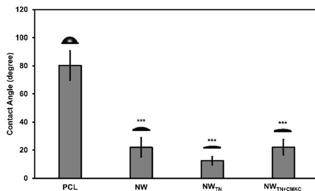
Fig. 2 Static water contact angle of different surfaces. Images of water droplet on the surfaces are also shown in the plot. Statistical significances ( $p$ -value) were represented as \*\*\* for  $p < 0.001$  when compared to PCL control.
