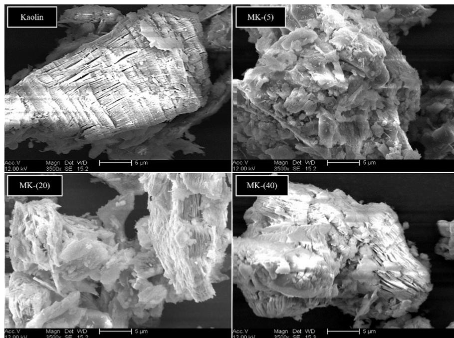
Fig. 2 SEM images of kaolin (top left) and metakaolin samples MK-(5) (top right), MK-(20) (bottom left) and MK-(40) (bottom right), achieved by TGA measurements using  $\beta = 5, 20$  and  $40 \text{ K min}^{-1}$ .
