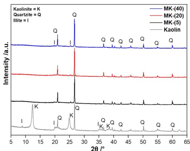
Fig. 1 XRD patterns of cameroonian kaolin and derived metakaolin samples MK-(5), MK-(20) and MK-(40), achieved by TGA measurements using  $\beta = 5, 20$  and  $40$  K min<sup>-1</sup>. The kaolin pattern shows the presence of kaolinite (K), illite (I), quartz (Q) and an amorphous phase. The measurements were performed using a PANalytical Empyrean diffractometer with Cu  $K_{\alpha 1+\alpha 2}$  radiation.
