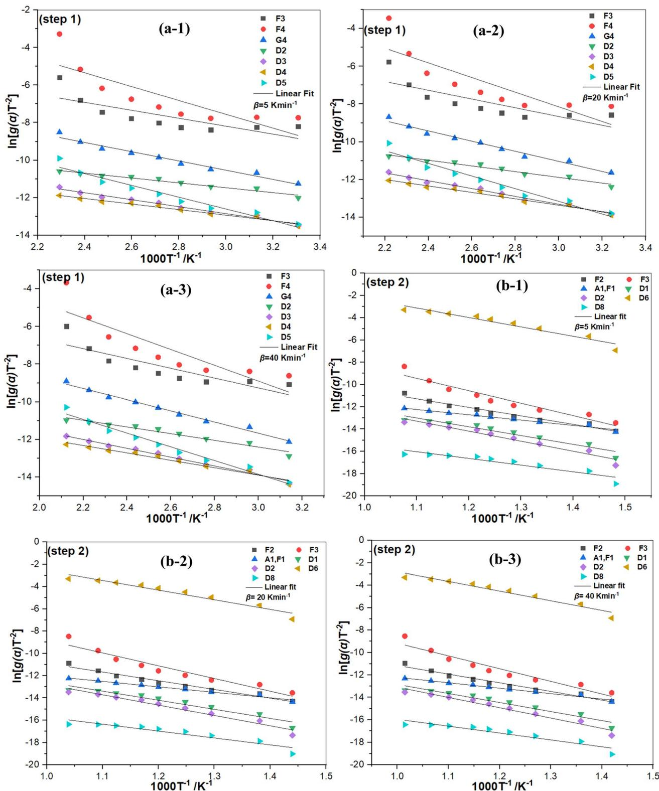
Fig. 8 Plots following the Coats-Redfern model to determine the thermokinetics of the kaolin conversion to metakaolin for step 1 (a) and step 2 (b) at heating rate of 5 K min<sup>-1</sup> (a-1 and b-1), 20 K min<sup>-1</sup> (a-2 and b-2) and 40 K min<sup>-1</sup> (a-3 and b-3).
