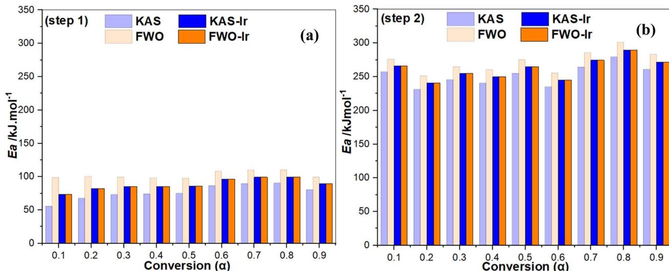
Fig. 6  $E_a$  versus degree of conversion  $\alpha$  for dehydration (step 1) (a) and dehydroxylation (step 2) (b) during the cameroonian kaolin conversion, calculated following the KAS and the FWO method. KAS-Ir and FWO-Ir describe the values derived from the iterative procedure.
