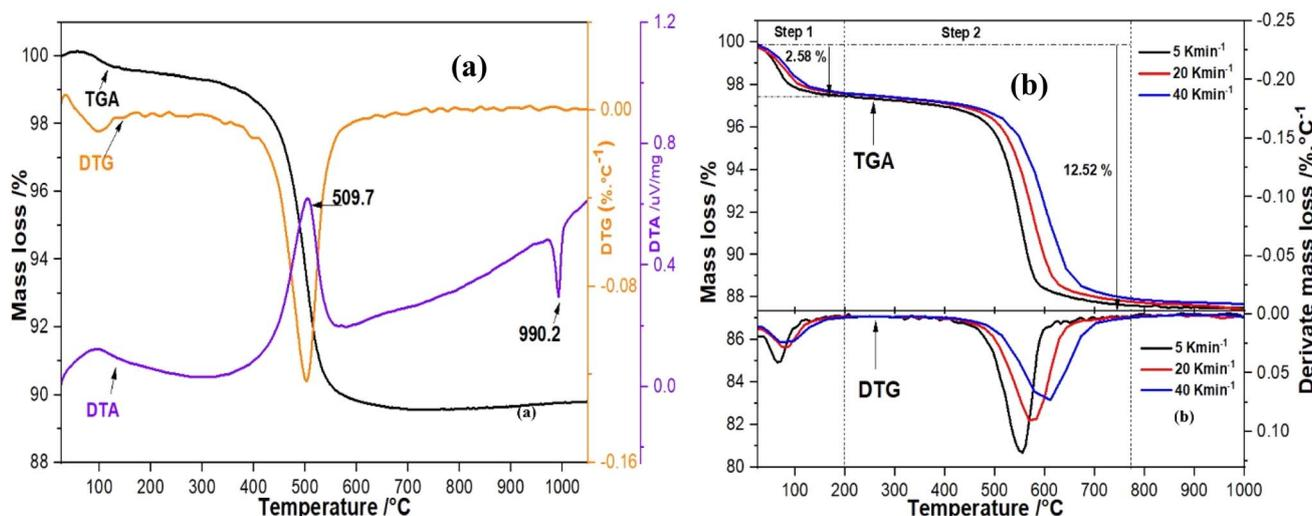
Fig. 4 (a) TGA/DTG/DTA data of cameroonian kaolin collected using an STA 449C Jupiter (Netzsch, Selb, Germany) with  $5 \text{ K min}^{-1}$ ; (b) TGA/DTG data of cameroonian kaolin collected using a TGA-701 (LECO, St. Joseph, USA) with  $\beta = 5, 20$  and  $40 \text{ K min}^{-1}$ .
