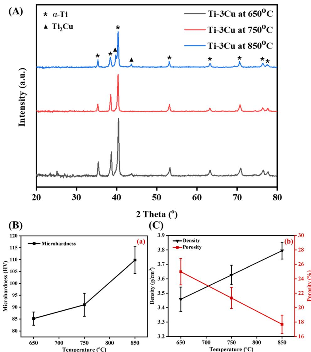
Fig. 2 (A) XRD patterns, (B) microhardness, and (C) density and porosity of Ti-3Cu substrates sintered at 650 °C, 750 °C, and 850 °C.
