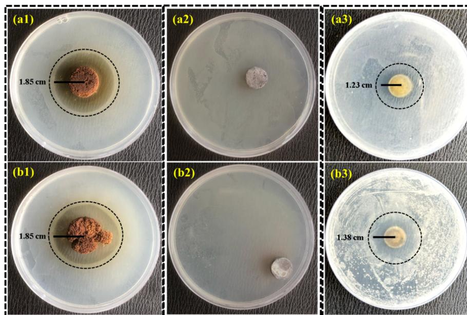
Fig. 6 Antibacterial activity of clove extract, Ti-3Cu substrate, and M-starch/MBGNs/clove extract-coated Ti-3Cu substrate against (a1–a3) *E. coli* and (b1–b3) *S. aureus*, determined through disc diffusion assay.
