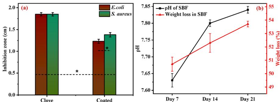
Fig. 7 Statistical analysis of the antibacterial activity of clove and the composite coated sample (a) showed a significant difference (\*) and the difference was significant in *E. coli* and *S. aureus* results of the coated sample. (b) Weight loss of the coating in SBF and changes in the alkalinity of SBF on day 7, 14, and 21.
