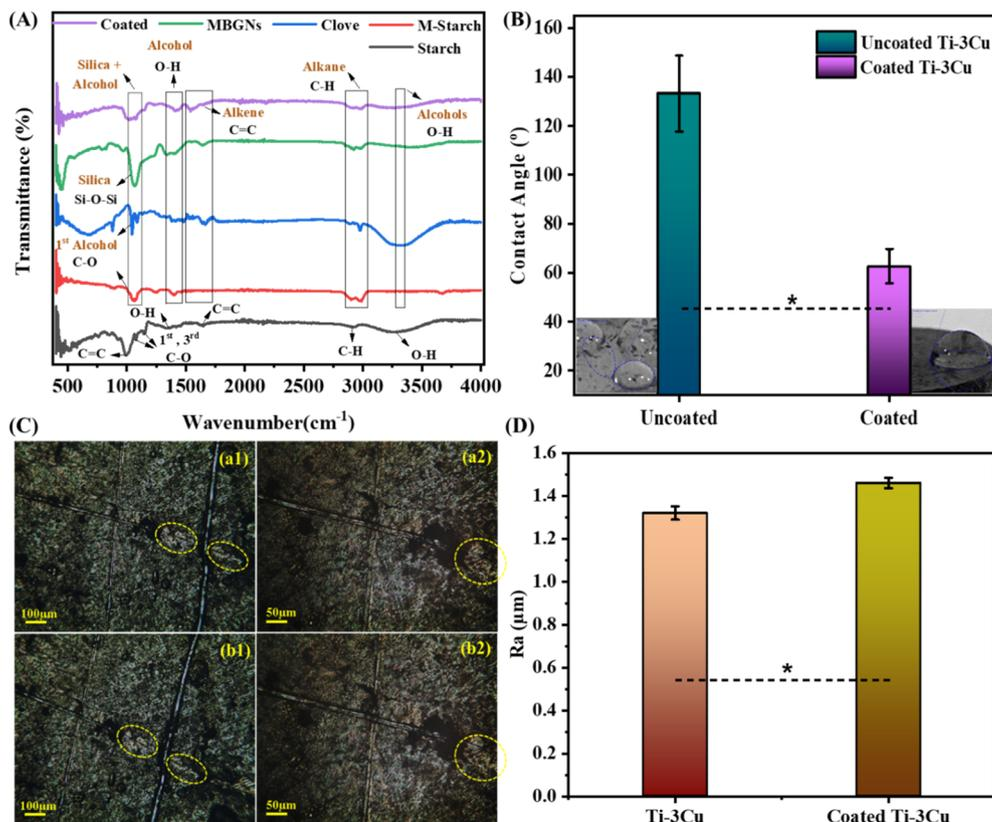
Fig. 5 (A) FTIR spectroscopy, (B) wettability analysis, (C) adhesion testing (a1 and a2) crosshatch test and (b1 and b2) tape test, and (D) surface roughness analysis ( $p < 0.05$ ) of pristine and composite-coated Ti-3Cu substrates.
