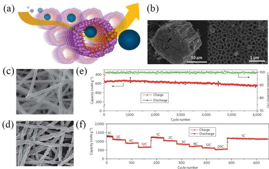
Fig. 7 (a) Schematic diagram of Li<sup>+</sup> pathways in Si nanotubes; (b) FE-SEM image of Si nanotubes. (c) SEM image of double-walled Si nanotubes (DWSiNT); (d) DWSiNT after 2000 cycles; (e) cycling performance curve at a rate of 10C and 12 °C; (f) rate performance plot of DWSiNT.
