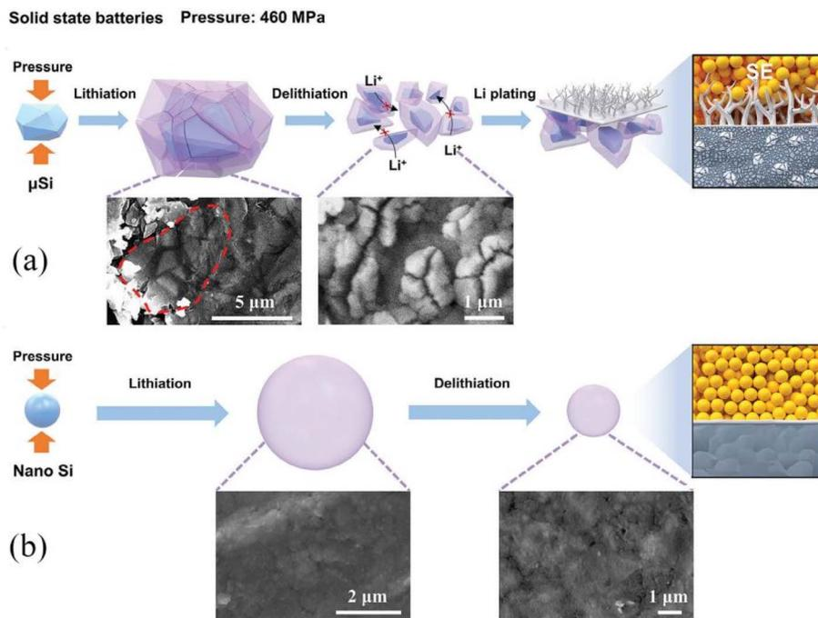
Fig. 5 Schematic illustration of the size effect during the charge–discharge process of batteries with Si anodes of different dimensions: (a) micro-silicon; (b) nano-silicon.
