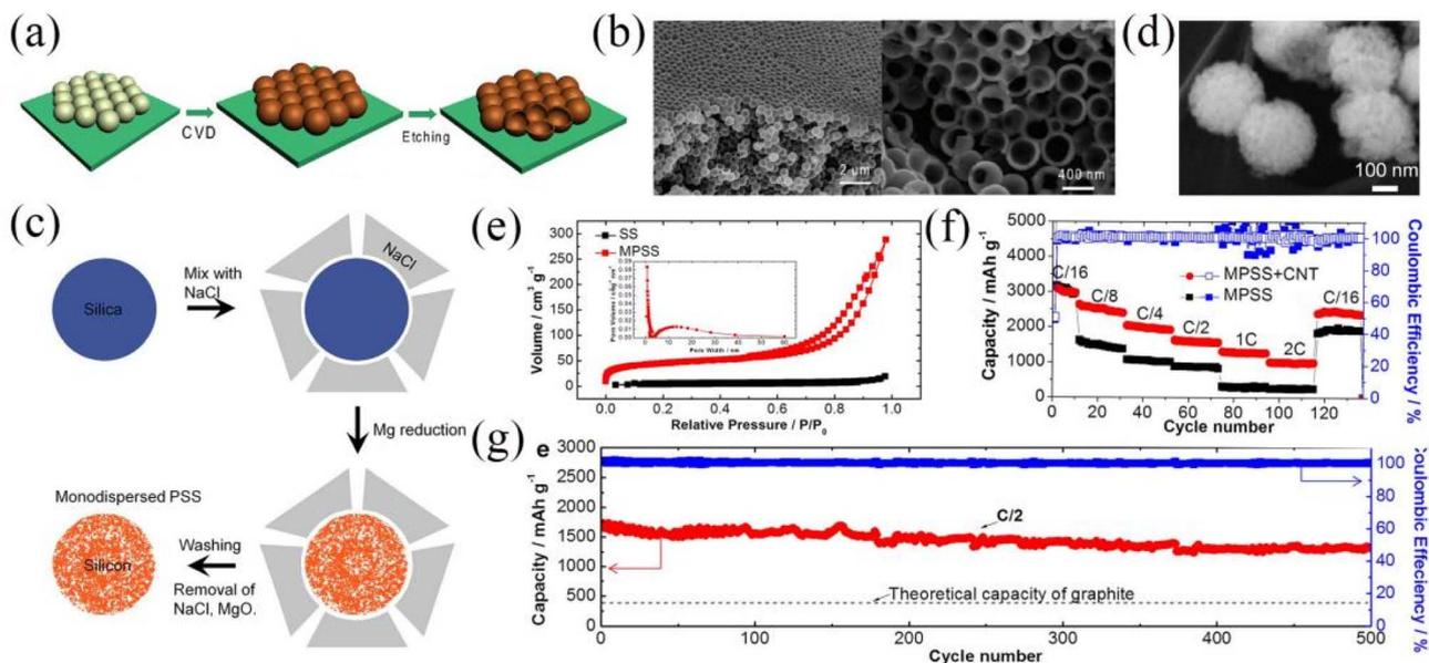
**Fig. 8** (a) Schematic illustration of the synthesis of Si hollow nanospheres; (b) SEM images of hollow Si nanospheres in the initial state and after scratch treatment. (c) Schematic illustration of the synthesis of MPSS; (d) SEM image of MPSS; (e) BET specific surface area measurement of SS and MPSS from  $N_2$  adsorption–desorption isotherms; (f) rate performance plots of MPSS electrodes with and without 2% CNTs; (g) cycling performance and CE curves of MPSS electrodes at 0.5C rate.
