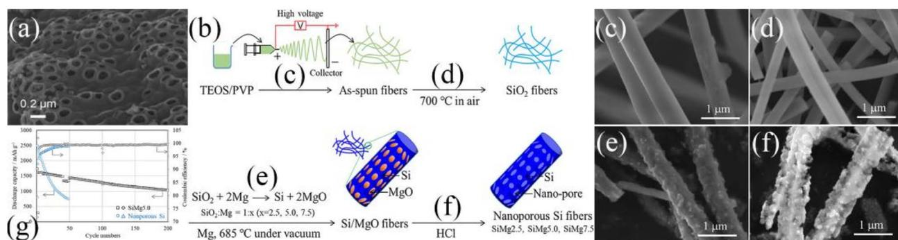
**Fig. 9** (a) SEM image of porous Si particles. (b) Schematic illustration of the synthesis process for nanoporous Si fibers; SEM images of each step during the MPSS preparation: (c) as-spun fibers; (d)  $SiO_2$  fibers after calcination in air; (e)  $SiMg_{5.0}$  before HCl etching and (f) SEM image of  $SiMg_{5.0}$ . (g) Cycling performance curves of  $SiMg_{5.0}$  and nonporous Si anodes.
