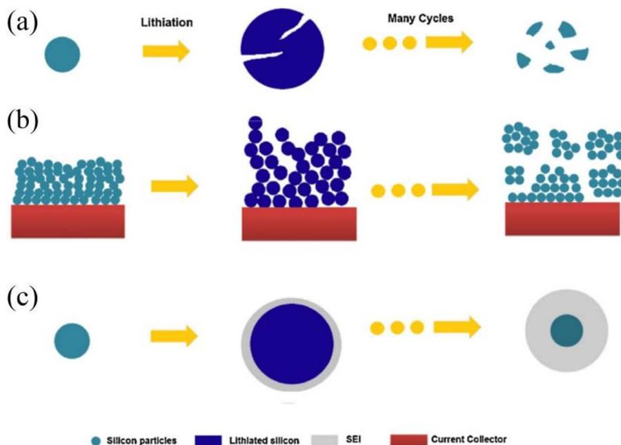
Fig. 2 Failure mechanisms of Si:<sup>2,17</sup> (a) extrusion and pulverization; (b) electrode detachment; (c) SEI evolution.
