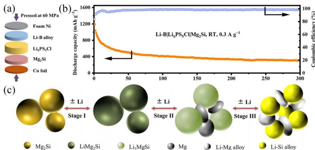
Fig. 4 (a) Layer-by-layer stacking process of the  $\text{Mg}_2\text{Si}$  battery; (b) cycling performance at a current rate of  $0.3 \text{ A g}^{-1}$ ; (c) schematic illustration of the charging/discharging processes of  $\text{Mg}_2\text{Si}$ .
