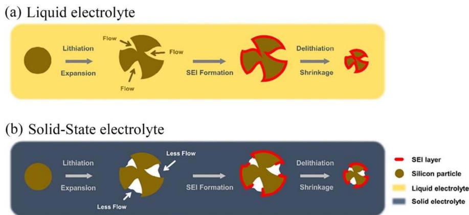
Fig. 3 The formation process of SEI in Si anodes:<sup>10</sup> (a) liquid electrolyte; (b) solid-state electrolyte.
