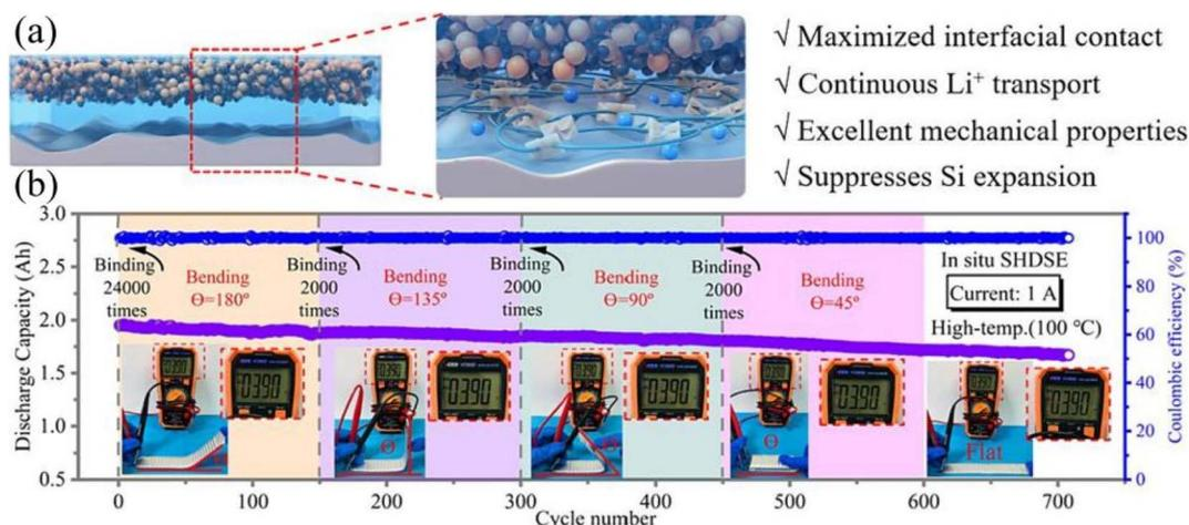
Fig. 15 (a) Schematic diagram of the Li|SHDSE|Si-SHDSE battery; (b) cycling performance curves of the SHDSE-based Si|LiCoO<sub>2</sub> pouch cell under harsh operating conditions of high temperature and continuous damage.
