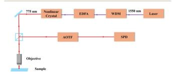
Fig. 1 The sketch of the experiment setup. A mode-locked laser operating at a wavelength of 1550.9 nm serves as the pump source, generating second harmonic (SH) light at  $\sim$  775 nm. An acoustic-optic tunable filter (AOTF)-based selective single-photon detector (SPD) detects the resulting Raman output signal.
