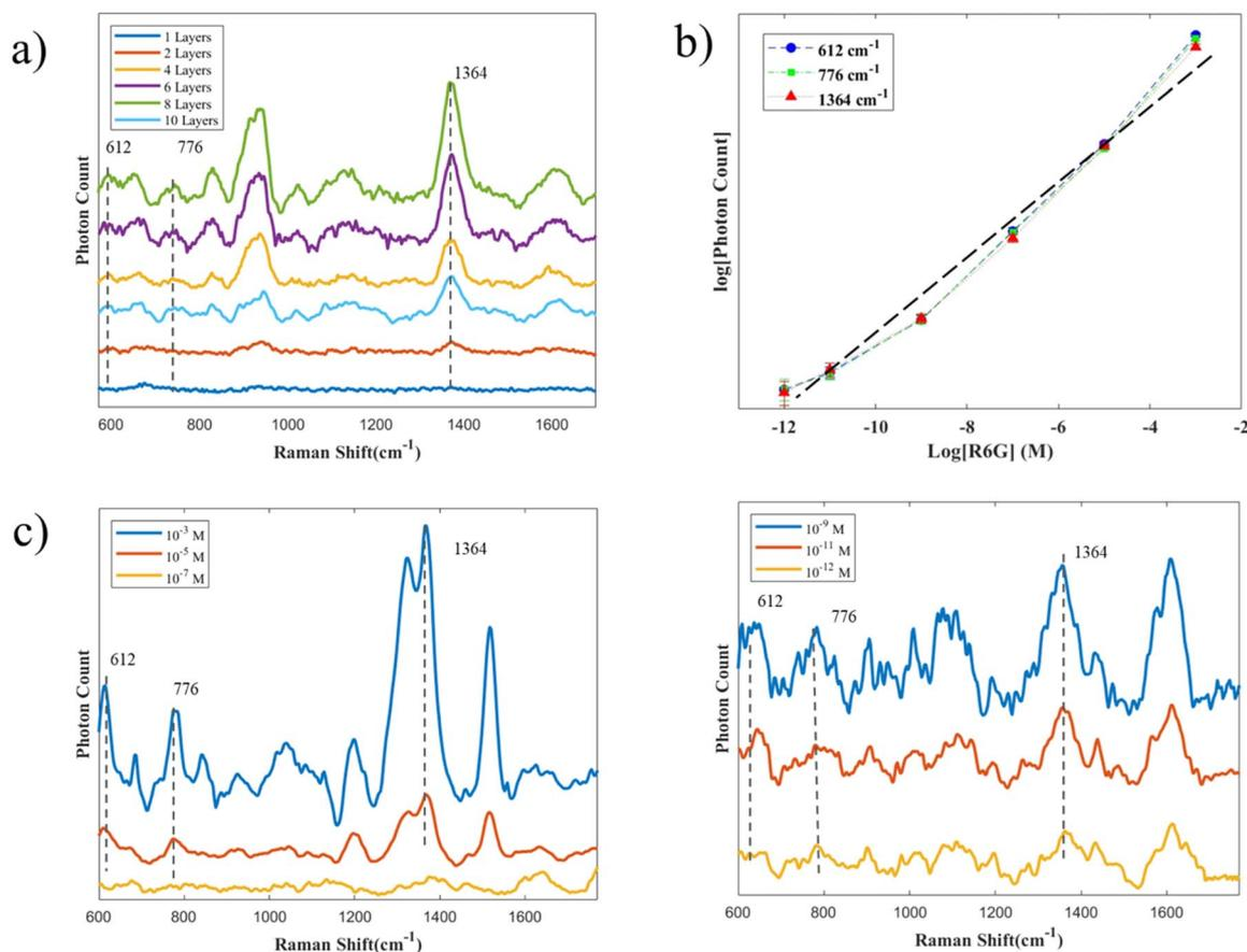
**Fig. 4** Sensitivity and reproducibility of 3D AgNPs substrate in SERS (a) Raman spectra of the  $n$ -layer AgNPs substrate ( $n = 1, 2, 4, 6, 8, 10$ ). (b) The corresponding relationship between Raman intensity and detected concentrations. (c) SERS spectra were obtained from the 8-layer structure from different concentrations of R6G.
