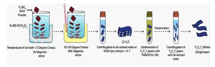
Fig. 1 Synthesis process of  $Ti_3C_2T_x$  (etching & delamination).
