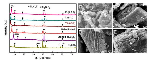
Fig. 2 (a) XRD pattern of MAX  $T_{i_3}SiC_2$  (green), etched MXene  $T_{i_3}C_2T_x$  (purple), delaminated MXene (red), and  $T_1$ ,  $T_2$ ,  $T_3$  nanocomposites with the best sample  $T_1$  (brown), (b) scanning electron microscopy (SEM) images of  $T_{i_3}SiC_2$  MAX phase at 5  $\mu$ m, (c) etched  $T_{i_3}C_2T_x$  MXene, (d) delaminated MXene at 1  $\mu$ m, (e) nanocomposite of Er@  $T_{i_3}C_2T_x$  at 1  $\mu$ m.
