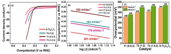
Fig. 5 (a) Polarization curve of HER against RHE, (b) Tafel slope of delaminated MXene  $Ti_3C_2T_x$  and  $T_1$  nanocomposite, (c) comparison of the current density at 10 mA cm<sup>-2</sup> ( $\eta_{10}$ ) and 20 mA cm<sup>-2</sup> ( $\eta_{20}$ ).
