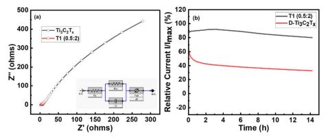
Fig. 6 (a) EIS curves of delaminated  $Ti_3C_2T_x$  MXene and Er intercalated  $Ti_3C_2T_x$  or  $T_1$  (0.5 : 2) nanocomposite along with an inset equivalent circuit. (b) Chronoamperometry curves of delaminated  $Ti_3C_2T_x$  MXene and Er intercalated  $Ti_3C_2T_x$  or T1 (0.5 : 2) for 14 h.
