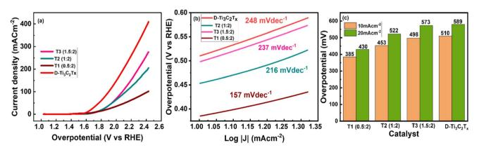
Fig. 4 (a) Polarization curve of OER against RHE, (b) Tafel slope of delaminated MXene  $Ti_3C_2T_x$  and  $T_1$  nanocomposite, (c) comparison of the current density at 10 mA cm<sup>-2</sup> ( $\eta_{10}$ ) and 20 mA cm<sup>-2</sup> ( $\eta_{20}$ ).
