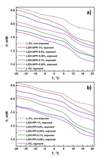
Fig. 15 DSC curves measured in the glass transition range for the latex films exposed to UV irradiation in contrast to the non-exposed reference latex film L 0%: L/DV-bPPI series (a); L/DV-PPI series (b).
