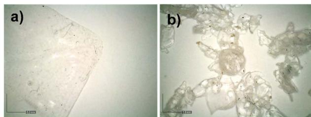
Fig. 7 Macroscopic appearance of the reference latex polymer film L 0% before (a) and after (b) the UV irradiation. The scale bars indicate 5 mm.
