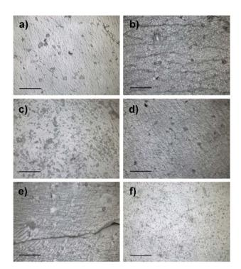
Fig. 12 Micrographs for the latex films containing DV-PPI derivative at different concentrations: L/DV-PPI 0.05% exposed to UV irradiation (a), L/DV-PPI 0.1% exposed to UV irradiation (b), L/DV-PPI 0.25% exposed to UV irradiation (c), L/DV-PPI 0.5% (d), L/DV-PPI 1% exposed to UV irradiation (e), L/DV-PPI 1% non-exposed (f). The scale bars indicate 200  $\mu m$ .
