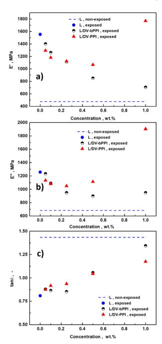
Fig. 16 Mechanical properties evaluated using DMA for the latex films exposed to UV irradiation, in contrast to the non-exposed reference latex film L 0%: (a) storage modulus (E'), (b) loss modulus (E''), (c) loss factor ( $\tan \delta$ ).
