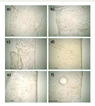
Fig. 8 Macroscopic appearance of the latex polymer films containing DV-bPPI derivative at different concentrations: L/DV-bPPI 0.05% exposed to UV irradiation (a), L/DV-bPPI 0.1% exposed to UV irradiation (b), L/DV-bPPI 0.25% exposed to UV irradiation (c), L/DV-bPPI 0.5% (d), L/DV-bPPI 1% exposed to UV irradiation (e), L/DV-bPPI 1% non-exposed (f). The scale bars indicate 5 mm.
