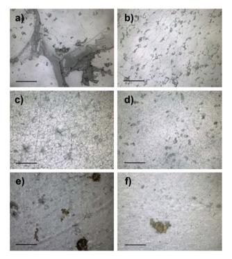
Fig. 11 Micrographs for the latex films containing DV-bPPI derivative at different concentrations: L/DV-bPPI 0.05% exposed to UV irradiation (a), L/DV-bPPI 0.1% exposed to UV irradiation (b), L/DV-bPPI 0.25% exposed to UV irradiation (c), L/DV-bPPI 0.5% (d), L/DV-bPPI 1% exposed to UV irradiation (e), L/DV-bPPI 1% non-exposed (f). The scale bars indicate 200 µm.
