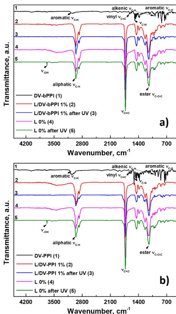
Fig. 14 FTIR spectra of monomers (UVAs), unexposed and UV-exposed latexes: DV-bPPI (a); DV-PPI (b).
