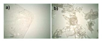
Fig. 7 Macroscopic appearance of the reference latex polymer film L 0% before (a) and after (b) the UV irradiation. The scale bars indicate 5 mm.
