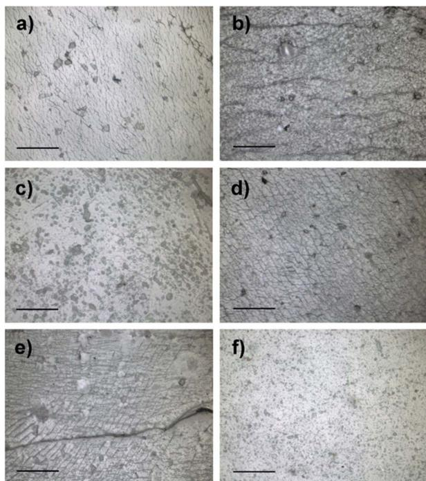
Fig. 12 Micrographs for the latex films containing DV-PPI derivative at different concentrations: L/DV-PPI 0.05% exposed to UV irradiation (a), L/DV-PPI 0.1% exposed to UV irradiation (b), L/DV-PPI 0.25% exposed to UV irradiation (c), L/DV-PPI 0.5% (d), L/DV-PPI 1% exposed to UV irradiation (e), L/DV-PPI 1% non-exposed (f). The scale bars indicate 200  $\mu\text{m}$ .
