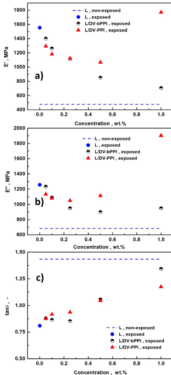
Fig. 16 Mechanical properties evaluated using DMA for the latex films exposed to UV irradiation, in contrast to the non-exposed reference latex film L 0%: (a) storage modulus ( $E'$ ), (b) loss modulus ( $E''$ ), (c) loss factor ( $\tan \delta$ ).
