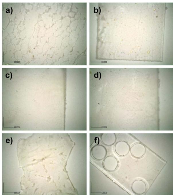
Fig. 9 Macroscopic appearance of the latex polymer films containing **DV-PPI** derivative at different concentrations: L/**DV-PPI** 0.05% exposed to UV irradiation (a), L/**DV-PPI** 0.1% exposed to UV irradiation (b), L/**DV-PPI** 0.25% exposed to UV irradiation (c), L/**DV-PPI** 0.5% (d), L/**DV-PPI** 1% exposed to UV irradiation (e), L/**DV-PPI** 1% non-exposed (f). The scale bars indicate 5 mm.
