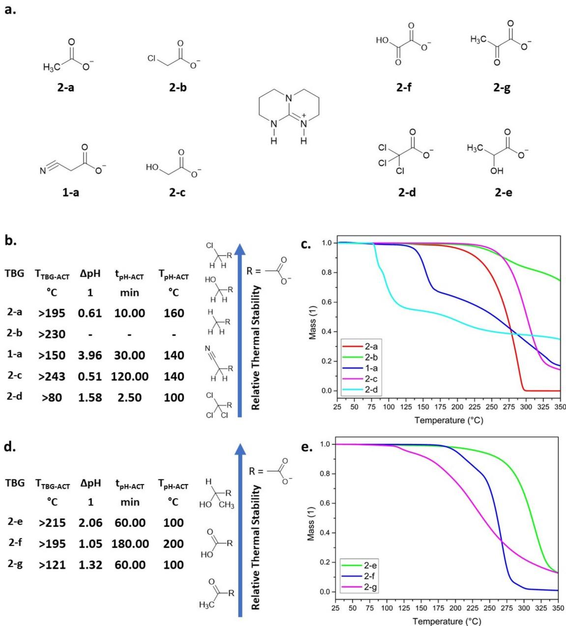
Fig. 2 Influence of different stabilization groups from acetate derivatives on the properties of TBD releasing QASs. (a) Chemical structures of the synthesized TBGs 2-a–g. (b and d) Summary of  $T_{\text{TBG-ACT}}$ ,  $\Delta\text{pH}$  after activation,  $t_{\text{pH-ACT}}$ , and  $T_{\text{pH-ACT}}$ ; including a schematic representation of the relative thermal stability of the acetate derivatives. TGA analysis of the TBGs (c) 1-a, 2-a–g and (e) 2-e–g.
