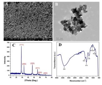
Fig. 1 SEM (A), TEM (B), XRD (C), and ATR-FTIR (D) of CeO<sub>2</sub>.
