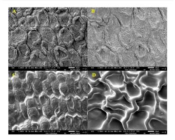
Fig. 5 SEM images of the peel surface of banana without coating (A) and coated with Kadozan (B), CS (C), and CS-1.5%-hCeO<sub>2</sub> (D).
