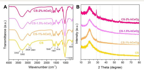
Fig. 4 ATR-FTIR (A) and XRD (B) of films.
