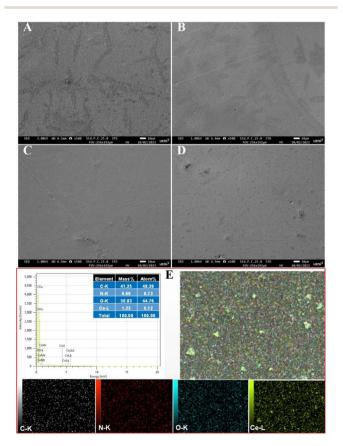
Fig. 2 SEM image of CS (A), CS-1%-hCeO $_2$  (B), CS-1.5%-hCeO $_2$  (C), CS-2%-hCeO $_2$  (D), and EDX mapping of CS-1.5%-hCeO $_2$  film (E).
