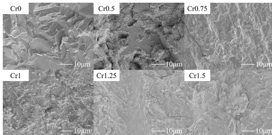
Fig. 7 Fracture surfaces of HfMoTaTiZrCr<sub>x</sub> RHEAs.
