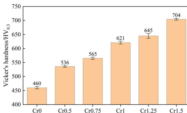
Fig. 5 Vicker's hardness of HfMoTaTiZrCr<sub>x</sub> (x = 0~1.5) RHEAs.
