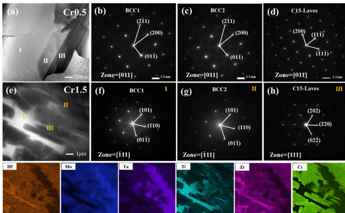
Fig. 4 Bright-field TEM image, corresponding elemental distribution maps and selective area electron diffraction patterns of areas I, II, and III of (a–d) HfMoTaTiZrCr<sub>0.5</sub> RHEA, (e–h) HfMoTaTiZrCr<sub>1.5</sub>.
