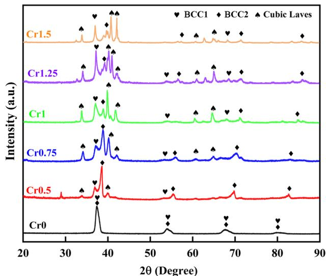
Fig. 1 XRD patterns of as-cast HfMoTaTiZrCr<sub>x</sub> RHEAs.
