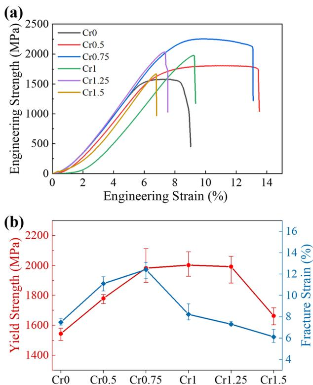
Fig. 6 (a) RT compressive stress–strain curves of as-cast HfMoTaTiZrCr<sub>x</sub> ( $x = 0, 0.5, 0.75, 1, 1.25, 1.5$ ) RHEAs and (b) the derived  $\sigma_{0.2}$  and  $\epsilon_f$  at different Cr content. Note: data for HfMoTaTiZr and HfMoTaTiZrCr<sub>0.5</sub>, originally reported in our previous work,<sup>17</sup> are strategically reused here to enable direct quantification of chromium's compositional effects.
