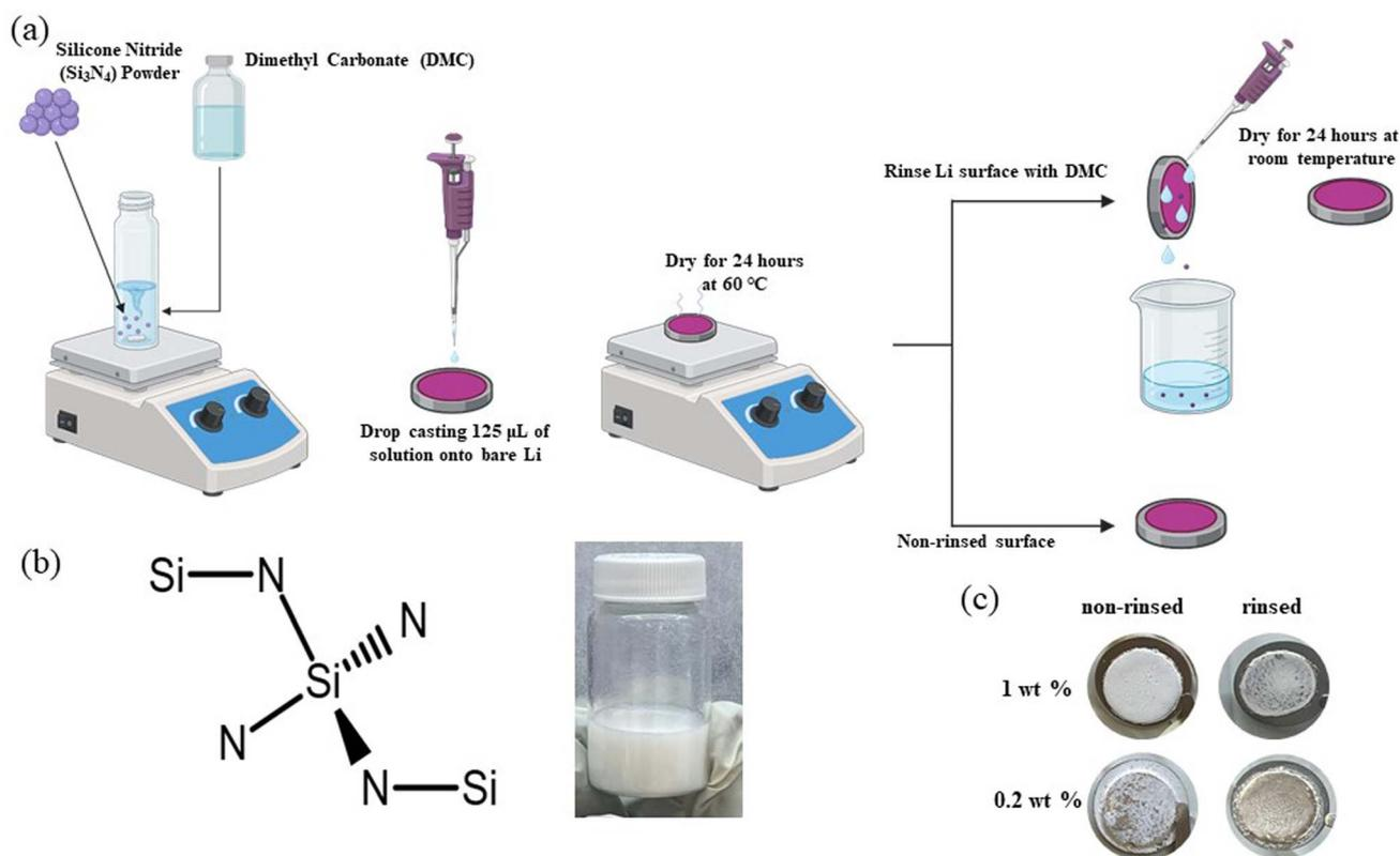
Fig. 1 (a) Schematic illustration showing the formation of the artificial nano  $\text{Si}_3\text{N}_4$  layer on lithium metal. (b) Structural representation of  $\text{Si}_3\text{N}_4$  and 1 wt% nano  $\text{Si}_3\text{N}_4$  dispersed in DMC. (c) Comparative analysis of 1 wt% and 0.2 wt% samples, including rinsed and non-rinsed conditions.
