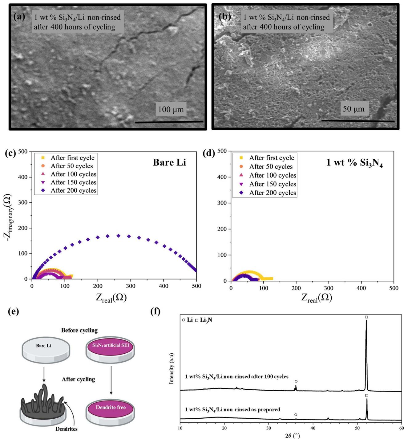
Fig. 4 (a and b) Top-view SEM images of 1 wt% nano  $\text{Si}_3\text{N}_4/\text{Li}$  samples, non-rinsed, after 400 hours of cycling. (c and d) Electrochemical impedance of bare Li and 1 wt% Li/nano  $\text{Si}_3\text{N}_4$  after  $x$  ( $x = 1, 50, 100, 50, 200$ ) cycles. (e) Dendrite growth schematic (f) XRD patterns of 1 wt% Li/nano  $\text{Si}_3\text{N}_4$  non-rinsed as prepared and after 100 cycles samples on a stainless-steel substrate.
