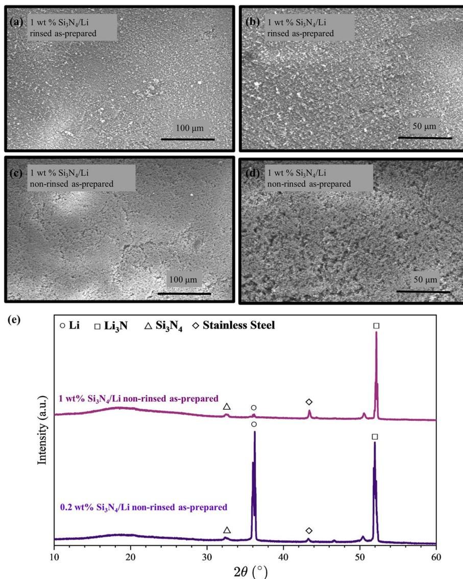
Fig. 2 (a–d) Top-view SEM images of 1 wt% nano  $\text{Si}_3\text{N}_4/\text{Li}$  samples, rinsed and non-rinsed samples in their as-prepared state. (e) XRD patterns of 1 wt% and 0.2 wt% nano  $\text{Si}_3\text{N}_4/\text{Li}$  non-rinsed as-prepared samples on a stainless-steel substrate.
