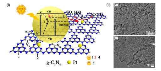
Fig. 5 (i) Schematic of  $g-C_3N_4$  with nitrogen vacancies. (ii) TEM images of CN-525. (This figure has been adapted from ref. 36 with permission from ACS Sustainable Chemistry & Engineering, copyright 2017).
