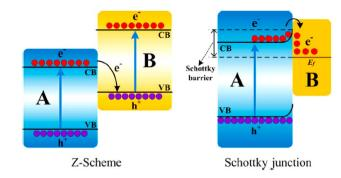
**Fig. 9** Diagram of charge transfer for Z-scheme and Schottky junction systems. (A and B) Two different semiconductor materials. (This figure has been adapted from ref. 75 with permission from MDPI Catalysts, copyright 2020).
