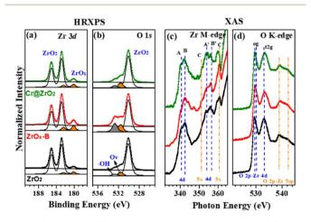
Fig. 2 (a) Zr 3d and (b) O 1s core-level HR-XP spectra and (c) Zr M-edge and (d) O K-edge X-ray absorption spectra of  $ZrO_2$  (bottom),  $ZrO_2$ -B (middle), and  $Cr@ZrO_2$  (top) NPs. (This figure has been adapted from ref. 22 with permission from ResearchGate Nature Portfolio, copyright 2022).
