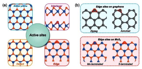
Fig. 7 (a) Different active sites on 2D materials. (b) Typical edge sites on 2D materials, including armchair and zigzag edges on graphene, and Mo/ S-terminated zigzag edges on 2D MoS<sub>2</sub>. (This figure has been adapted from ref. 50 with permission from Wiley Advanced, copyright 2025).
