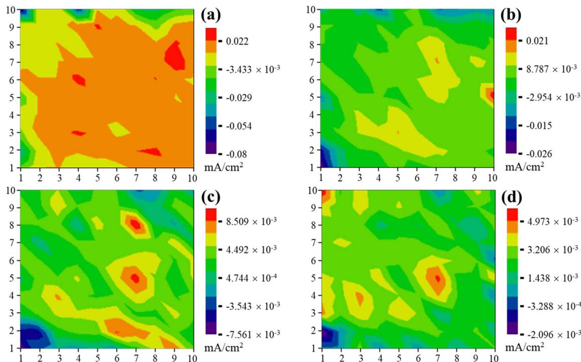
Fig. 8 Galvanic current map distributed to the WBE surface after (a) 1 h immersion in a CO<sub>2</sub>-saturated 0.01 M NaCl solution without inhibitor addition and after 24 h with (b) 0.4, (c) 1.2, and (d) 2.4 mM PrCl<sub>3</sub> additions.
