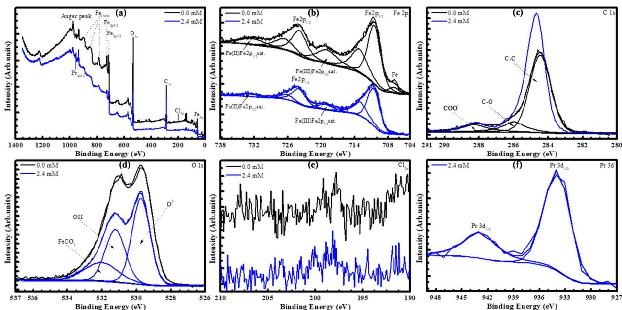
Fig. 3 Survey and narrow XPS spectra of MS surfaces immersed in a CO<sub>2</sub>-saturated 0.01 M NaCl solution with 0.0 and 2.4 mM PrCl<sub>3</sub> addition: (a) survey, (b) Fe 2p, (c) C 1s, (d) O 1s, (e) Cl 2p, and (f) Pr 3d spectra.
