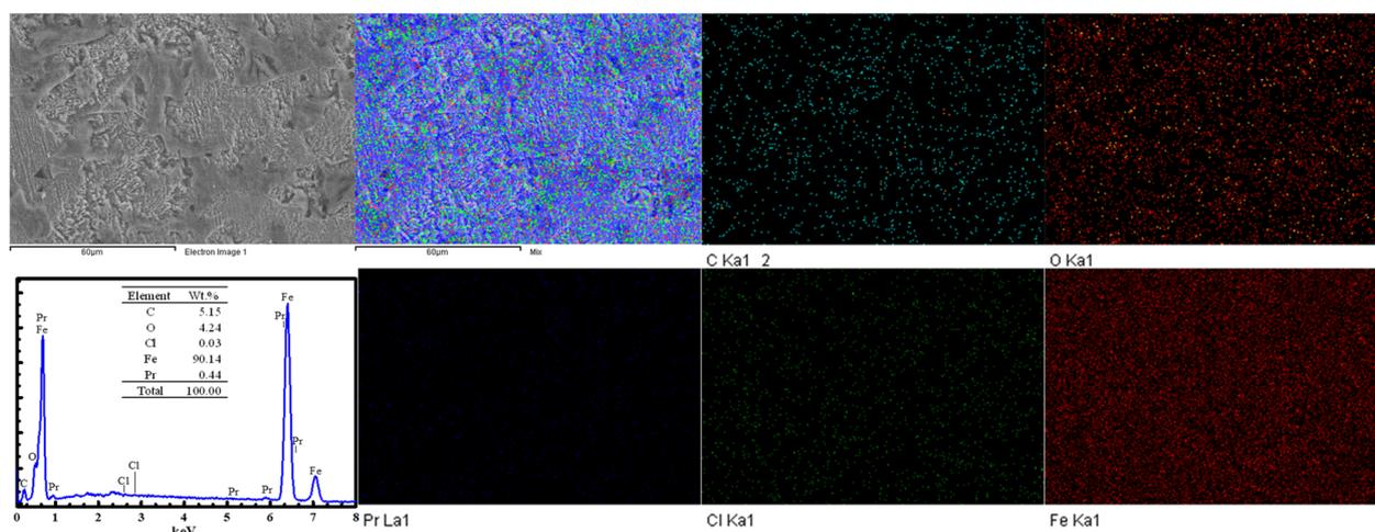
Fig. 2 SEM/EDS mapping of the substrate surface after 72 hours corrosion in a CO<sub>2</sub>-saturated 0.01 M NaCl solution with 2.4 mM PrCl<sub>3</sub> addition.
