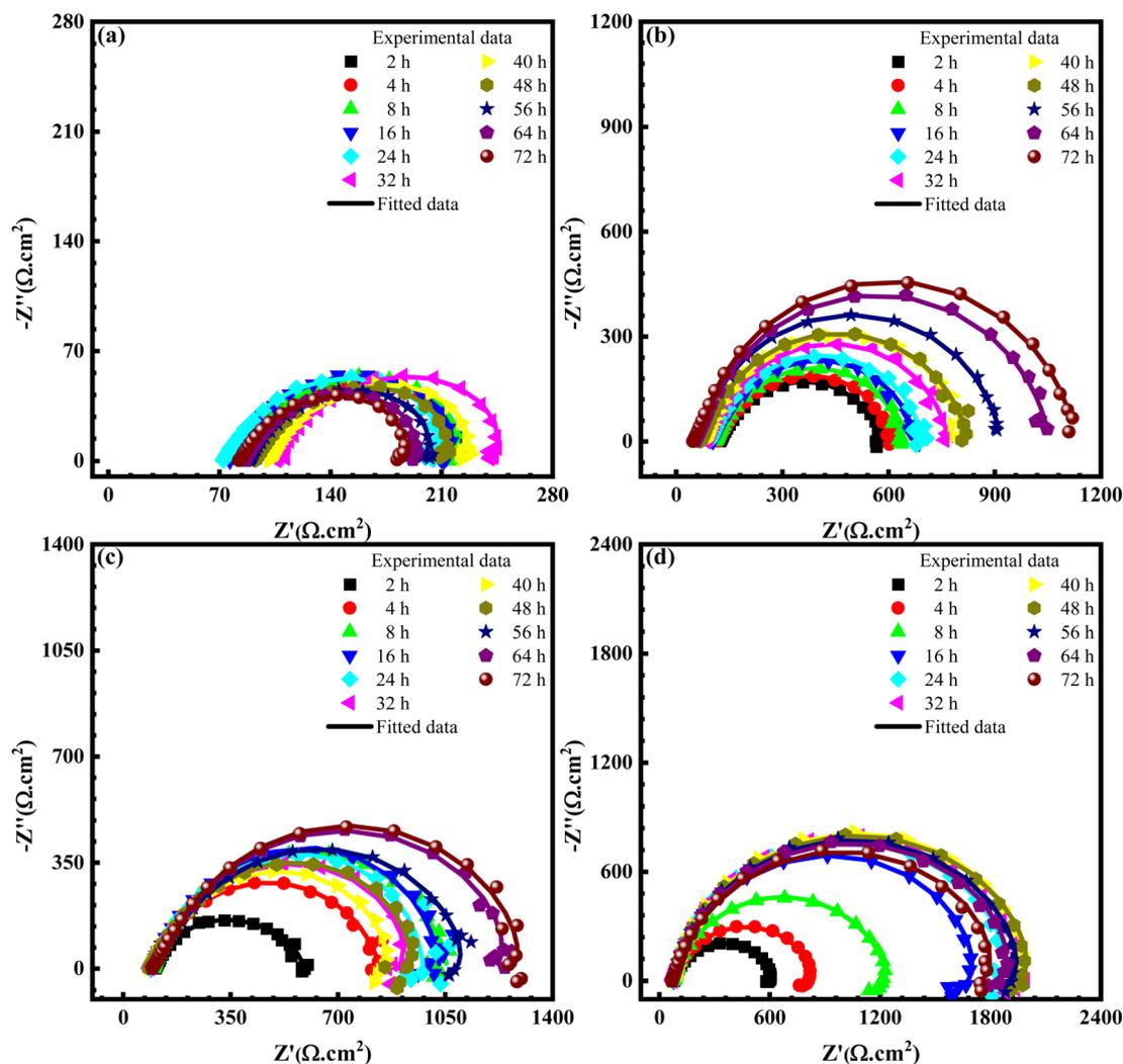
**Fig. 5** Nyquist plots representing the experimental and fitted EIS results of mild steel during 72 hours corrosion in CO<sub>2</sub>-saturated 0.01 M NaCl solutions with (a) 0.0, (b) 0.4, (c) 1.2, and (d) 2.4 mM PrCl<sub>3</sub> addition.
