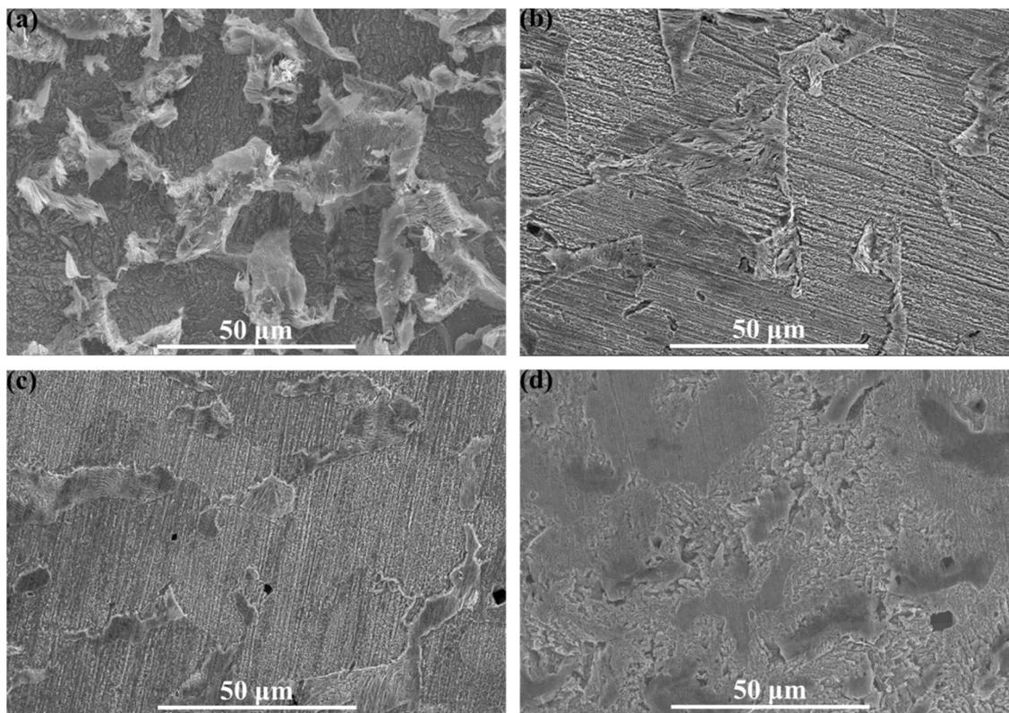
Fig. 1 Scanning electron microscopy images showing morphologies after 72 hours corrosion in a CO<sub>2</sub>-saturated 0.01 M NaCl solution with: (a) 0.0, (b) 0.4, (c) 1.2, and (d) 2.4 mM PrCl<sub>3</sub> addition.
