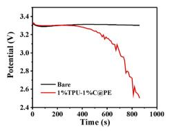
Fig. 8 The voltage cut-off behavior of 1% TPU-1% C@PE battery in  $160~^{\circ}\text{C}$  environment.
