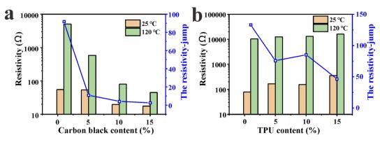
Fig. 3 Electrical properties of carbon-based composites: (a) C@PE with 1–15 wt% carbon black showing resistance and resistance increase ratio; (b) PE/CB composites with 1–15 wt% TPU (fixed 1 wt% CB content).
