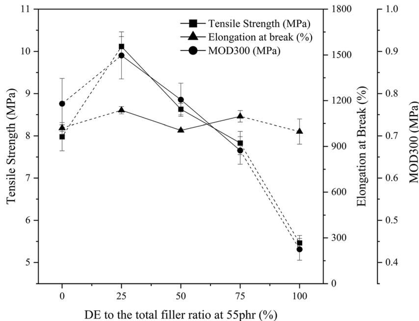
Fig. 5 Variation of tensile strength, elongation at break, and MOD300 with DE to the total filler ratio at 55 phr\*. \* Note that the variation of properties from 0–25 and from 75–100 might exhibit a notable variation. As it is not validated using experimental data, it has been denoted using a dotted line.
