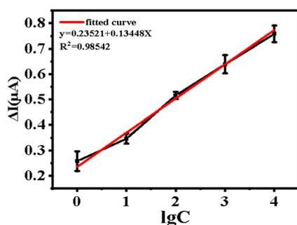
Fig. 5 Calibration curve corresponding to different target mRNA concentrations. (Error bars represent the standard deviation of three independent measurements.)
