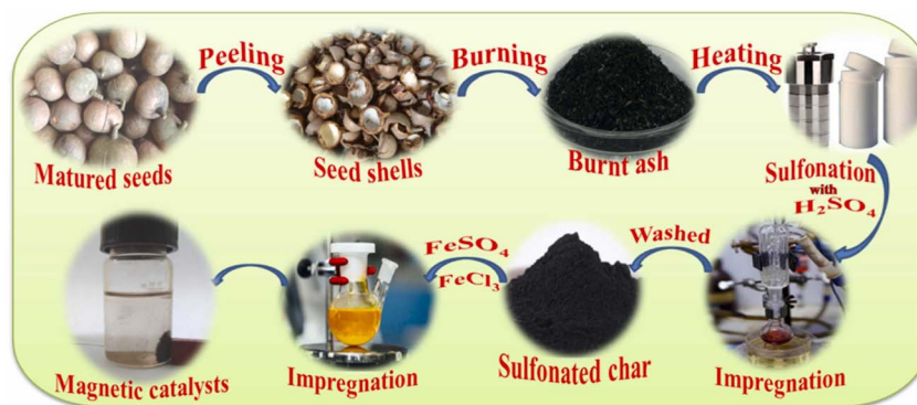
Fig. 6 Synthesis processes of the \text{Fe}_3\text{O}_4@biochar@SO_3H nanocatalyst. Ref. 84, reprinted with permission of copyright© (2024) from Elsevier.
