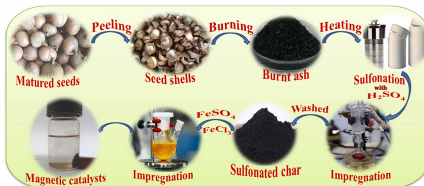
Fig. 6 Synthesis processes of the \text{Fe}_3\text{O}_4\text{@biochar@SO}_3\text{H} nanocatalyst. Ref. 84, reprinted with permission of copyright© (2024) from Elsevier.
