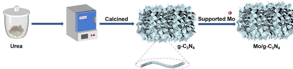
Fig. 4 Synthesis process of the Mo/g-C<sub>3</sub>N<sub>4</sub> catalyst. Ref. 58, reprinted with permission of copyright© (2023) from Elsevier.
