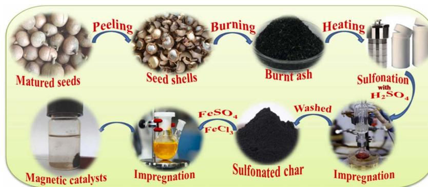
Fig. 6 Synthesis processes of the  $\text{Fe}_3\text{O}_4@biochar@SO_3H$  nanocatalyst. Ref. 84, reprinted with permission of copyright© (2024) from Elsevier.
