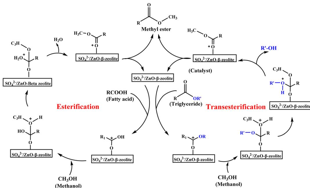
Fig. 2 Plausible mechanism for the concurrent esterification and transesterification reactions by  $\text{SO}_4^{2-}/\text{ZnO}-\beta$ -zeolite. Ref. 32, reprinted with permission of copyright© (2023) open-access from the American Chemical Society.
