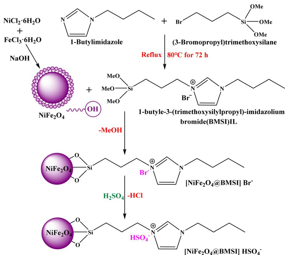
Fig. 8 Preparation methods for [NiFe<sub>2</sub>O<sub>4</sub>@BMSI]Br and [NiFe<sub>2</sub>O<sub>4</sub>@BMSI]HSO<sub>4</sub>. Ref. 116, reprinted with permission of copyright© (2021) from Elsevier.
