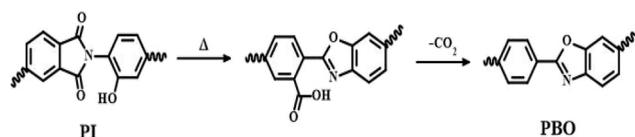
Scheme 2 Thermal rearrangement of polybenzoxazole from PI by heat treatment.
