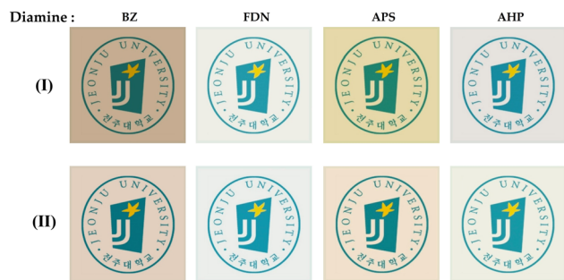
Fig. 8 Photographs of PI films based on (I) BPADA and (II) HBPDA dianhydride monomers.
