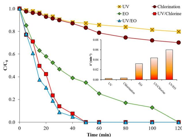
Fig. 1 Removal of ATL by chlorination, UV irradiation, EO, UV/chlorine, and UV/EO (pH 7, NaCl 500 mg  $\text{L}^{-1}$ , 1 UV lamp, CD 5 mA  $\text{cm}^{-2}$ ,  $n = 3$ ).
