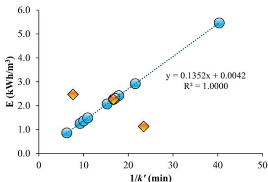
Fig. 4 Correlation between specific energy consumption and  $1/k'$  (circles = fixed CD at  $5 \text{ mA cm}^{-2}$ , diamonds = CD values of 2.5, 5, and  $10 \text{ mA cm}^{-2}$ ).
