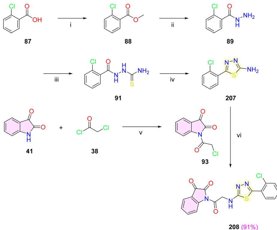
Scheme 40 Synthesis of isatin–thiadiazole hybrid **208**. Reagents and conditions: (i)  $\text{H}_2\text{SO}_4$ , MeOH, reflux, 16 h; (ii)  $\text{N}_2\text{H}_4 \cdot \text{H}_2\text{O}$ , reflux, 4 h; (iii) KSCN, HCl,  $\text{H}_2\text{O}$ , reflux, 5 h; (iv)  $\text{H}_2\text{SO}_4$ , stirring, r.t., 6 h; (v) (a) reflux, 5 h; (b) stirring, r.t., 24 h; (vi) EtOH,  $\text{K}_2\text{CO}_3$ , reflux, 4 h.
