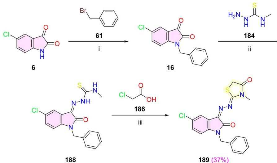
**Scheme 36** Synthesis of isatin–thiazolidine hybrid **189**. Reagents and conditions: (i)  $K_2CO_3$ , DMF, KI, 80 °C, 45 min; (ii) EtOH, *gl.* AcOH (cat.), reflux, 3 h; (iii) EtOH, AcONa (cat.), reflux, 24 h.
