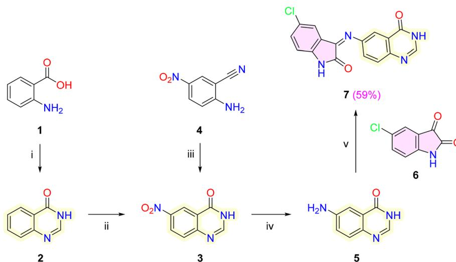
**Scheme 1** Synthesis of isatin–quinazoline **7**. Reagents and conditions: (i)  $\text{HCONH}_2$ , reflux, 6 h; (ii)  $\text{HNO}_3$ ,  $\text{H}_2\text{SO}_4$ ,  $90^\circ\text{C}$ , 30 min; (iii)  $\text{HCOOH}$ ,  $\text{H}_2\text{SO}_4$ , reflux, 1 h; (iv)  $\text{Fe}$ ,  $\text{NH}_4\text{Cl}$ ,  $i\text{PrOH}$ , reflux, 1.5 h; (v)  $\text{EtOH}$ ,  $gl.$   $\text{AcOH}$  (cat.), reflux, 4–6 h.
