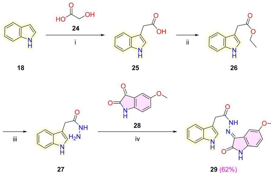
**Scheme 5** Synthesis of isatin–indole hybrid **29**. Reagents and conditions: (i) KOH, HCl, H<sub>2</sub>O; (ii) EtOH, H<sup>+</sup>, reflux, 10 h; (iii) N<sub>2</sub>H<sub>4</sub>·H<sub>2</sub>O, EtOH, reflux, 2 h; (iv) EtOH, *gl.* AcOH (cat.), reflux, 4 h.
