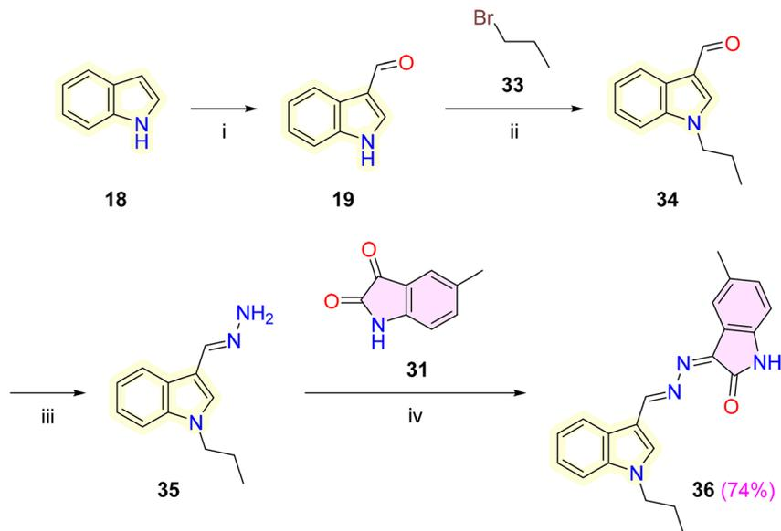
Scheme 7 Synthesis of isatin–indole hybrid **36**. Reagents and conditions: (i) DMF,  $\text{POCl}_3$ , reflux, 8 h; (ii) DMF, NaH, stirring, r.t., 24 h; (iii)  $\text{N}_2\text{H}_4 \cdot \text{H}_2\text{O}$ , EtOH, reflux, 2 h; (iv) EtOH, *gl.* AcOH (cat.), reflux, 3 h.
