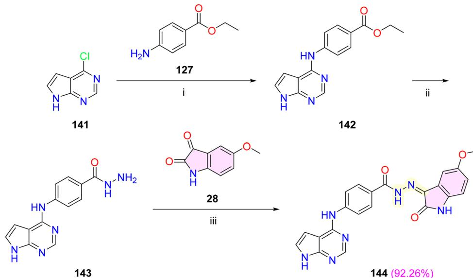
**Scheme 24** Synthesis of isatin–hydrazone hybrid **144**. Reagents and conditions: (i) EtOH, reflux, 7 h; (ii)  $\text{N}_2\text{H}_4 \cdot \text{H}_2\text{O}$ , EtOH, reflux, 5 h; (iii) EtOH, AcOH, reflux, 6–9 h.
