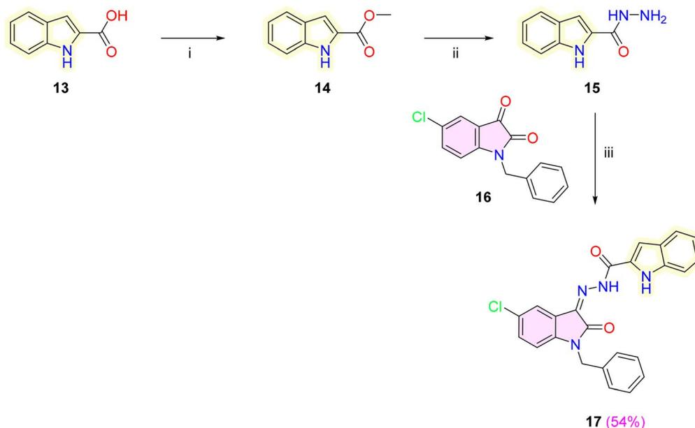
Scheme 3 Synthesis of isatin–indole hybrid **17**. Reagents and conditions: (i) MeOH, H<sub>2</sub>SO<sub>4</sub> (cat.), reflux, 4 h; (ii) N<sub>2</sub>H<sub>4</sub>·H<sub>2</sub>O, MeOH, reflux, 2 h; (iii) EtOH, *gl. AcOH* (cat.), reflux, 4 h.
