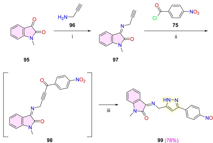
**Scheme 16** Synthesis of isatin-pyrazole hybrid **99**. Reagents and conditions: (i) MeOH, 60 °C, 9 h; (ii) PdCl<sub>2</sub>(PPh<sub>3</sub>)<sub>2</sub>, CuI, sodium laurylsulfate, K<sub>2</sub>CO<sub>3</sub>, water, 65 °C, 7 h; (iii) N<sub>2</sub>H<sub>4</sub>·H<sub>2</sub>O, 65 °C, 12 h.
