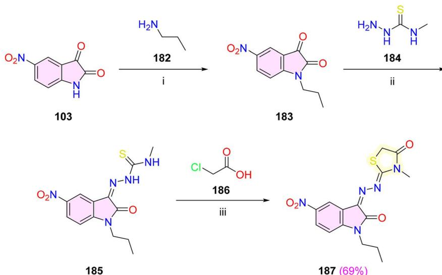
**Scheme 35** Synthesis of isatin–thiazolidine hybrid **187**. Reagents and conditions: (i)  $K_2CO_3$ , DMF, 80 °C, 45 min; (ii) EtOH, *gl.* AcOH (cat.), reflux, 2 h; (iii) EtOH, AcONa (cat.), reflux, 24 h.
