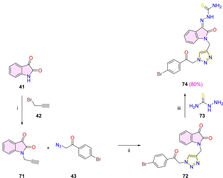
Scheme 13 Synthesis of isatin-1,2,3-triazole hybrid 74. Reagents and conditions: (i)  $K_2CO_3$ , DMF, r.t., 3 h; (ii)  $CuSO_4 \cdot 5H_2O$ , sodium ascorbate, *t*-BuOH,  $H_2O$ , r.t., sonication, 1 h; (iii) *i*PrOH, 65  $^{\circ}C$ , sonication, 1 h.
