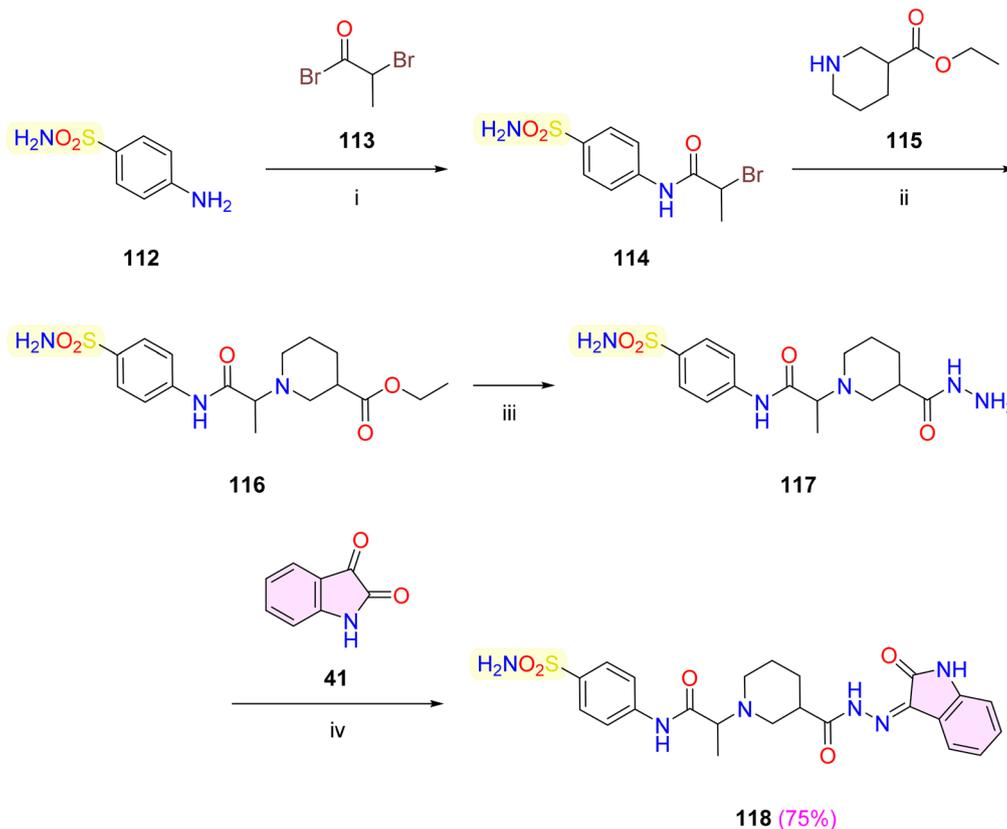
**Scheme 19** Synthesis of isatin–sulphonamide hybrid **118**. Reagents and conditions: (i) dioxane, Et<sub>3</sub>N, stirring, r.t., 20 h; (ii) acetone, K<sub>2</sub>CO<sub>3</sub>, KI, stirring, r.t., 2 h; (iii) N<sub>2</sub>H<sub>4</sub>·H<sub>2</sub>O, EtOH, reflux, 4 h; (iv) EtOH, *gl.* AcOH (cat.), reflux, 6 h.
