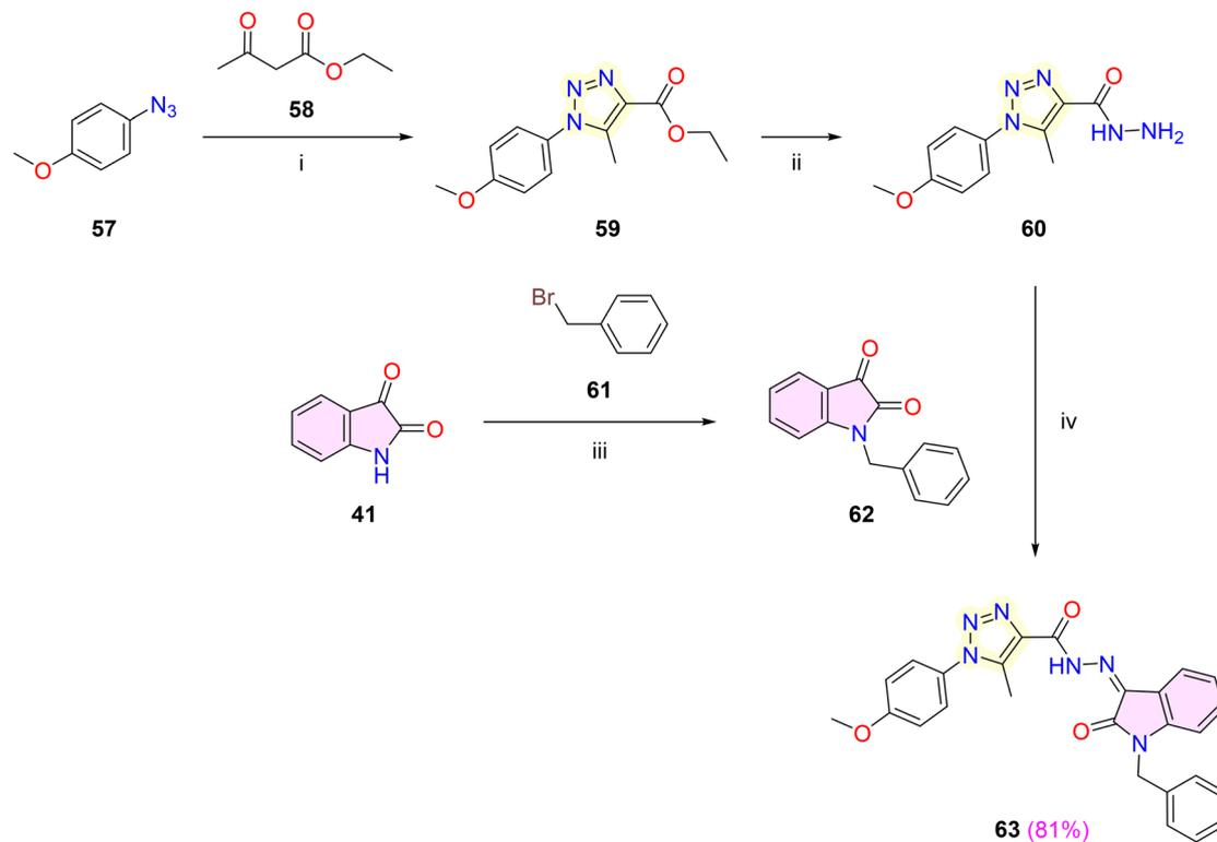
**Scheme 11** Synthesis of isatin-1,2,3-triazole hybrid **63**. Reagents and conditions: (i) Et<sub>2</sub>NH, DMSO, reflux, 6 h; (ii) N<sub>2</sub>H<sub>4</sub>·H<sub>2</sub>O, EtOH, reflux, 4 h; (iii) K<sub>2</sub>CO<sub>3</sub>, KI, MeCN, reflux, 6 h; (iv) EtOH, *gl. AcOH* (cat.), reflux, 12 h.
