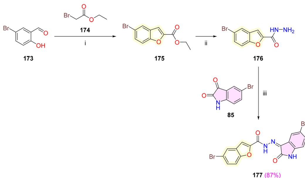
**Scheme 33** Synthesis of isatin–benzofuran hybrid **177**. Reagents and conditions: (i) MeCN, K<sub>2</sub>CO<sub>3</sub>, reflux, 4 h; (ii) N<sub>2</sub>H<sub>4</sub>·H<sub>2</sub>O, MeOH, reflux, 3 h; (iii) EtOH, *gl.* AcOH (cat.), reflux, 4–7 h.
