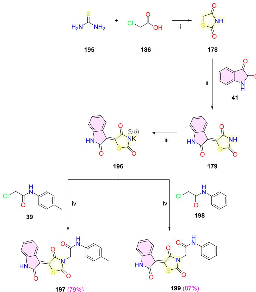
**Scheme 38** Synthesis of isatin–thiazolidine hybrids **197** and **199**. Reagents and conditions: (i) (a)  $H_2O$ , 0–5 °C, stirring, 15 min; (b) conc. HCl, reflux, 10 h; (ii) AcOH, AcONa, reflux, 6 h; (iii) KOH, EtOH, reflux; (iv) DMF,  $K_2CO_3$ , KI, reflux, 6 h.
