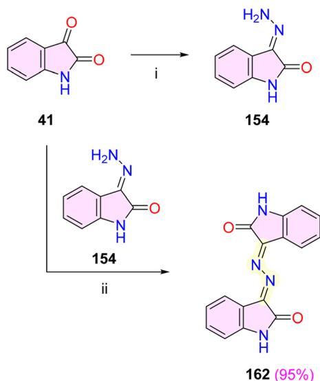
**Scheme 29** Synthesis of isatin–hydrazone hybrid **162**. Reagents and conditions: (i)  $\text{N}_2\text{H}_4 \cdot \text{H}_2\text{O}$ , EtOH, reflux, 1 h; (ii) EtOH, *gl.* AcOH (cat.), reflux, 3 h.
