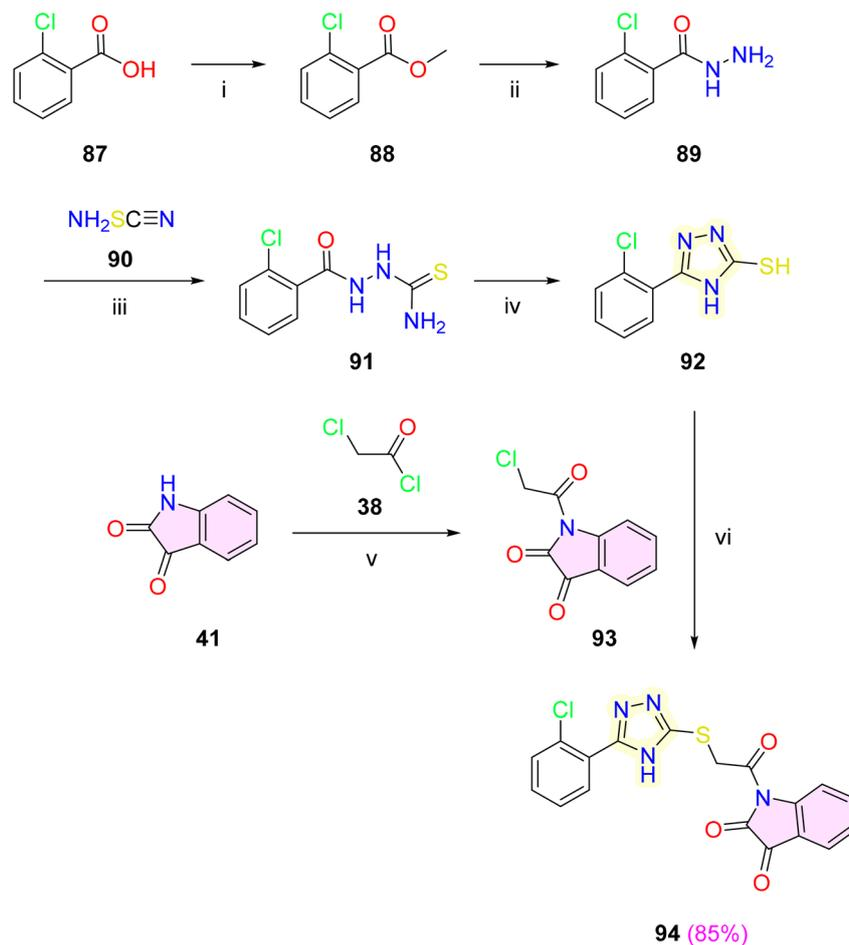
**Scheme 15** Synthesis of isatin-1,2,4-triazole hybrid **94**. Reagents and conditions: (i) MeOH, H<sub>2</sub>SO<sub>4</sub>, reflux, 8 h; (ii) N<sub>2</sub>H<sub>4</sub>·H<sub>2</sub>O, MeOH, r.t., 4 h; (iii) EtOH, conc. HCl, reflux, 6 h; (iv) NaOH, H<sub>2</sub>O, reflux, 4 h; (v) reflux, 140 °C, 5 h, r.t., overnight; (vi) EtOH, K<sub>2</sub>CO<sub>3</sub>, reflux, 4 h.
