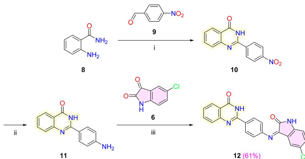
Scheme 2 Synthesis of isatin–quinazoline hybrid **12**. Reagents and conditions: (i)  $\text{CuCl}_2 \cdot 2\text{H}_2\text{O}$ , EtOH, reflux, 16 h; (ii) Fe, HCl; (iii) EtOH, *gl.* AcOH (cat.) reflux, 6 h.
