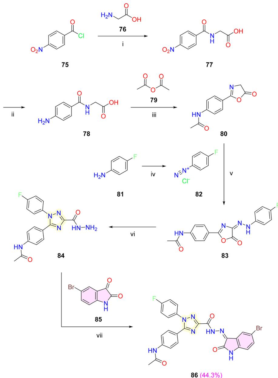
**Scheme 14** Synthesis of isatin-1,2,4-triazole hybrid **86**. Reagents and conditions: (i) NaOH (aq.), r.t., 1 h; (ii) MeOH, Pd/C, r.t., 3 h; (iii) heating, 75 °C, 40 min; (iv) HCl, NaNO<sub>2</sub>, 0–5 °C, 20 min; (v) AcONa, 0–10 °C, 3 h; (vi) EtOH, N<sub>2</sub>H<sub>4</sub>·H<sub>2</sub>O, reflux, 1 h; (vii) EtOH, AcOH, reflux, 2 h.
