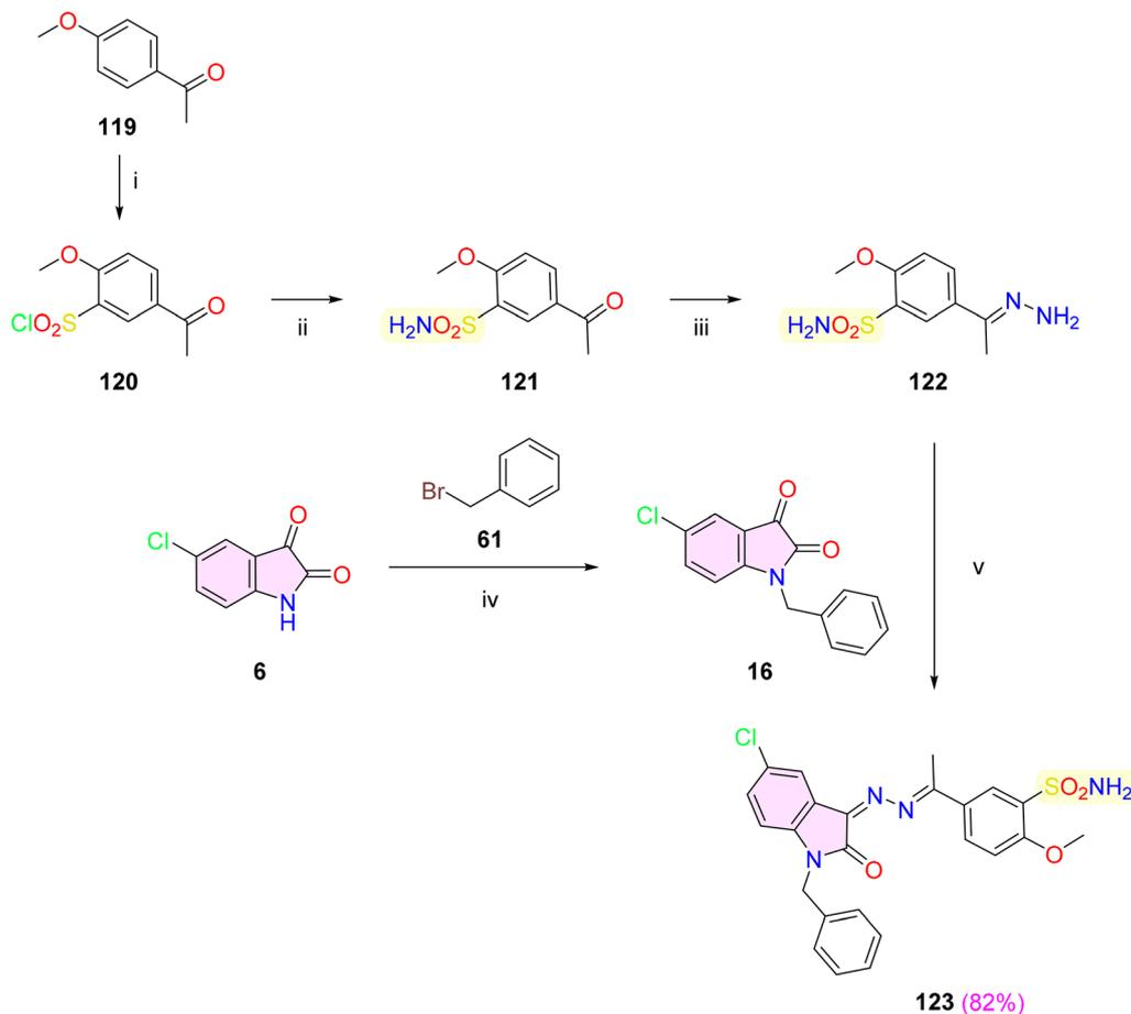
Scheme 20 Synthesis of isatin-sulphonamide hybrid **123**. Reagents and conditions: (i)  $\text{HOSO}_2\text{Cl}$ ,  $\text{SOCl}_2$ ,  $0^\circ\text{C}$ , 30 min, r.t., 26 h; (ii) EtOH, ammonia, r.t.; (iii)  $\text{N}_2\text{H}_4 \cdot \text{H}_2\text{O}$ , EtOH, *gl. AcOH* (cat.) reflux, 4 h; (iv)  $\text{K}_2\text{CO}_3$ , MeCN, reflux, 5 h; (v) EtOH, *gl. AcOH* (cat.), reflux, 4 h.
