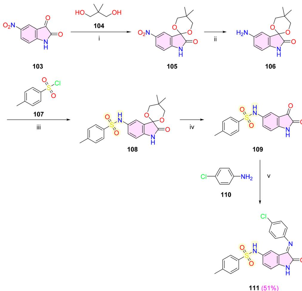
**Scheme 18** Synthesis of isatin-sulphonamide hybrid **111**. Reagents and conditions: (i) PTSA, cyclohexane, reflux, 24 h; (ii) Pd/C, H<sub>2</sub>, MeOH, r.t., 24 h; (iii) pyridine, DCM, r.t., 24 h; (iv) *gl.* AcOH, HCl, 30 °C, overnight; (v) PTSA, MeOH, 80 °C, 8 h.
