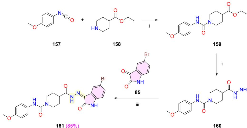
**Scheme 28** Synthesis of isatin–hydrazone hybrid **161**. Reagents and conditions: (i) toluene, stirring, 90 °C, 2 h; (ii)  $\text{N}_2\text{H}_4 \cdot \text{H}_2\text{O}$ , EtOH, reflux, 4 h; (iii) *gl.* AcOH, reflux, 4 h.
