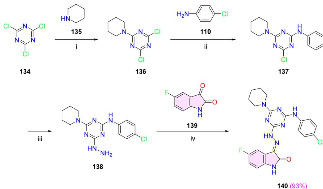
**Scheme 23** Synthesis of isatin–hydrazone hybrid **140**. Reagents and conditions: (i)  $\text{NaHCO}_3$ , 0 °C, 1–2 h; (ii) acetone,  $\text{H}_2\text{O}$ ,  $\text{NaHCO}_3$ , 0 °C to r.t., overnight; (iii)  $\text{N}_2\text{H}_4 \cdot \text{H}_2\text{O}$ , EtOH, reflux, 6–12 h; (iv) EtOH, AcOH (cat.), reflux, 6–8 h.
