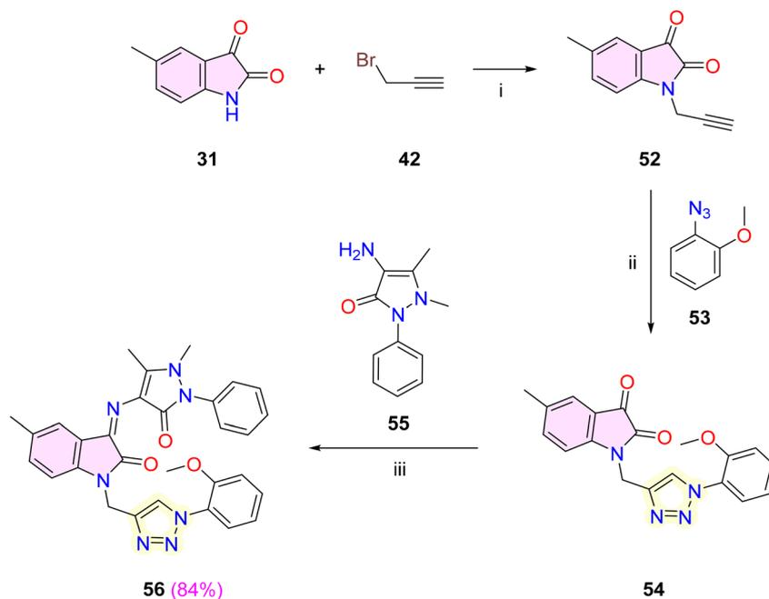
Scheme 10 Synthesis of isatin-1,2,3-triazole hybrid **56**. Reagents and conditions: (i)  $K_2CO_3$ , DMF, r.t., 4 h; (ii) sodium D-isoascorbate,  $CuSO_4 \cdot 5H_2O$ , *t*-butanol/ $H_2O$ , MW, 100 °C, 2 h; (iii) EtOH, r.t., 2 h.
