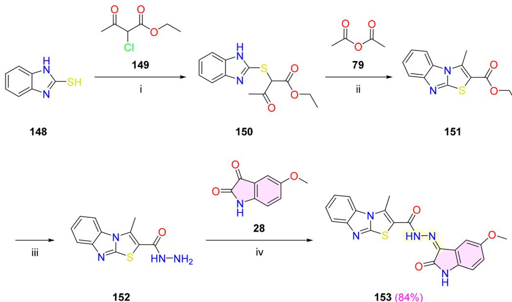
**Scheme 26** Synthesis of isatin–hydrazone hybrid **153**. Reagents and conditions: (i) EtOH, TEA, reflux, 6 h; (ii) reflux, 5 h; (iii)  $\text{N}_2\text{H}_4 \cdot \text{H}_2\text{O}$ , iPrOH, reflux, 6 h; (iv) *gl.* AcOH, reflux, 3–5 h.
