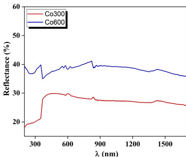
Fig. 7 Reflectance spectra of the compound  $\text{Co}_{0.33}\text{Mn}_{0.33}\text{Fe}_{2.33}\text{O}_4$  annealed at 300 °C and 600 °C at room temperature in the wavelength range between 200 and 1700 nm.
