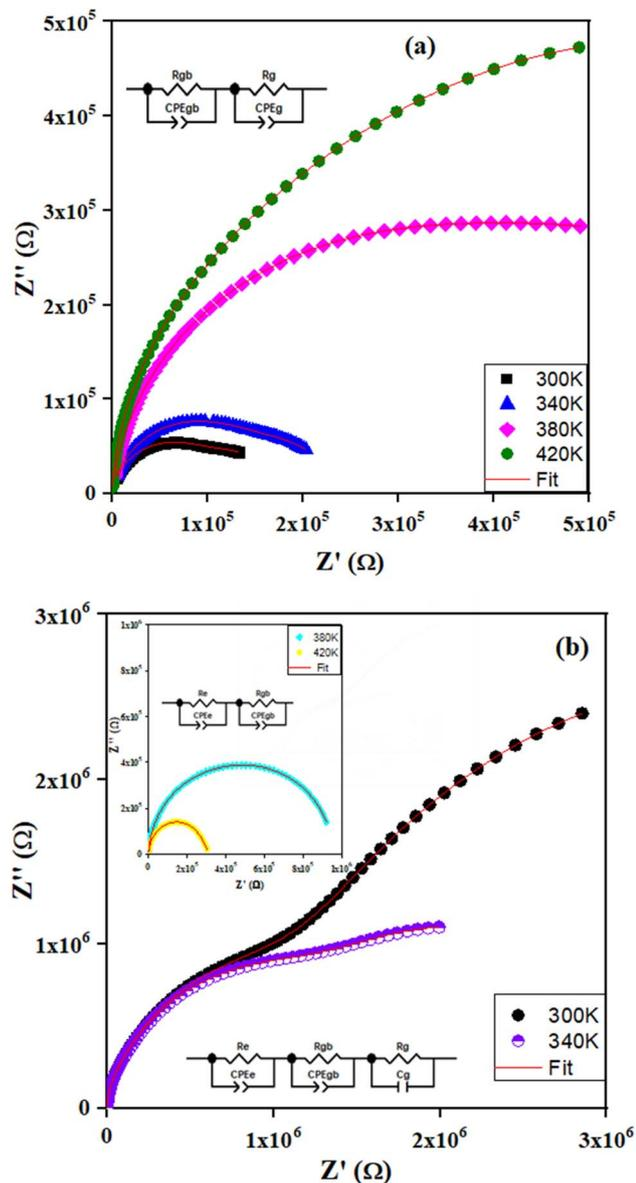
Fig. 13 Nyquist diagram and associated electrical circuits for samples Co300 (a) and Co600 (b).
