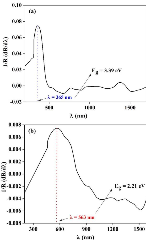
Fig. 9 Variation of the first derivative of reflectance ( $\frac{dR}{d\lambda}$ ) as a function of wavelength ( $\lambda$ ) of  $\text{Co}_{0.33}\text{Mn}_{0.33}\text{Fe}_{2.33}\text{O}_4$  annealed at 300 °C (a) and 600 °C (b).
