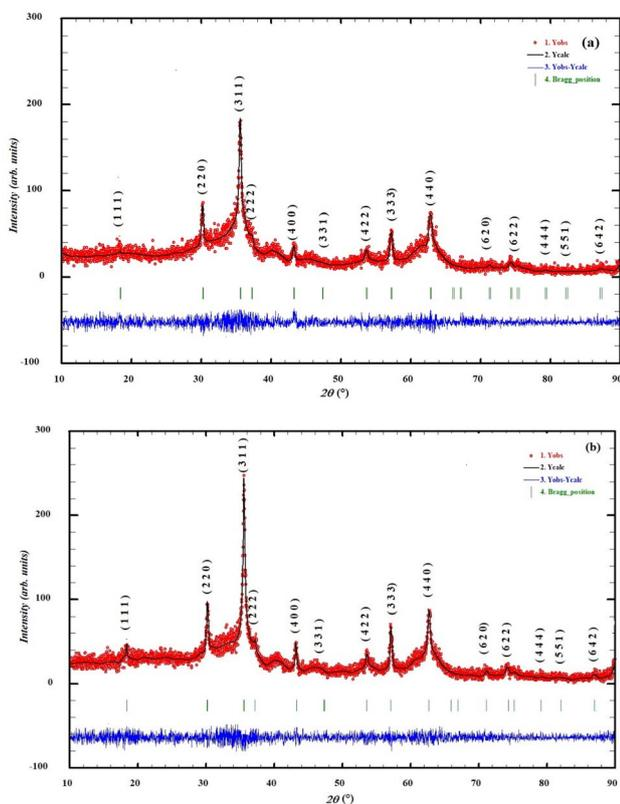
**Fig. 1** Refined XRD patterns of  $\text{Co}_{0.33}\text{Mn}_{0.33}\text{Fe}_{2.33}\text{O}_4$  annealed at 300 °C (a) and 600 °C (b) at room temperature. The red dotted line stands for the experimental data. The calculated data are represented by a black continuous line. The curve in blue shows the difference between the experimental and calculated patterns. The vertical bars in green indicate the Bragg positions.
