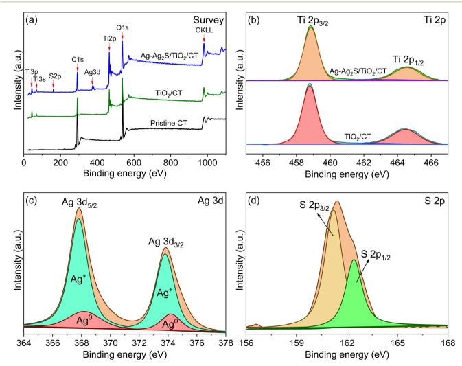
Fig. 4 (a) XPS survey spectra of pristine CT, TiO<sub>2</sub>/CT, and Ag-Ag<sub>2</sub>S/TiO<sub>2</sub>/CT; (b-d) high-resolution XPS spectra: (b) Ti 2p, (c) Ag 3d, and (d) S 2p.
