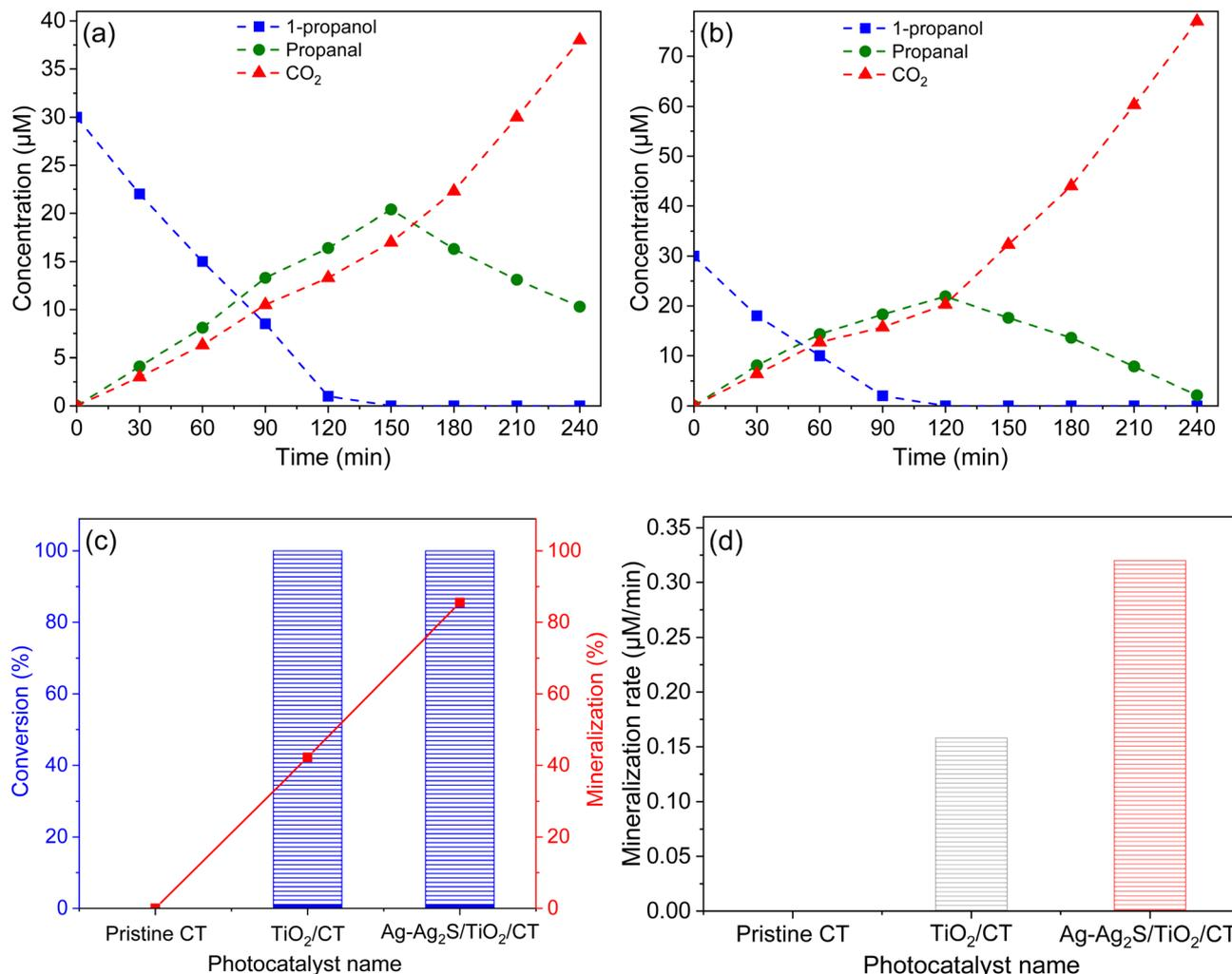
Fig. 7 Photodegradation curves of 1-propanol and the production of CO<sub>2</sub> and propanal vs. irradiation time via TiO<sub>2</sub>/CT (a) and Ag-Ag<sub>2</sub>S/TiO<sub>2</sub>/CT (b). The mineralization and conversion ratio of 1-propanol (c), and the mineralization rate of 1-propanol (d).
