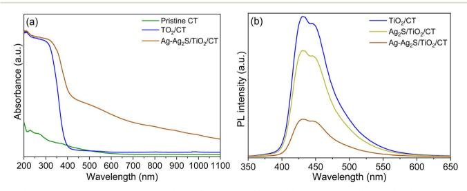
Fig. 5 (a) UV-Vis-NIR absorption spectra of pristine CT,  $TiO_2/CT$ , and  $Ag-Ag_2S/TiO_2/CT$ ; (b) PL spectra of  $TiO_2/CT$ ,  $Ag_2S/TiO_2/CT$ , and  $Ag-Ag_2S/TiO_2/CT$ .
