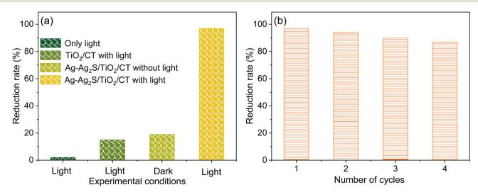
(a) Photocatalytic disinfection of E. coli with and without light for 1 h; (b) the reusability of Ag-Ag<sub>2</sub>S/TiO<sub>2</sub>/CT for the inactivation of E. coli.
