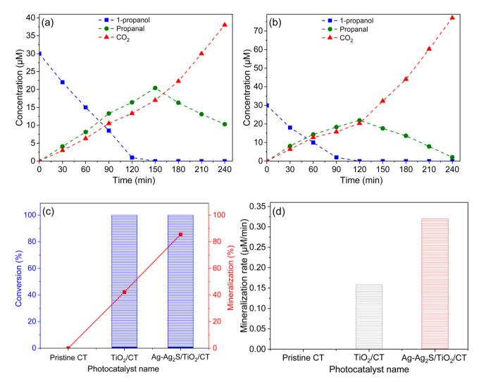
Fig. 7 Photodegradation curves of 1-propanol and the production of  $CO_2$  and propanal vs. irradiation time via  $TiO_2/CT$  (a) and  $Ag-Ag_2S/TiO_2/CT$  (b). The mineralization and conversion ratio of 1-propanol (c), and the mineralization rate of 1-propanol (d).
