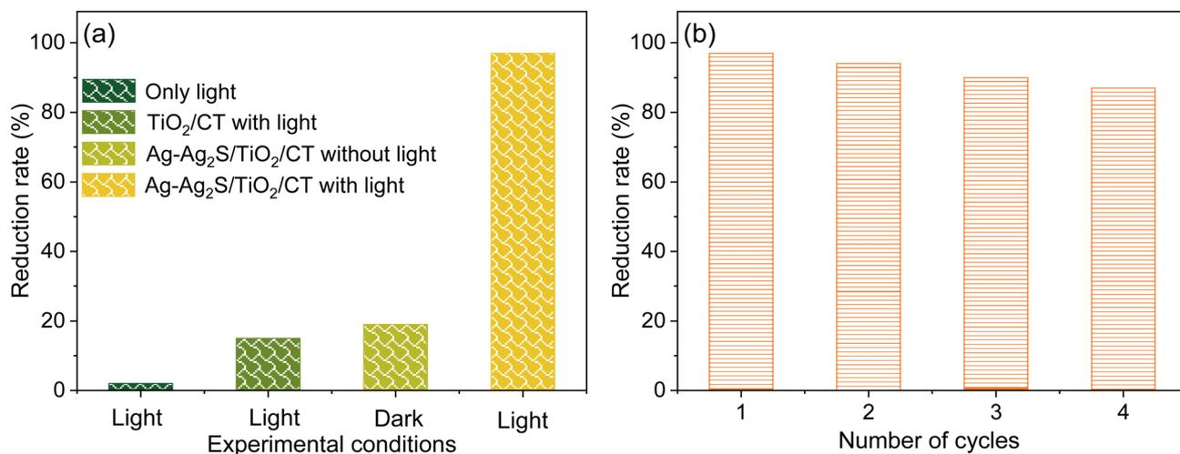
Fig. 8 (a) Photocatalytic disinfection of *E. coli* with and without light for 1 h; (b) the reusability of Ag-Ag<sub>2</sub>S/TiO<sub>2</sub>/CT for the inactivation of *E. coli*.
