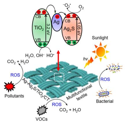
Scheme 1 Proposed photocatalytic mechanism of Ag-Ag<sub>2</sub>S/TiO<sub>2</sub>/CT under sunlight.
