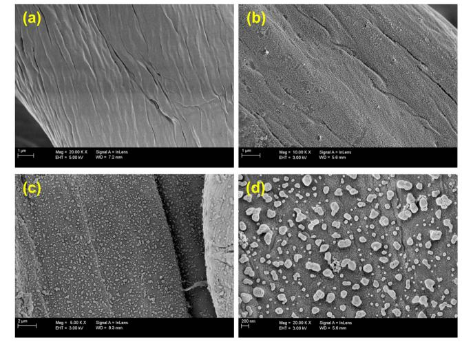
Fig. 3 FE-SEM images of pristine CT (a), TiO<sub>2</sub>/CT (b), and Ag-Ag<sub>2</sub>S/TiO<sub>2</sub>/CT (c and d).
