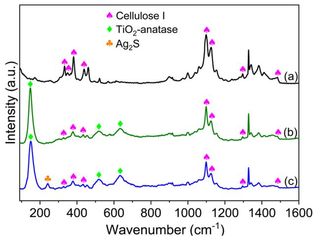
Fig. 2 Raman spectra of pristine CT (a), TiO<sub>2</sub>/CT (b), and Ag-Ag<sub>2</sub>S/TiO<sub>2</sub>/CT (c).
