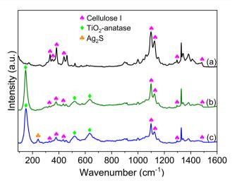
Fig. 2 Raman spectra of pristine CT (a), TiO<sub>2</sub>/CT (b), and Ag-Ag<sub>2</sub>S/ TiO2/CT (c).
