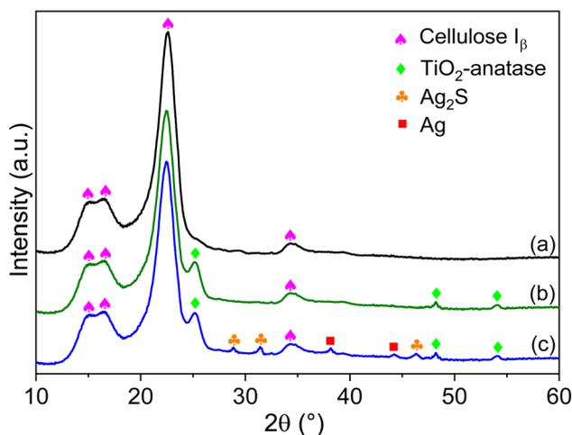
Fig. 1 X-ray diffractogram of pristine CT (a), TiO<sub>2</sub>/CT (b), and Ag-Ag<sub>2</sub>S/TiO<sub>2</sub>/CT (c).
