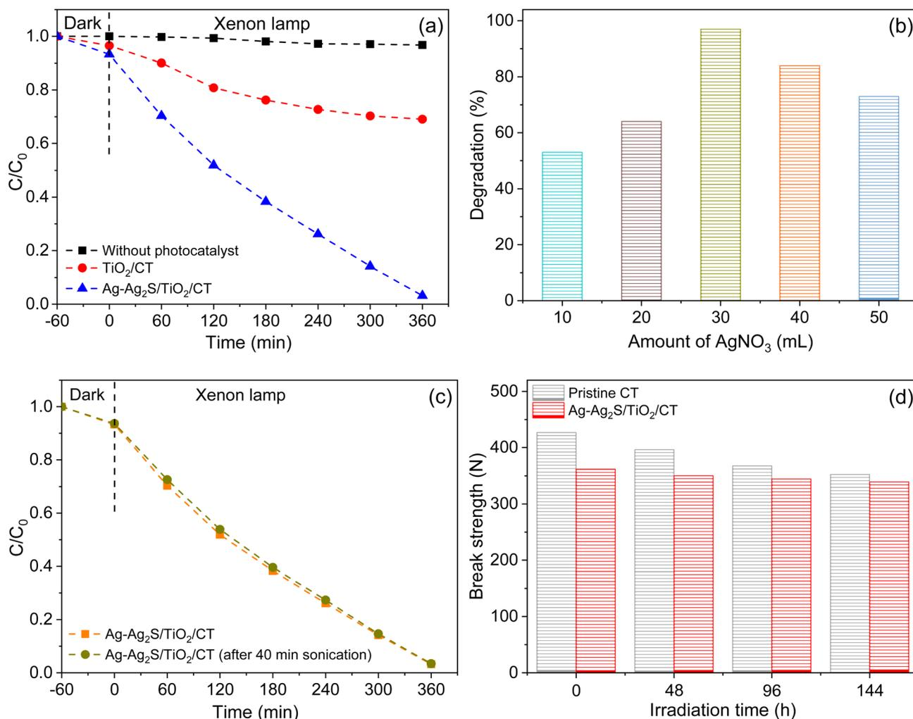
Fig. 6 (a) TOD degradation curves; (b) the effect of the amount of AgNO<sub>3</sub> solution as a precursor of Ag-Ag<sub>2</sub>S on the degradation of TOD; (c) evaluation of TOD concentration in the presence of Ag-Ag<sub>2</sub>S/ $\text{TiO}_2/\text{CT}$  with and without sonication for 40 min; (d) break strength of the pristine textile and Ag-Ag<sub>2</sub>S/ $\text{TiO}_2/\text{CT}$  with and without irradiation.
