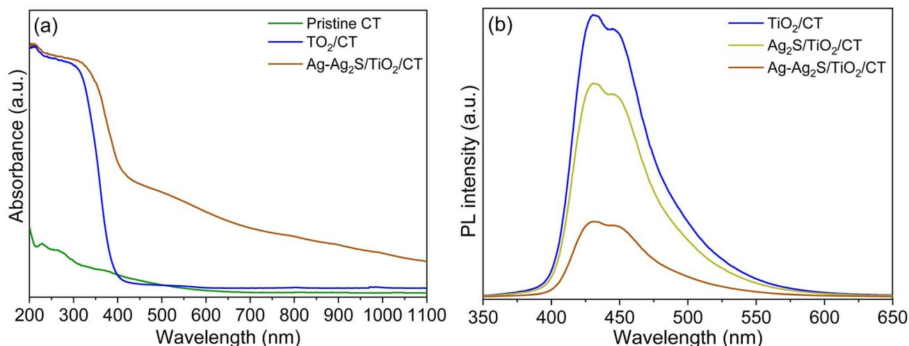
Fig. 5 (a) UV-Vis-NIR absorption spectra of pristine CT,  $\text{TiO}_2/\text{CT}$ , and Ag- $\text{Ag}_2\text{S}/\text{TiO}_2/\text{CT}$ ; (b) PL spectra of  $\text{TiO}_2/\text{CT}$ ,  $\text{Ag}_2\text{S}/\text{TiO}_2/\text{CT}$ , and Ag- $\text{Ag}_2\text{S}/\text{TiO}_2/\text{CT}$ .
