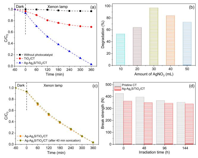
Fig. 6 (a) TOD degradation curves; (b) the effect of the amount of  $AgNO_3$  solution as a precursor of  $Ag-Ag_2S$  on the degradation of TOD; (c) evaluation of TOD concentration in the presence of  $Ag-Ag_2S/TiO_2/CT$  with and without sonication for 40 min; (d) break strength of the pristine textile and  $Ag-Ag_2S/TiO_2/CT$  with and without irradiation.
