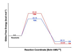
Fig. 3 Gibbs free energy profiles ( $\Delta G$ , expressed in kcal mol<sup>-1</sup>) for each stationary point along the path CN and CX, were assessed with various IEFPCM(1,4-dioxane)/B3LYP-D3/6-311++G(d, p).
