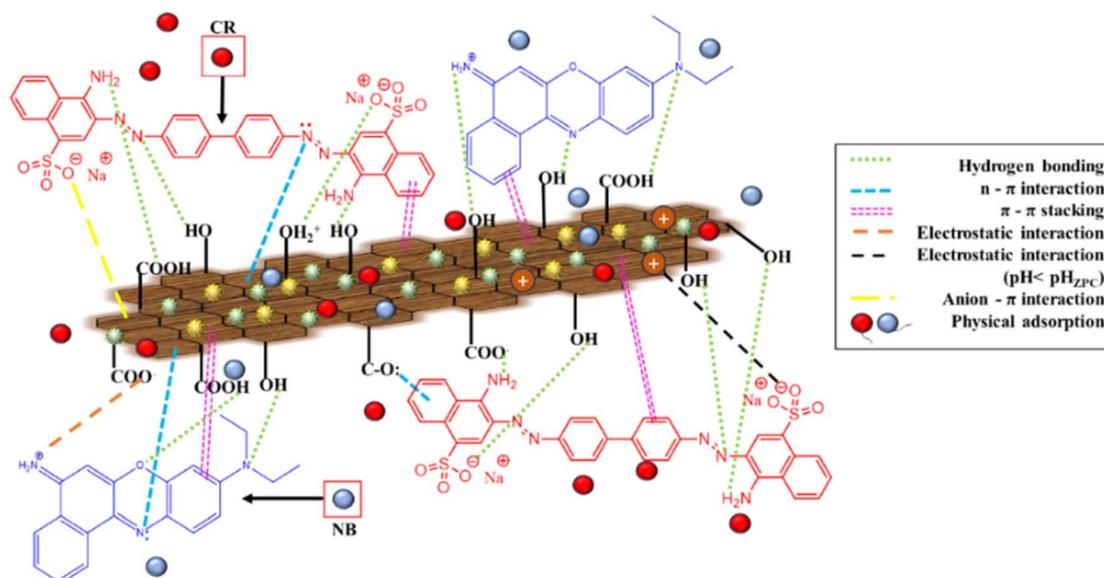
Fig. 7 Plausible mechanism for the adsorption of CR and NB by GG/ $\gamma$ -Fe<sub>2</sub>O<sub>3</sub>.
