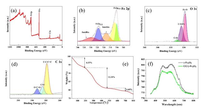
Fig. 5 (a) The full survey scan, and high-resolution spectra of (b) Fe 2p, (c) O 1s, (d) C 1s of  $GG/\gamma$ -Fe<sub>2</sub>O<sub>3</sub>; (e) TGA of  $GG/\gamma$ -Fe<sub>2</sub>O<sub>3</sub>; (f) PL spectra of  $\gamma$ -Fe<sub>2</sub>O<sub>3</sub> and  $GG/\gamma$ -Fe<sub>2</sub>O<sub>3</sub>.
