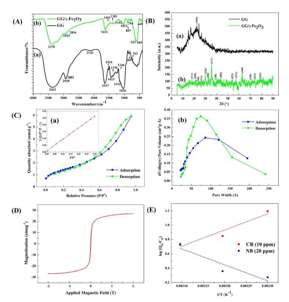
Fig. 1 (A) FT-IR spectra of (a) GG, and (b)  $GG/\gamma$ -Fe<sub>2</sub>O<sub>3</sub>; (B) P-XRD analysis of (a) GG, and (b)  $GG/\gamma$ -Fe<sub>2</sub>O<sub>3</sub>; (C) (a) BET, and (b) BJH curves; (D) M-H magnetization curve of  $GG/\gamma$ -Fe<sub>2</sub>O<sub>3</sub>; (E) Van't Hoff plots.
