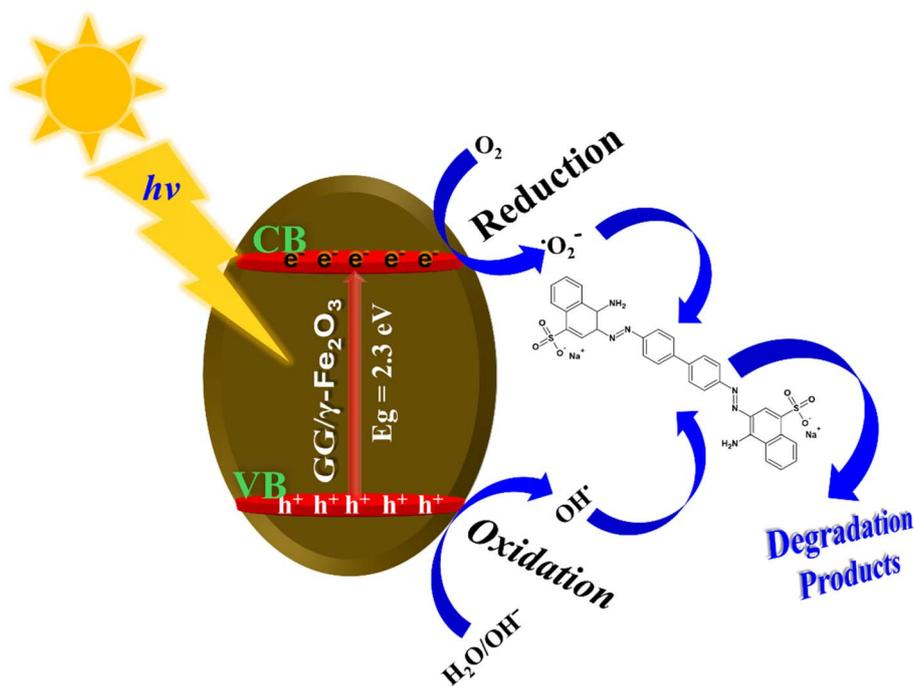
Fig. 8 Proposed mechanism for photodegradation of azo-CR by GG/γ-Fe<sub>2</sub>O<sub>3</sub>.
