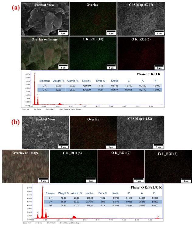
Fig. 3 EDX and mapping of (a) GG and (b)  $GG/\gamma$ -Fe<sub>2</sub>O<sub>3</sub>.
