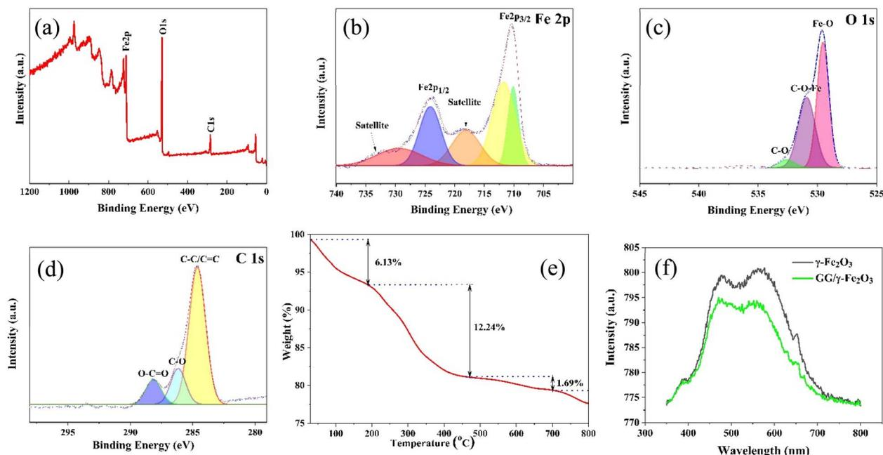
Fig. 5 (a) The full survey scan, and high-resolution spectra of (b) Fe 2p, (c) O 1s, (d) C 1s of GG/ $\gamma$ -Fe<sub>2</sub>O<sub>3</sub>; (e) TGA of GG/ $\gamma$ -Fe<sub>2</sub>O<sub>3</sub>; (f) PL spectra of  $\gamma$ -Fe<sub>2</sub>O<sub>3</sub> and GG/ $\gamma$ -Fe<sub>2</sub>O<sub>3</sub>.
