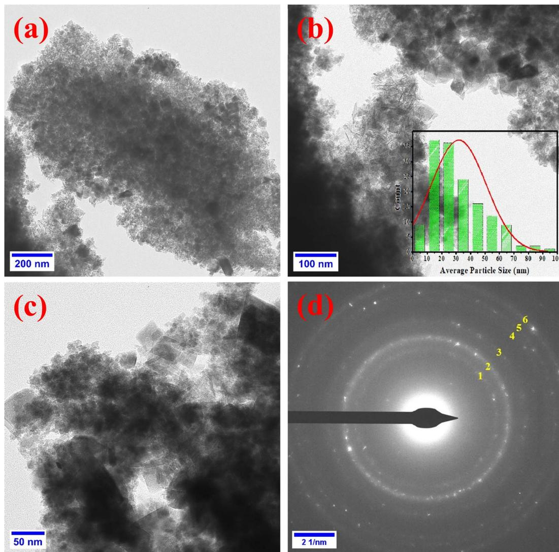
Fig. 4 (a)–(c) represent TEM images, and (d) the SAED ring pattern of GG/ $\gamma$ -Fe<sub>2</sub>O<sub>3</sub>.
