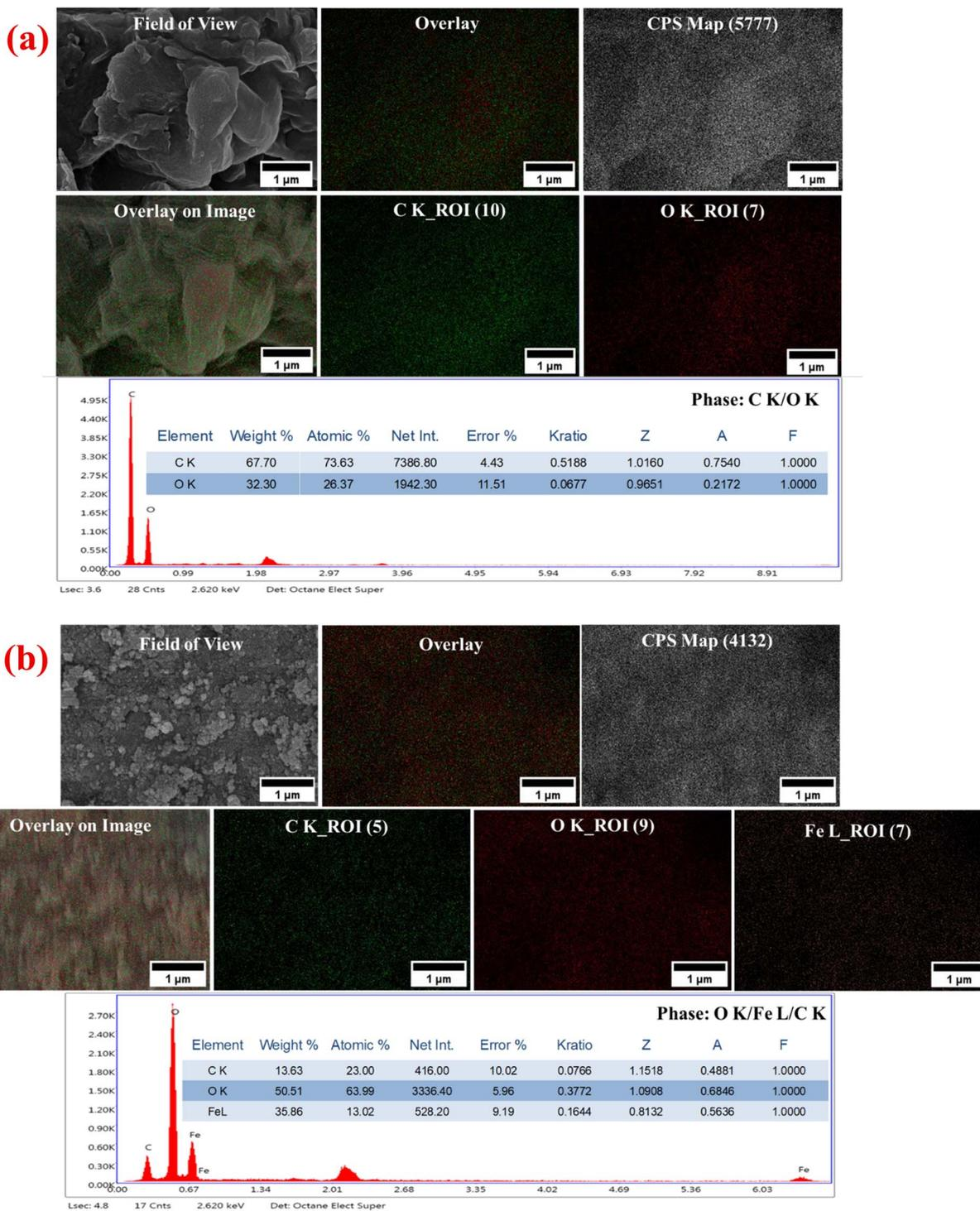
Fig. 3 EDX and mapping of (a) GG and (b) GG/ $\gamma$ -Fe<sub>2</sub>O<sub>3</sub>.
