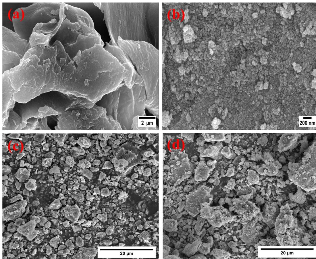
Fig. 2 FE-SEM images of (a) GG, (b) GG/ $\gamma$ -Fe<sub>2</sub>O<sub>3</sub>, (c) GG/ $\gamma$ -Fe<sub>2</sub>O<sub>3</sub> before adsorption, and (d) GG/ $\gamma$ -Fe<sub>2</sub>O<sub>3</sub>@CR.
