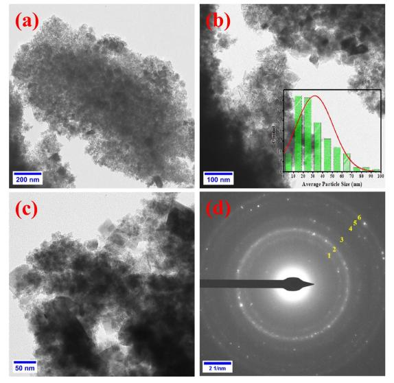
(a)–(c) represent TEM images, and (d) the SAED ring pattern of  $GG/\gamma$ -Fe<sub>2</sub>O<sub>3</sub>.
