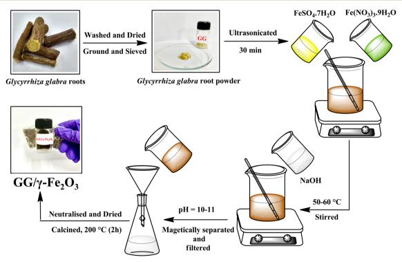
Scheme 1 Stepwise depiction of the synthesis of  $GG/\gamma$ -Fe<sub>2</sub>O<sub>3</sub> nanocomposite.
