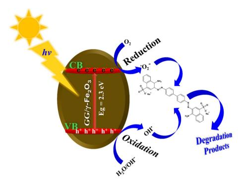
Fig. 8 Proposed mechanism for photodegradation of azo-CR by GG/γ-Fe<sub>2</sub>O<sub>3</sub>
