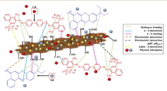
Fig. 7 Plausible mechanism for the adsorption of CR and NB by  $GG/\gamma$ -Fe<sub>2</sub>O<sub>3</sub>.
