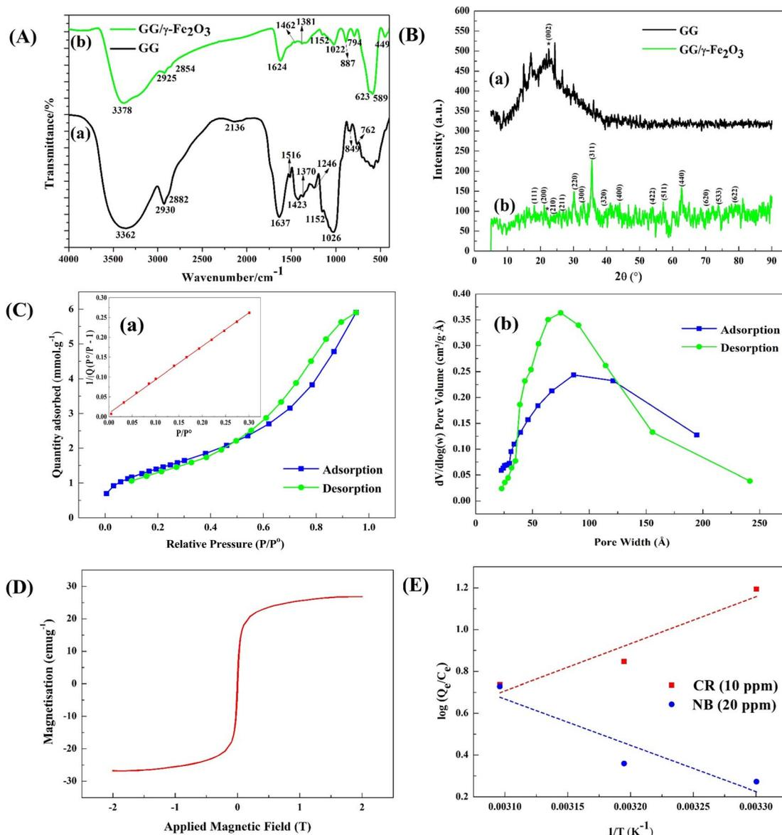
Fig. 1 (A) FT-IR spectra of (a) GG, and (b) GG/γ-Fe<sub>2</sub>O<sub>3</sub>; (B) P-XRD analysis of (a) GG, and (b) GG/γ-Fe<sub>2</sub>O<sub>3</sub>; (C) (a) BET, and (b) BJH curves; (D) *M*–*H* magnetization curve of GG/γ-Fe<sub>2</sub>O<sub>3</sub>; (E) Van't Hoff plots.
