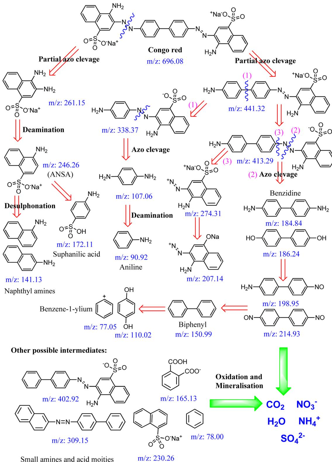
Scheme 2 Proposed degradation pathways of CR by GG/ $\gamma$ -Fe<sub>2</sub>O<sub>3</sub>.
