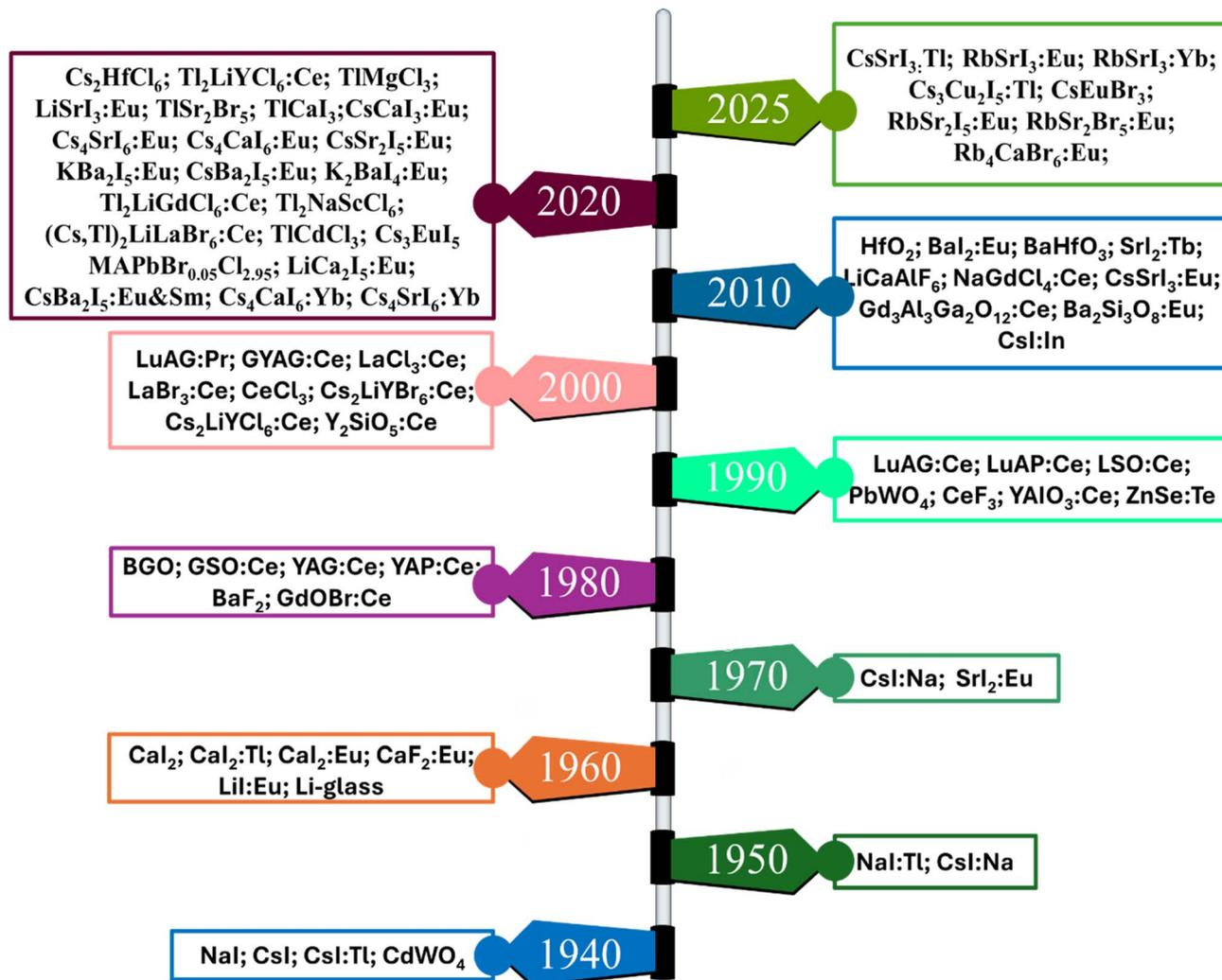
Fig. 1 Timeline of the discovery of various scintillators.<sup>4,9–13</sup>
