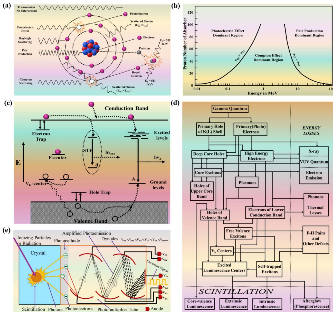
Fig. 4 (a) Graphical representation of light-matter interaction. (b) Probability of the occurrence of PE, CE and PP, depending on the incident radiation's energy and proton number of the absorber<sup>121</sup>. (c) Depiction of energy band scheme of the scintillation process.<sup>91</sup> (d) Flowchart of the scintillation in an inorganic scintillator.<sup>91</sup> (e) Schematic diagram of a high energy radiation detection procedure through scintillation.
