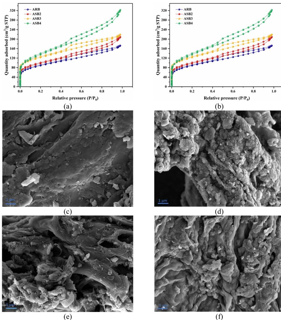
Fig. 1 (a) N<sub>2</sub> adsorption–desorption isotherms of biochar materials at 77 K, (b) the pore size distributions of biochar materials based on nonlocal density functional theory (NLDFT), SEM images of prepared biochars (c) ARB, (d) ASB2, (e) ASB3, (f) ASB4.
