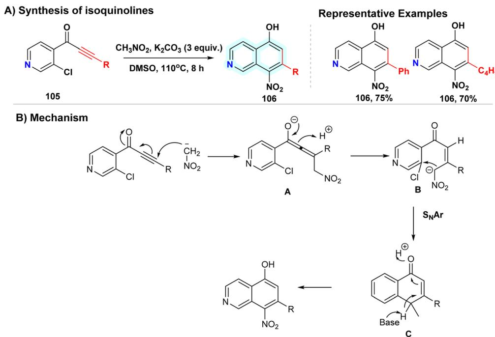
Scheme 35 Synthesis of 5-OH-8-NO<sub>2</sub>- isoquinolines by Beesu *et al.*<sup>106</sup>
