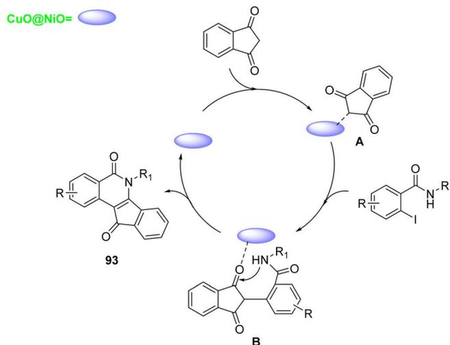
Scheme 29 Synthesis of fused isoquinolinone scaffold by Rawat *et al.*<sup>95</sup>
