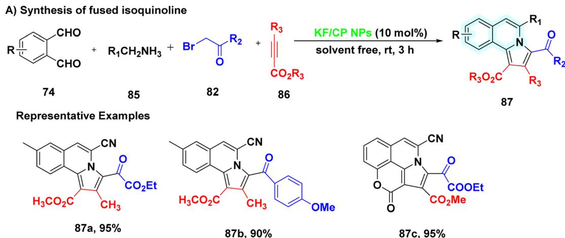
Scheme 27 Synthesis of pyrrolo-fused isoquinolines by S. Amiri *et al.*<sup>93</sup>
