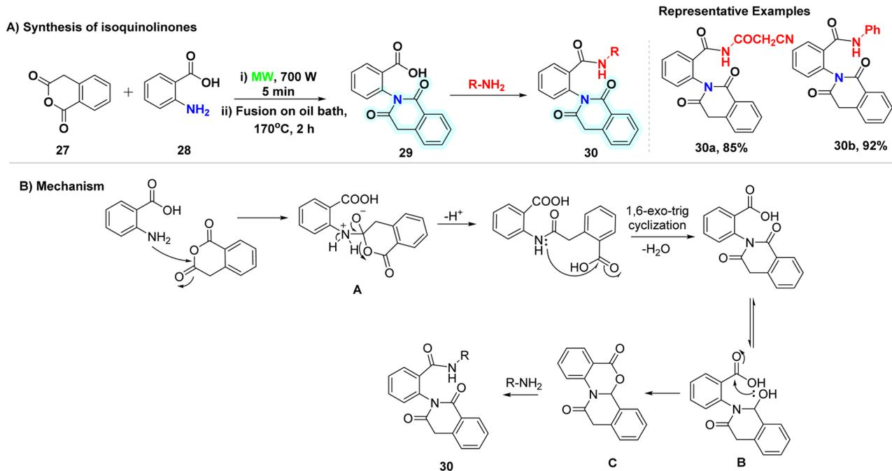
Scheme 10 Synthesis of isoquinolinones by Hekal *et al.*<sup>65</sup>
