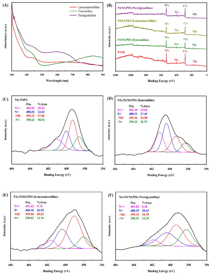
Fig. 2 (A) UV-VIS spectra of PANI : PSS with various structures; (B) XPS survey scans of PANI and PANI : PSS with various structures; and high-resolution XPS N 1s spectra of (C) PANI, (D) PANI : PSS (emeraldine), (E) PANI : PSS (leucoemeraldine), and (F) PANI : PSS (pernigraniline).
