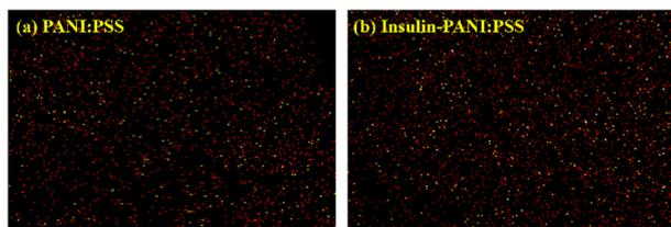
Fig. 6 EDX mapping of the N element: (a) PANI : PSS and (b) insulin-PANI : PSS.
