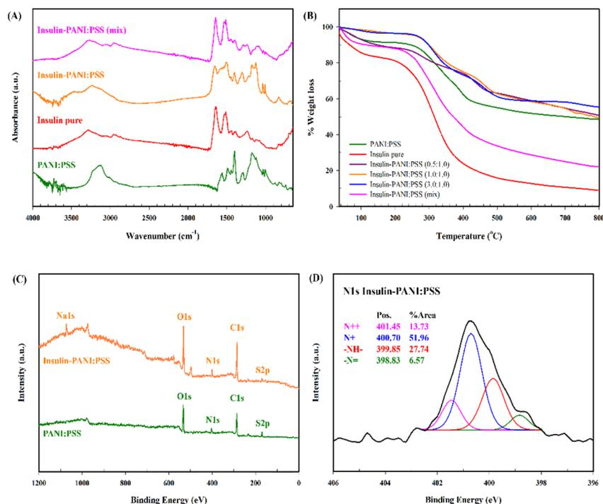
Fig. 5 Characterization of insulin-PANI : PSS: (A) FTIR spectra, (B) thermograms, (C) XPS survey scans, and (D) N 1s spectrum of insulin-PANI : PSS.
