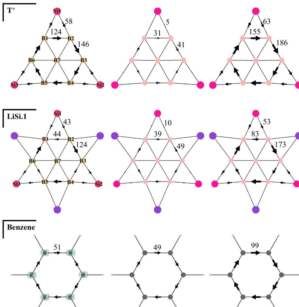
Fig. 6 Bond current strengths of  $T^+$  (top),  $LiSi.1$  (middle) and benzene (bottom) from  $\sigma$  electron contribution (left),  $\pi$  electron contribution (center), and all electrons (right). Each arrow represents the percentage relationship with respect to the diatropic benzene current strength of  $12 \text{ nA T}^{-1}$ .
