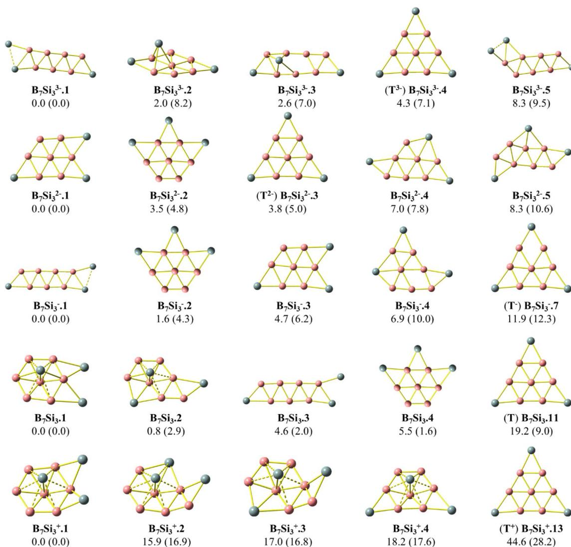
Fig. 1 Optimized geometries of the  $B_7Si_3^q$  cluster ( $q = +, 0, -, 2-,$  and  $3-$ ) obtained at the PBE/6-311+G(d) level. Relative energies ( $\text{kcal mol}^{-1}$ ) were calculated using (U)CCSD(T)/aug-cc-pVTZ//PBE/6-311+G(d), with values from PBE/6-311+G(d) given in parentheses. All energies include zero-point energy (ZPE) corrections evaluated at the PBE/6-311+G(d) level.
