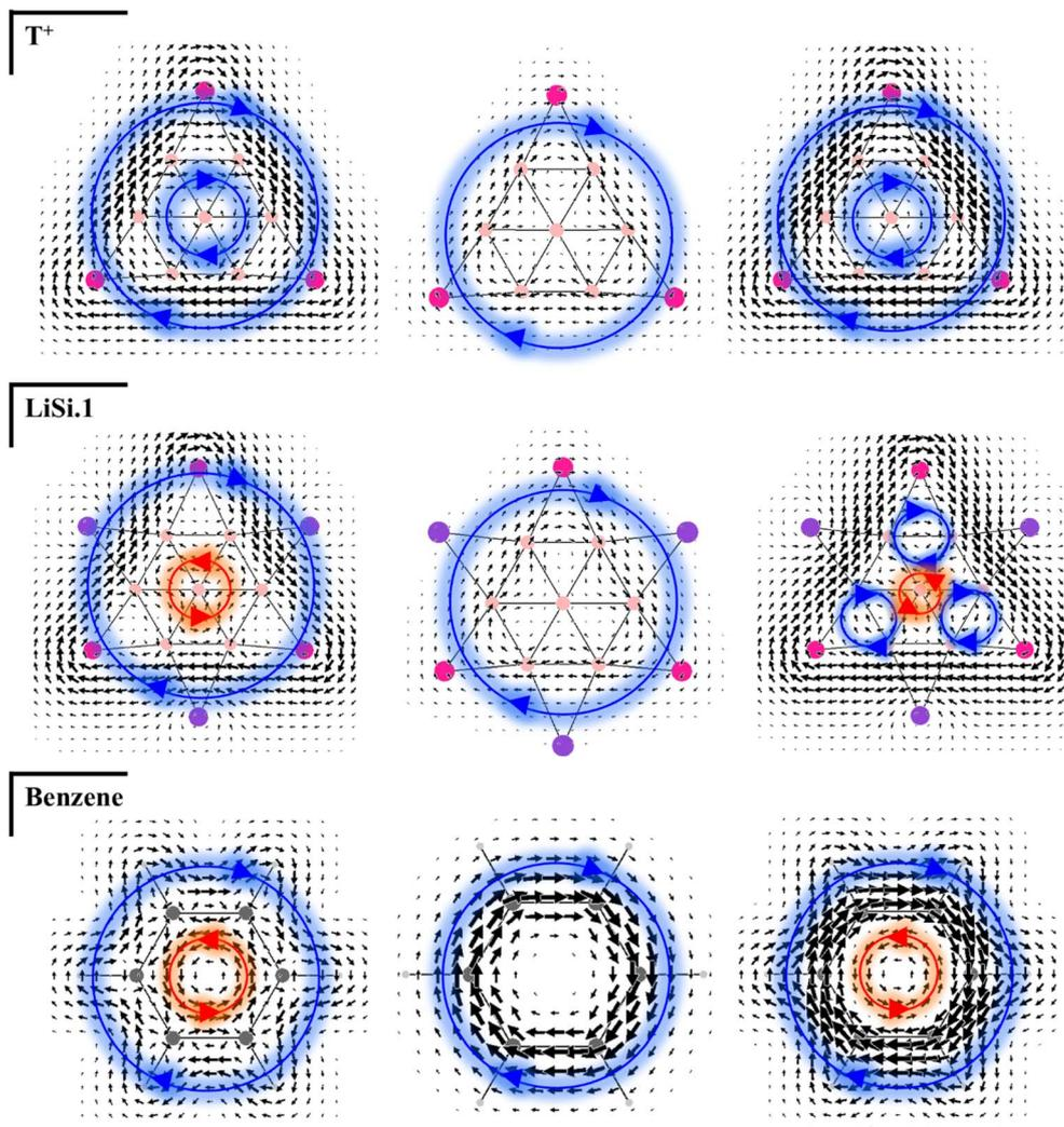
Fig. 5 Magnetic current density maps of  $T^+$  (top),  $LiSi.1$  (middle) and benzene (bottom) from  $\sigma$ -electron contribution (left),  $\pi$ -electron contribution (center), and all-electron contribution (right) at 1 Bohr above the molecular planes. Diatropic and paratropic domains are marked by green and red rings, respectively.
