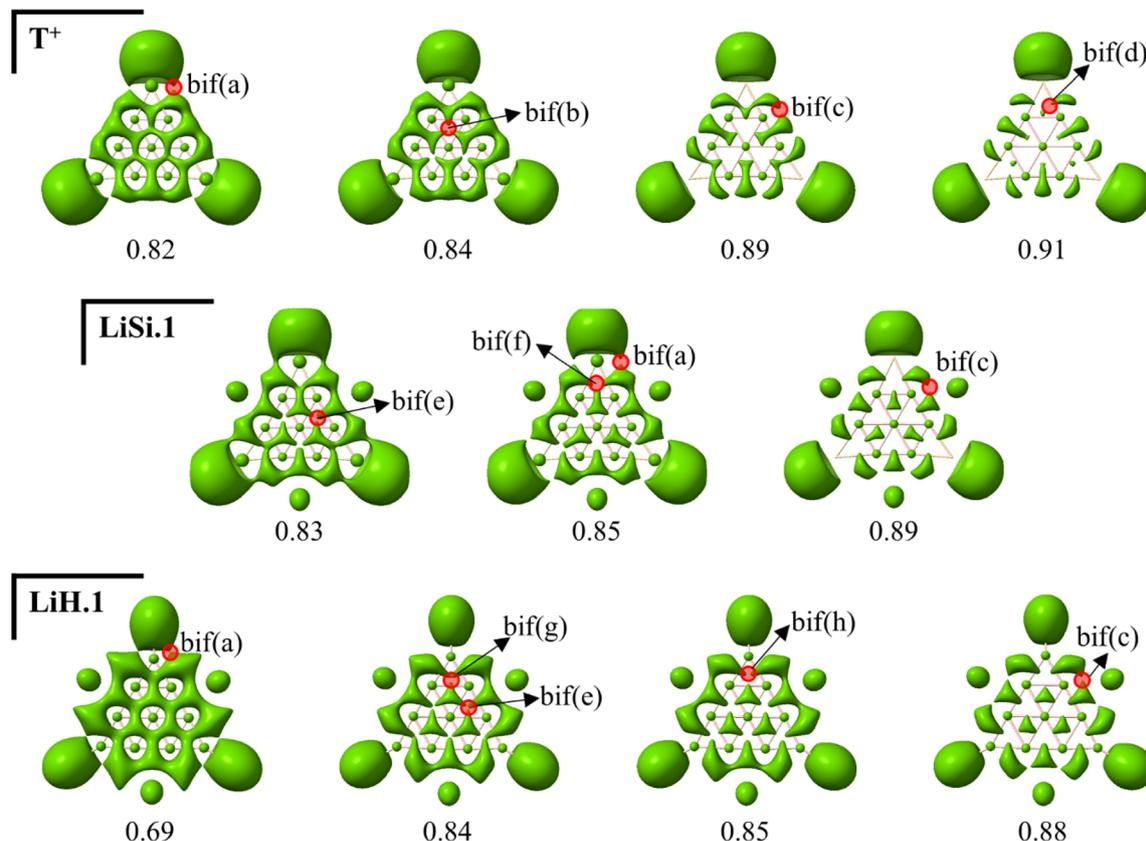
Fig. 8 Electron localization function  $ELF_{\sigma}$  maps of  $T^+$  (top),  $LiSi.1$  (middle), and  $LiH.1$  (bottom) at different isosurface values. Red circles (with the label from bif(a) to bif(h)) indicate the positions of bifurcations corresponding to each isosurface value.
