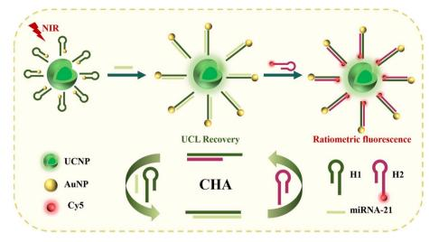
Scheme 1 Schematic diagram of a fluorescence sensor for measuring miRNA-21
