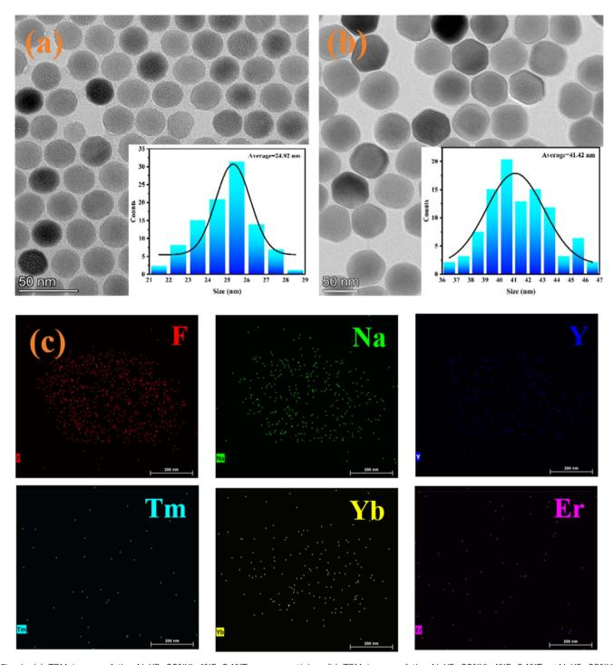
Fig. 1 (a) TEM image of the NaYF<sub>4</sub>:20%Yb,4%Er,0.1%Tm nanoparticles; (b) TEM image of the NaYF<sub>4</sub>:20%Yb,4%Er,0.1%Tm@NaYF<sub>4</sub>:20%Yb nanoparticles; (c) EDS images of the NaYF<sub>4</sub>:20%Yb,4%Er,0.1%Tm@NaYF<sub>4</sub>:20%Yb nanoparticles.
