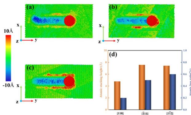
Fig. 2 Surface morphology of the alloy. (a) [110] orientation, (b) [ $\bar{1}\bar{1}\bar{1}$ ] orientation, (c) [ $\bar{1}\bar{1}\bar{2}$ ] orientation, (d) maximum atomic pile-up height and atom loss ratio.
