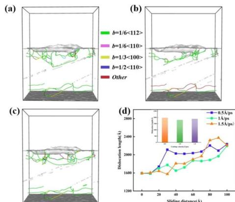
Fig. 7 Dislocation distribution and variation of dislocation line length with sliding distance during steady-state friction of the alloy. (a) 0.5 Å ps<sup>-1</sup>, (b) 1 Å ps<sup>-1</sup>, (c) 1.5 Å ps<sup>-1</sup>, (d) dislocation line length as a function of sliding distance.
