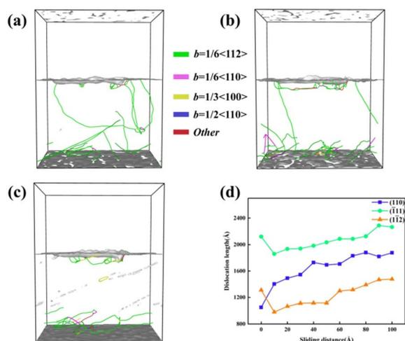
Fig. 3 Dislocation distribution and the variation of dislocation line length with sliding distance for the three crystallographic orientations. (a)  $[110]$  orientation, (b)  $[\bar{1}11]$  orientation, (c)  $[1\bar{1}2]$  orientation, (d) dislocation line length as a function of sliding distance.
