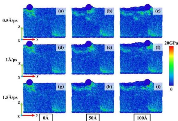
Fig. 8 Atomic stress distribution maps. (a–c) Sliding velocity of 0.5 Å ps<sup>-1</sup>, (d–f) sliding velocity of 1 Å ps<sup>-1</sup>, (g–i) sliding velocity of 1.5 Å ps<sup>-1</sup>.
