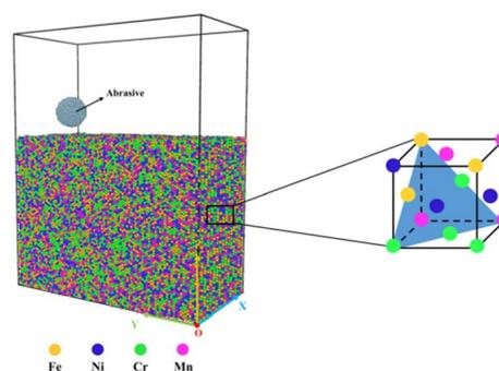
Fig. 1 Model of the FeNiCrMn high-entropy alloy.
