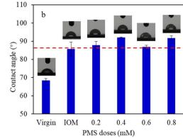
Fig. 7 Variation in functional groups (a) and contact angles (b) on the clean and fouled membrane surfaces using ATR-FTIR and contact angle measurements.
