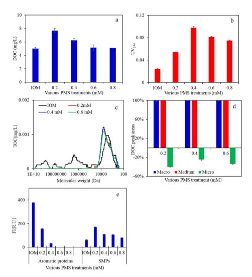
Fig. 4 Organic content, MW distribution and fluorescent organic properties of IOM by various heat-activated PMS treatments: (a) DOC content, (b) UV<sub>254</sub> content, (c) MW distribution, (d) peak area rejection, and (e) FI.
