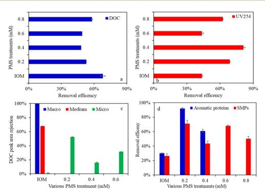
Fig. 5 Organic rejection of IOM by UF after various heat-activated PMS treatments, (a) DOC, (b) UV<sub>254</sub>, (c) peak areas of molecular organics, (d) fluorescent organics.
