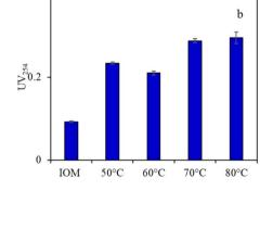
Fig. 2 Organic removal of IOM under various activation temperatures by PMS (IOM DOC = 3 mg  $L^{-1}$ , PMS = 0.4 mM, 60 min): (a) DOC content, (b)  $UV_{254}$  content, and (c) FI.
