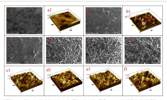
Fig. 6 SEM and AFM images of clean and fouled membranes by IOM under various PMS treatment: (a, a1) Virgin; (b, b1) IOM under control; (c, c1) PMS 0.2 mM; (d, d1) PMS 0.4 mM; (e, e1) PMS 0.6 mM; and (f, f1) PMS 0.8 mM.
