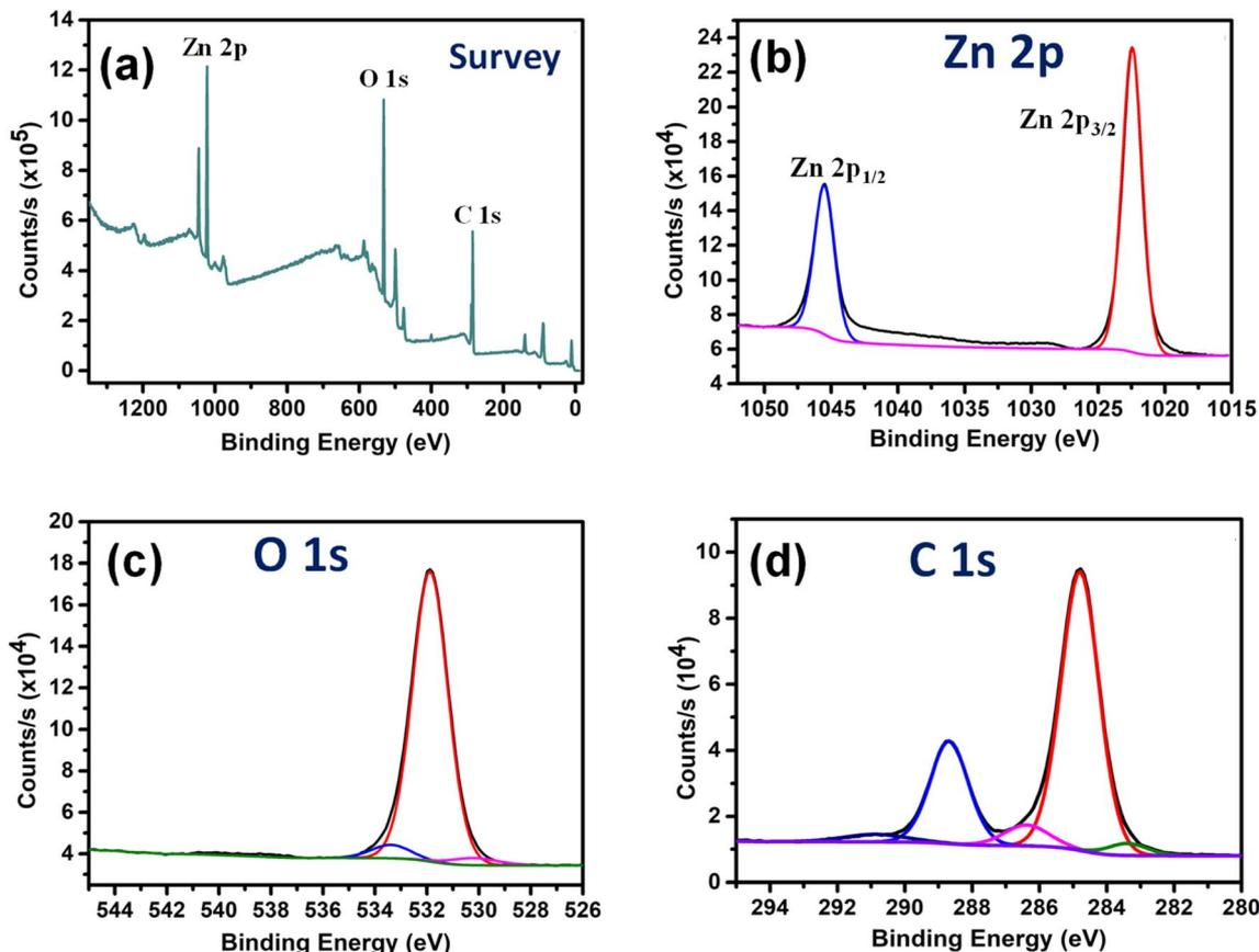
Fig. 4 XPS analysis of Zn-BTC MOF: (a) survey spectra; high resolution spectra of (b) Zn 2p, (c) O 1s and (d) C 1s.
