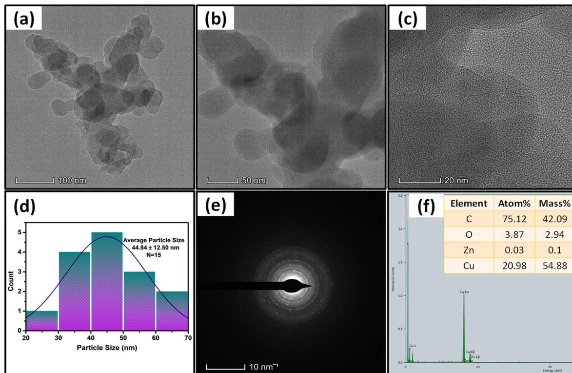
Fig. 3 (a)–(c) TEM images, (d) particle size distribution histogram, (e) SAED pattern, and (f) EDS spectrum with elemental composition.
