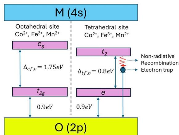
Fig. 8 Schematic of the proposed energy band structure for  $\text{MFe}_2\text{O}_4$  ( $\text{M} = \text{Co}, \text{Mn}$ ) nanoparticles. The diagram is constructed based on UV-vis absorption, PL spectra, and Urbach tail analysis. This diagram elucidates the correlation among crystal field environments, cation distribution, and optical transitions in spinel ferrites.
