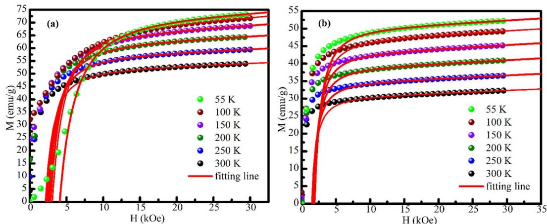
Fig. 11 Experimental and fitted magnetization curves of (a)  $\text{CoFe}_2\text{O}_4$  and (b)  $\text{MnFe}_2\text{O}_4$  nanoparticles at selected temperatures based on the law of approach to saturation (LAS). The solid dots represent experimental  $M$ - $H$  data, and the solid lines denote the best-fit curves obtained by minimizing the sum of squared residuals.
