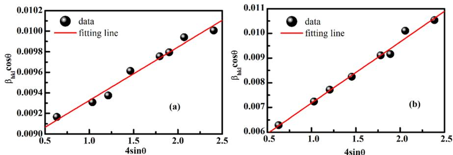
Fig. 2 Williamson–Hall (W–H) plots for (a)  $\text{CoFe}_2\text{O}_4$  and (b)  $\text{MnFe}_2\text{O}_4$  nanoparticles. The red lines represent linear fits to the experimental data based on the W–H equation. The lattice strain was calculated from the slope of the fitted line, while the average crystallite size was determined from the y-intercept.
