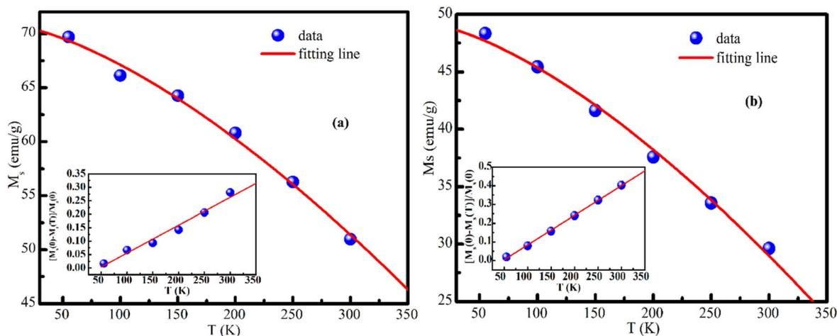
Fig. 12 Temperature dependence of the saturation magnetization for (a)  $\text{CoFe}_2\text{O}_4$  and (b)  $\text{MnFe}_2\text{O}_4$  nanoparticles. The solid red lines indicate the fitting to Bloch's law, as described in the text. Insets show the reduced magnetization,  $[M_s(0) - M_s(T)]/M_s(0)$ , plotted as a function of temperature to highlight the spin-wave excitation behavior.
