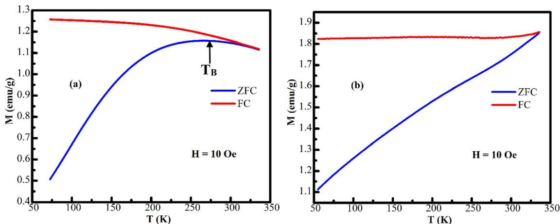
Fig. 14 ZFC and FC magnetization curves of (a)  $\text{CoFe}_2\text{O}_4$  and (b)  $\text{MnFe}_2\text{O}_4$  measured at 10 Oe in the temperature range of 55–350 K. The blocking temperature ( $T_B$ ) for  $\text{CoFe}_2\text{O}_4$  is indicated by a dashed vertical line. For  $\text{MnFe}_2\text{O}_4$ ,  $T_B$  lies above the measurement range, as suggested by the convergence of FC/ZFC curves at high temperatures.
