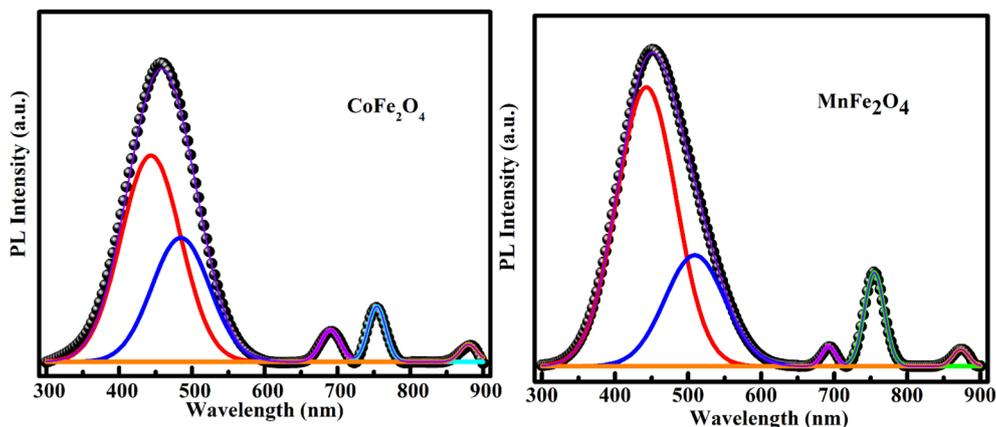
Fig. 7 Deconvolution of the photoluminescence (PL) spectra of  $\text{CoFe}_2\text{O}_4$  and  $\text{MnFe}_2\text{O}_4$  nanoparticles excited at 310 nm. The broad emission peak centred at 458 nm in both samples is resolved into two Gaussian components. In  $\text{CoFe}_2\text{O}_4$ , peaks at 443 nm (2.80 eV) and 485 nm (2.56 eV) are identified, while in  $\text{MnFe}_2\text{O}_4$ , the components appear at 443 nm (2.80 eV) and 509 nm (2.44 eV).
