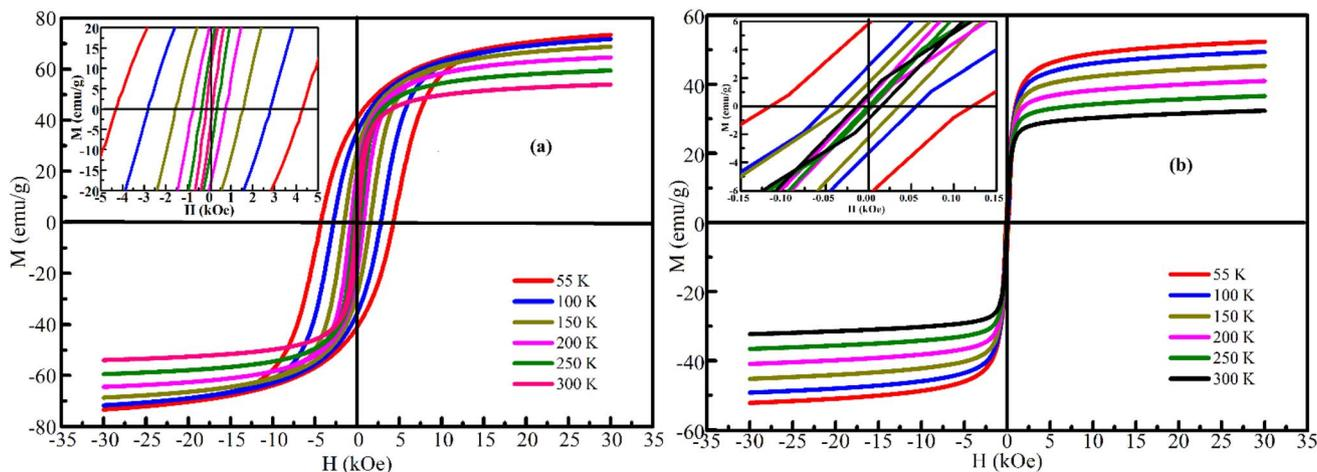
Fig. 10 The typical hysteresis loop of  $\text{CoFe}_2\text{O}_4$  NPs (a) and  $\text{MnFe}_2\text{O}_4$  NPs (b) for different temperatures. The insets are an enlargement of the magnetization at low field.
