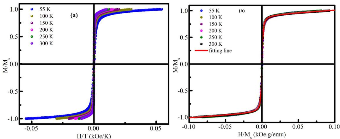
Fig. 15 Relative magnetization ( $M/M_s$ ) of  $\text{MnFe}_2\text{O}_4$  NPs measured at six different temperatures plotted as a function of  $H/T$  (a) and  $H/M_s$  (b), according to the interacting superparamagnetic (ISP) scaling law. The red line in (b) represents the fit using the modified Langevin function, illustrating the presence of dipolar interactions among nanoparticles.
