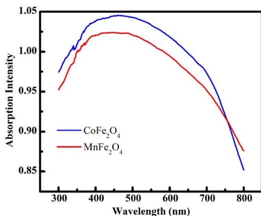
Fig. 5 Optical absorption spectra for the CoFe<sub>2</sub>O<sub>4</sub> and MnFe<sub>2</sub>O<sub>4</sub> nanoparticles.
