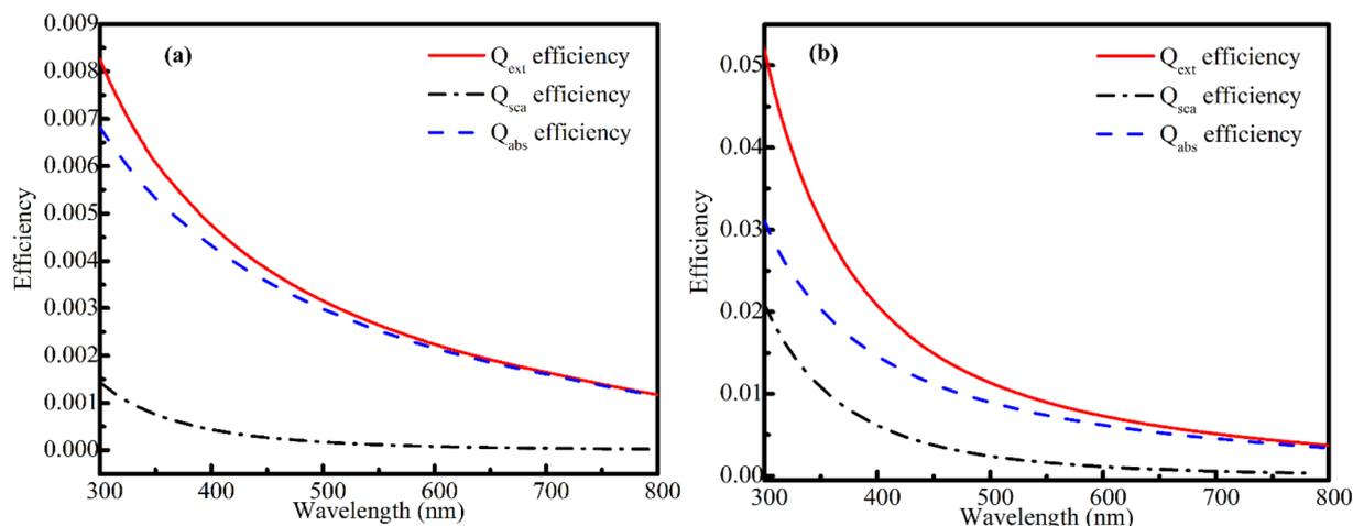
Fig. 9 The wavelength dependence of extinction ( $Q_{\text{ext}}$ ), absorption ( $Q_{\text{abs}}$ ), and scattering ( $Q_{\text{sca}}$ ) efficiencies for (a)  $\text{CoFe}_2\text{O}_4$  NPs and (b)  $\text{MnFe}_2\text{O}_4$  NPs. The parameters are determined from the Mie theory using eqn 4(a)–(c).
