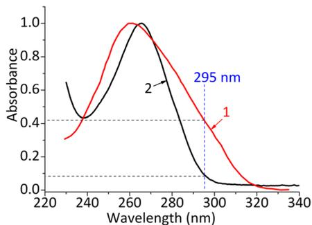
Fig. 1 Normalized absorption spectra of Tel22-G4 (1) and (dT)<sub>15</sub> (2). Oligonucleotide concentration:  $5 \times 10^{-6}$  M in 10 mM sodium cacodylate buffer containing 100 mM NaCl (pH 7.3).
