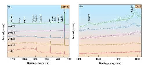
Fig. 2 (a) XPS full spectra of CCO@xZnO and (b) Zn 2p high-resolution spectrum.
