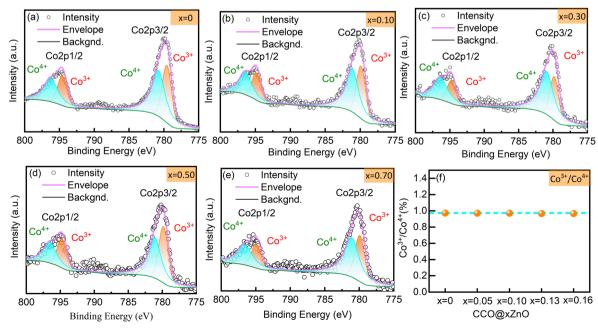
Fig. 3 (a-e) Co ion split peak fitting curves for CCO@xZnO and (f) relative  $Co^{3+}$  and  $Co^{4+}$  contents in the samples.
