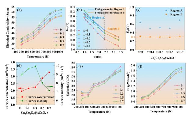
Fig. 6 Plots of (a) conductivity *versus* temperature, (b)  $\ln(T)$  *versus* 1000/T, (c)  $E_{ar}$  (d) carrier concentration and mobility (e) Seebeck coefficient *versus* temperature, and (f) PF *versus* temperature for CCO@xZnO.
