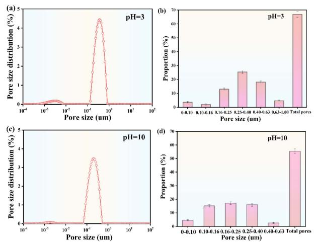
ig. 6 PSD and porosity of aggregates in the filter cake of mixed clay at pH 3 (a) and (b) and pH 10 (c) and (d)
