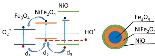
Fig. 8 Zone diagram of developed core-shell nanofibers.
