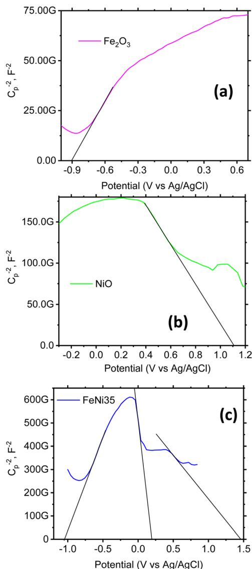
Fig. 9 Mott-Schottky spectra: (a) Fe<sub>2</sub>O<sub>3</sub> nanofibers, (b) NiO nanotubes, and (c) FeNi35.
