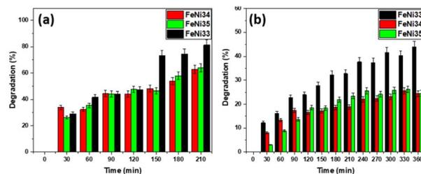
Fig. 7 Visible-light degradation of methylene blue (a) and acetaminophen (b) using FeNi33, FeNi34, and FeNi35 catalysts.
