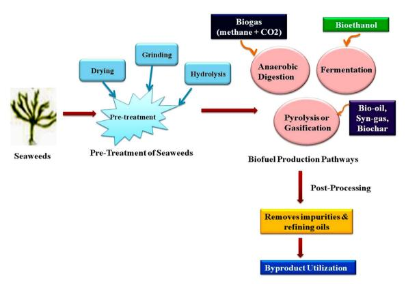
Fig. 4 Biofuel production pathways by seaweeds in biorefinery.
