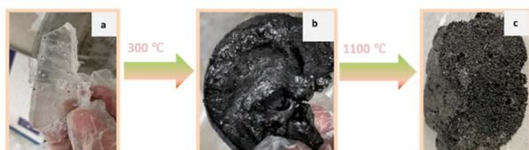
Fig. 5 Pre-carbonization and post-carbonization morphology of sucrose gel.
