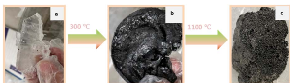
Fig. 5 Pre-carbonization and post-carbonization morphology of sucrose gel.
