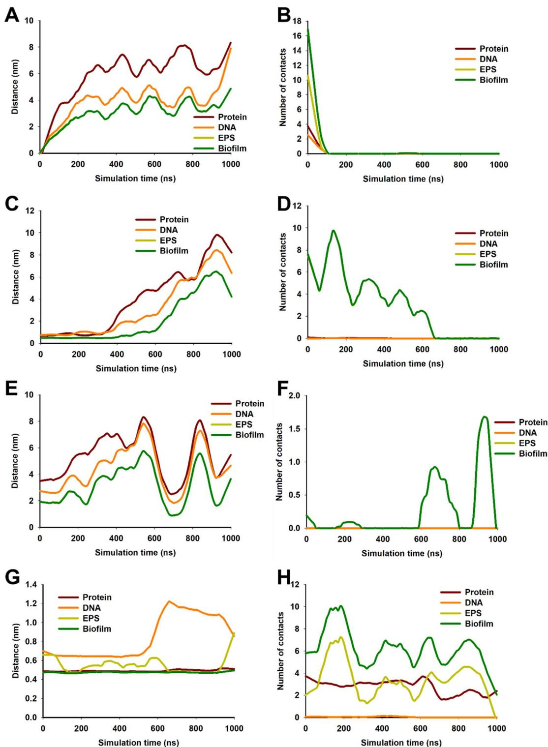
Fig. 10 Interaction of NPs with biofilm and its components (protein, DNA and EPS) with CNT (A and B), Ag (C and D), TiO<sub>2</sub> (E and F), and ZnO NP (G and H). A, C, E and G show distance between biofilm and its components and NPs during 1  $\mu$ s of simulation. B, D, F and H show number of contacts between biofilm and its components and NPs during 1  $\mu$ s of simulation. The line graphs of EPS and biofilm overlap in A to F.
