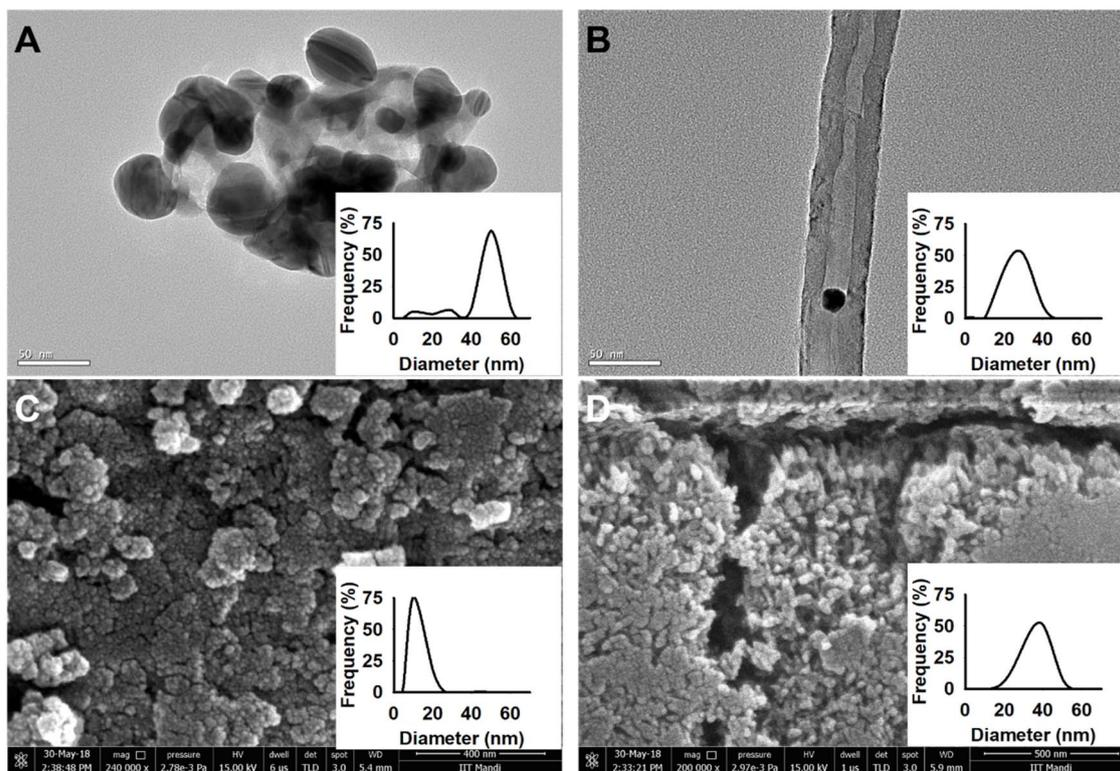
Fig. 1 Electron microscopy of NP used in the study. (A) and (B) show HRTEM images of AgNP and MWCNT (B), respectively. (C) and (D) show SEM images of TiO<sub>2</sub> and ZnO NPs, respectively. Scale bar is 50 nm in (A) and (B), 400 nm in (C) and 500 nm in (D). The inset shows diameter distribution determined from SEM/TEM images for 100–150 NPs except CNT where diameter of 75 CNTs was determined.
