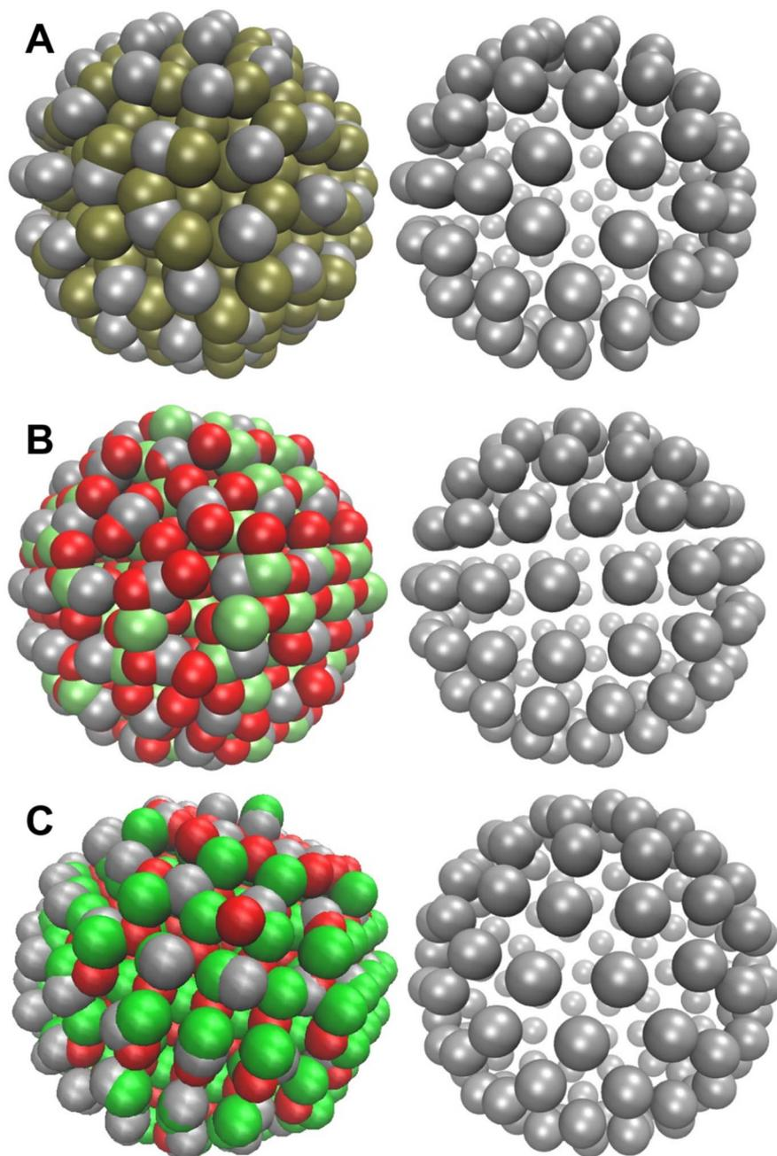
Fig. 2 Models of Ag (A),  $\text{TiO}_2$  (B) and ZnO NPs (C). The left panel shows an overlay of all-atom and CG model while the right panel shows only the CG model. The red and green beads in the left panel represent metal and oxygen atoms, respectively. The silver beads in the left panel show the overlaid CG model shown separately in the right panel. All NPs have a diameter of  $\sim 2.5$  nm.
