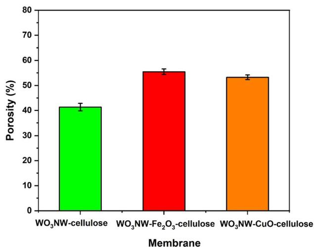
Fig. 2 Effect of Fe<sub>2</sub>O<sub>3</sub> and CuO on the membrane porosity.
