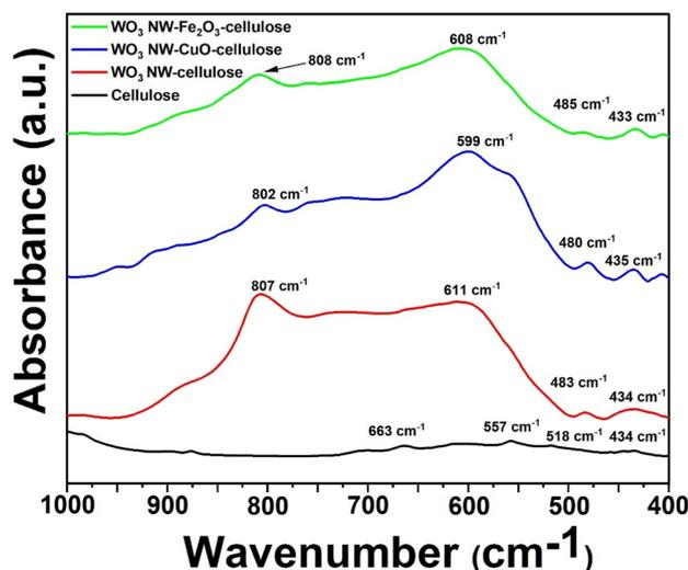
Fig. 4 FT-IR spectra of cellulose (black curve),  $\text{WO}_3$ –cellulose (red curve),  $\text{WO}_3$  NW–CuO–cellulose (blue curve) and  $\text{WO}_3$  NW– $\text{Fe}_2\text{O}_3$ –cellulose (green curve).
