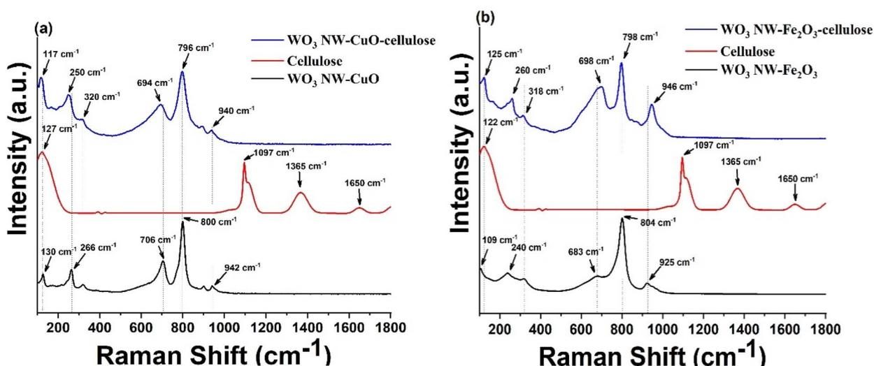
Fig. 3 Raman spectra of (a) WO<sub>3</sub> NW-CuO-cellulose, (b) WO<sub>3</sub> NW-Fe<sub>2</sub>O<sub>3</sub>-cellulose hybrid membranes.
