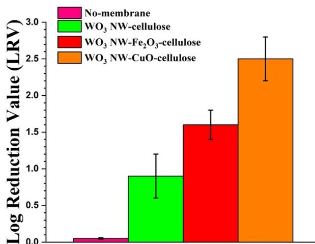
Fig. 7 MS2 retention values of WO<sub>3</sub> NW-based membranes in gravity driven filtration.
