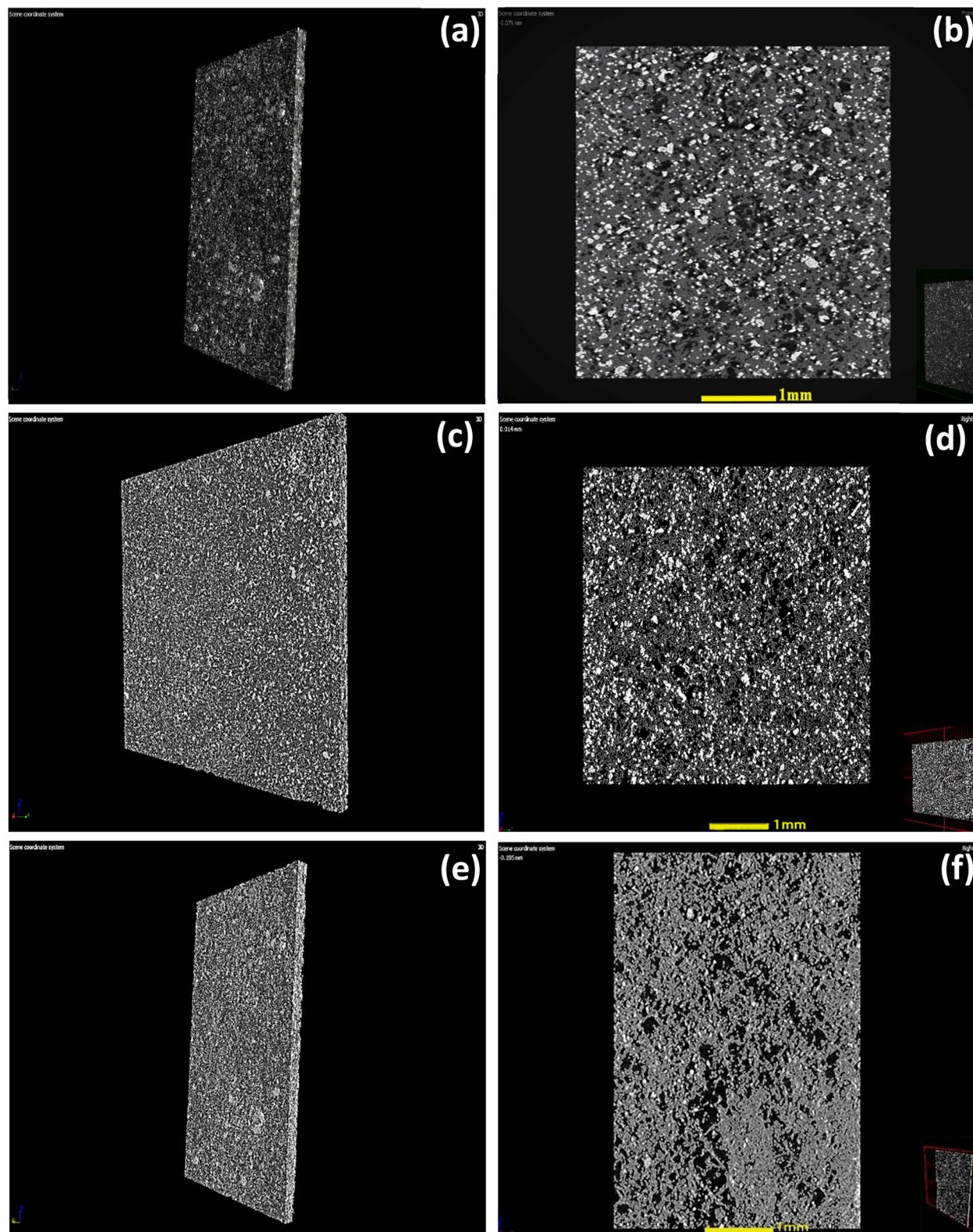
Fig. 1 Three-dimensional computed tomography (CT) cross-section analysis of hybrid membranes:  $\text{WO}_3$  NWs-cellulose (a and b),  $\text{WO}_3$  NW- $\text{Fe}_2\text{O}_3$ -cellulose (c and d) and  $\text{WO}_3$  NW-CuO-cellulose (e and f).
