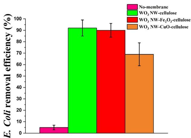
Fig. 6 Bacterial filtration efficiency (BFE%) of WO<sub>3</sub> NW-based hybrid membranes.
