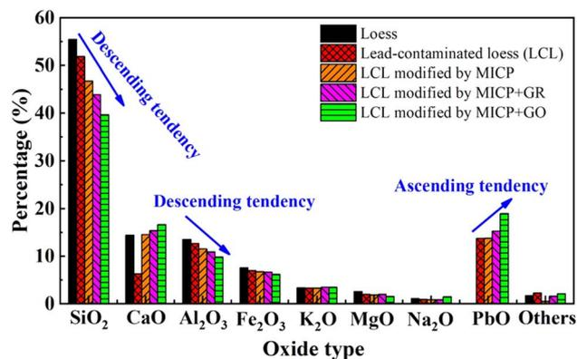
Fig. 13 Variation patterns of oxide composition under different remediation conditions.
