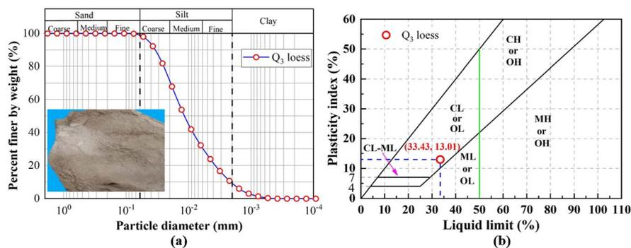
Fig. 2 (a) Particle size distribution of  $Q_3$  loess and (b) liquid limit and plastic index.
