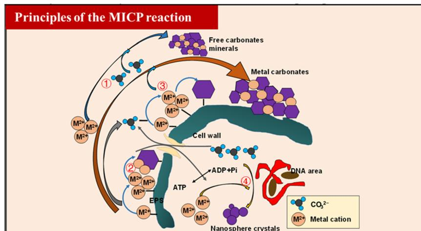
Fig. 3 The process of MICP (EPS: extracellular polymeric substances) (modified from He *et al.*<sup>6</sup>).
