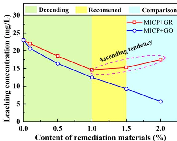
Fig. 11 Relationship between leaching concentration of lead and content of different remediation materials.
