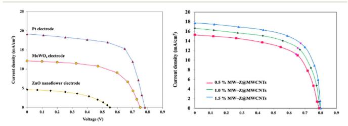
Fig. 7 Current-voltage characteristics of DSSCs with different counter electrodes. (Reproduced from ref. 80 with permission from Nature, copyright 2022.).
