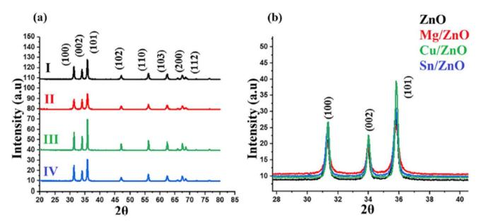
Fig. 2 (a) XRD patterns of (I) undoped ZnO (II) Mg/ZnO (III) Cu/ZnO (IV) Sn/ZnO. (b) High-resolution XRD patterns of undoped and doped ZnO NPs. (Reproduced from ref. 17 with permission from Springer, copyright 2024).
