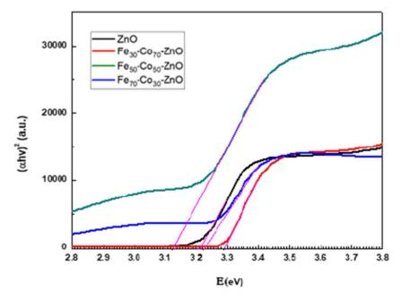
Fig. 3 Tauc plots for pure ZnO and dopped ZnO samples used to calculate the band gap. (Reproduced from ref. 19 with permission from MDPI, copyright 2022).
