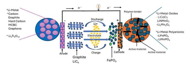
Fig. 8 Schematic diagram of basic components of an operational lithium-ion battery. (Reproduced from ref. 100 with permission from MDPI, copyright 2025).
