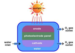
Fig. 6 Photoelectrochemical (PEC) water splitting. (Authors' work).
