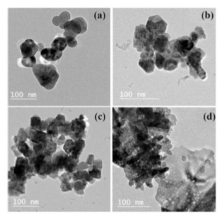
Fig. 1 TEM images of (a) undoped ZnO (b) Mg/ZnO (c) Cu/ZnO (d) Sn/ZnO. (Reproduced from ref. 18 with permission from Springer Nature, copyright 2023).
