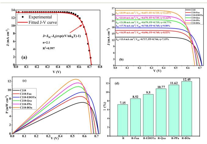
Fig. 18 Experimental and fitted J-V curves for the reference dye (a), simulated electron transfer results (b), simulated J-V and P-V curves (c), and estimated PCE (d) for the studied dyes.
