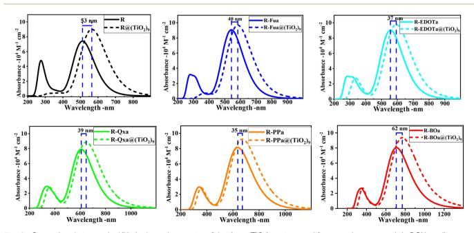
Fig. 10 Comparison between the UV-vis absorption spectra of the dyes@(TiO<sub>2</sub>)<sub>9</sub> systems and free organic compounds in DCM medium.
