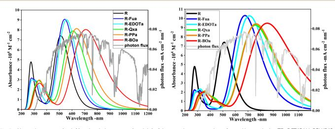
Fig. 5 Absorption spectra (on left) and emission spectra (on right) of the organic compounds performed by employing TD-DFT/CAM-B3LYP/6-311G\*\* under CPCM in DCM medium.
