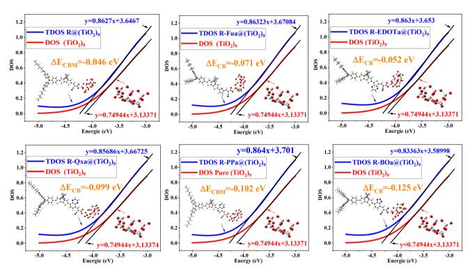
Fig. 17 DOS of  $(TiO_2)_9$  cluster and PDOS of the free organic compounds with linear fits and  $\Delta E_{CB}$ .
