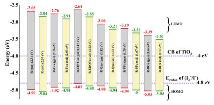
Fig. 4 The schematic energy diagram of each organic compound in DCM medium and vacuum level.
