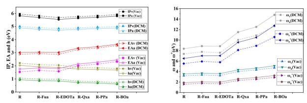
Fig. 11 Plot of adiabatic (a) and vertical (v) chemical reactive parameters of the investigated dyes in vacuum level (Vac) and DCM medium calculated by employing DFT/B3LYP/6-311G\*\*.
