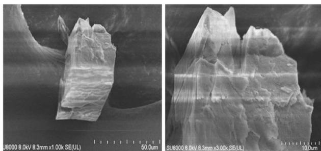
Fig. 3 SEM images of FCCF at different magnifications.
