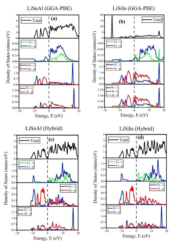
Fig. 3 The Total Density of States (TDOS) and partial density of states (PDOS) of LiSnAl and LiSiln compounds *via* GGA-PBE and Hybrid-HSE06 functionals [(a) LiSnAl with GGA-PBE, (b) LiSiln with GGA-PBE, (c) LiSnAl with Hybrid-HSE06 (d) LiSiln with Hybrid-HSE06].
