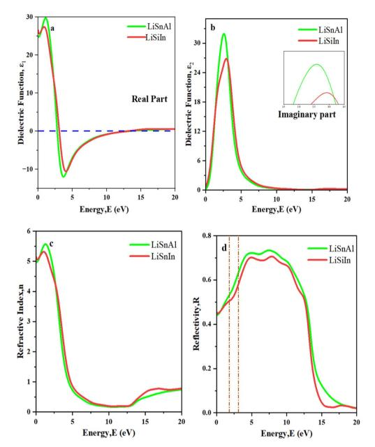
Fig. 6 Photon energy dependence of (a) real  $\varepsilon_1$ , (b) imaginary part of dielectric function  $\varepsilon_2$ , (c) refractive index n, (d) reflectivity R of LiSnAl and LiSiIn.
