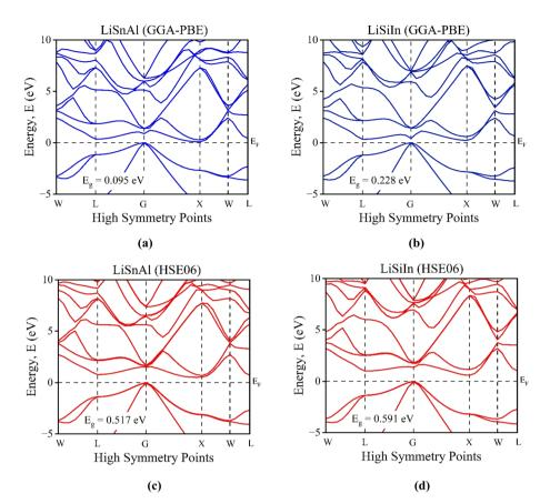
Fig. 2 The calculated electronic band structure (EBS) of the half-Heusler compounds with GGA-PBE and Hybrid-HSE06 functionals [(a) LiSnAl with GGA-PBE, (b) LiSiln with GGA-PBE, (c) LiSnAl with Hybrid-HSE06 (d) LiSiln with Hybrid-HSE06].
