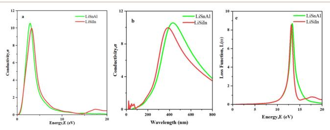
Fig. 8 Optical properties (a) and (b) conductivity and (c) loss function of LiSnAl and LiSiln at the polarization vector [100].
