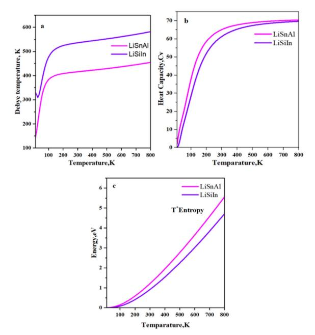
Fig. 10 The calculated thermodynamic properties (a) Debye temperature, (b) heat capacity (C<sub>v</sub>), and (c) entropy with respect to internal energy.
