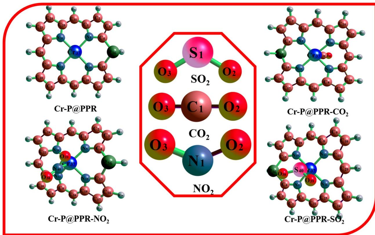
Fig. 1 Optimized structures of CO<sub>2</sub>, SO<sub>2</sub>, and NO<sub>2</sub> adsorption on the Cr-P@PPR surface, showing the configurations before and after adsorption for each gas molecule.
