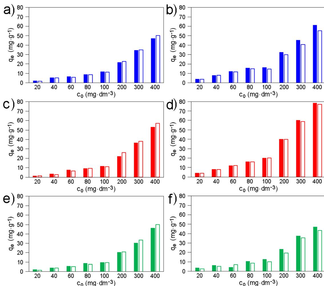
Fig. 10 Comparison of  $q_e$  values from the first (filled bars) and the second (empty bars) adsorption experiment for (a) MMT/AMP, (b) MMT/LAM, (c) BEI/AMP, (d) BEI/LAM, (e) NON/AMP, and (f) NON/LAM in dependence on  $c_0$  values. The numerical values of  $q_e$ ,  $c_0$ , and  $c_e$  are provided in Table S19.
