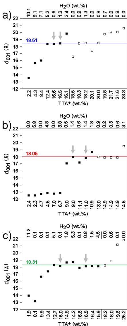
Fig. 2 The content of TTA<sup>+</sup> (wt%) and H<sub>2</sub>O (wt%) in the optimized models, and corresponding  $d_{001}$  values obtained by simulated diffraction (squares) compared to experimentally determined  $d_{001}$  values (horizontal lines) are shown for MMT-M (a), BEI-M (b), and NON-M (c). Models agreeing with the experimental results of elemental analysis are represented by solid squares. Models corresponding to real samples are indicated by grey arrows.
