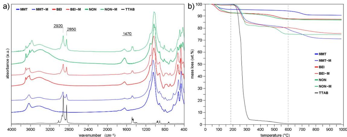
Fig. 1 (a) FTIR spectra and (b) TGA curves of original smectites, modified smectites and TTAB.
