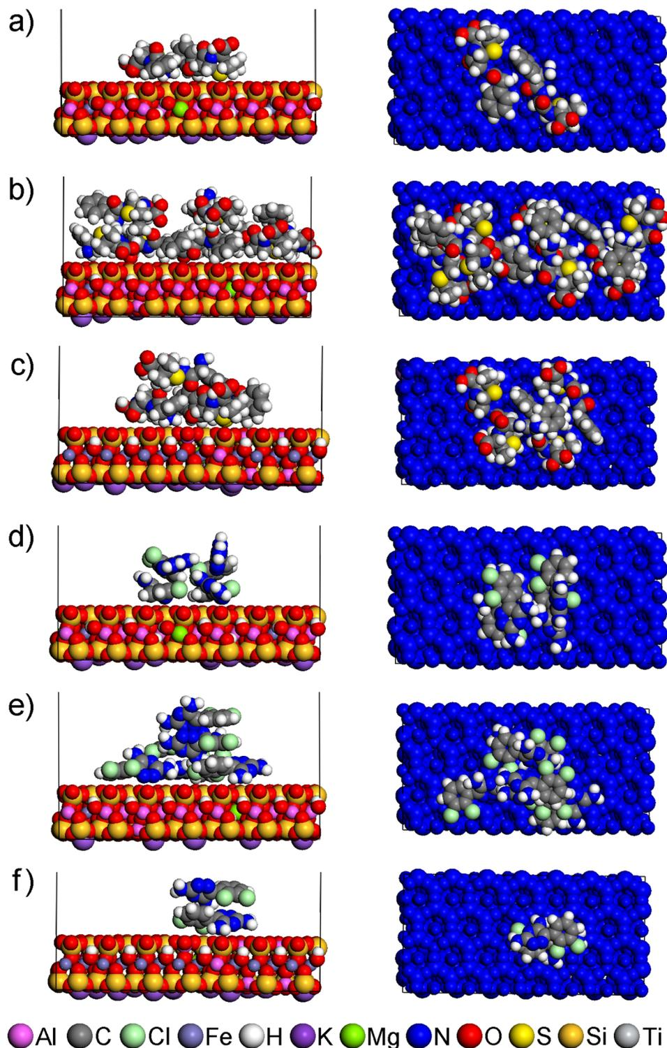
Fig. 9 Side views (left) and top views (right) of the models of the surfaces of original smectites with more drug molecules (*i.e.* 2, 7, 4 AMPs and 3, 6, 2 LAMs for MMT, BEI, NON, respectively): (a) MMT/AMP, (b) BEI/AMP, (c) NON/AMP, (d) MMT/LAM, (e) BEI/LAM, (f) NON/LAM. For clarity, each smectite is colored blue in the top views. Composition of the displayed models together with  $E_{\text{int}}$  values is available in Table S18.
